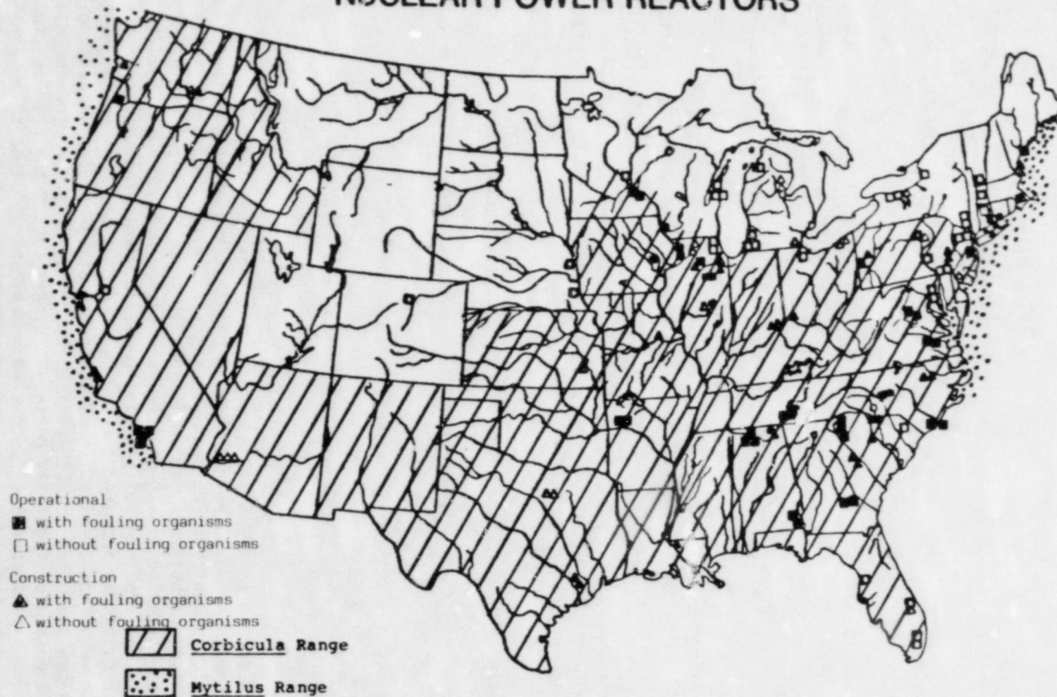
Figure A-1. Corbicula and Mytilus ranges and their relationship to nuclear power reactors in the United States 1983. Only facilities actively operating or under construction are shown.
