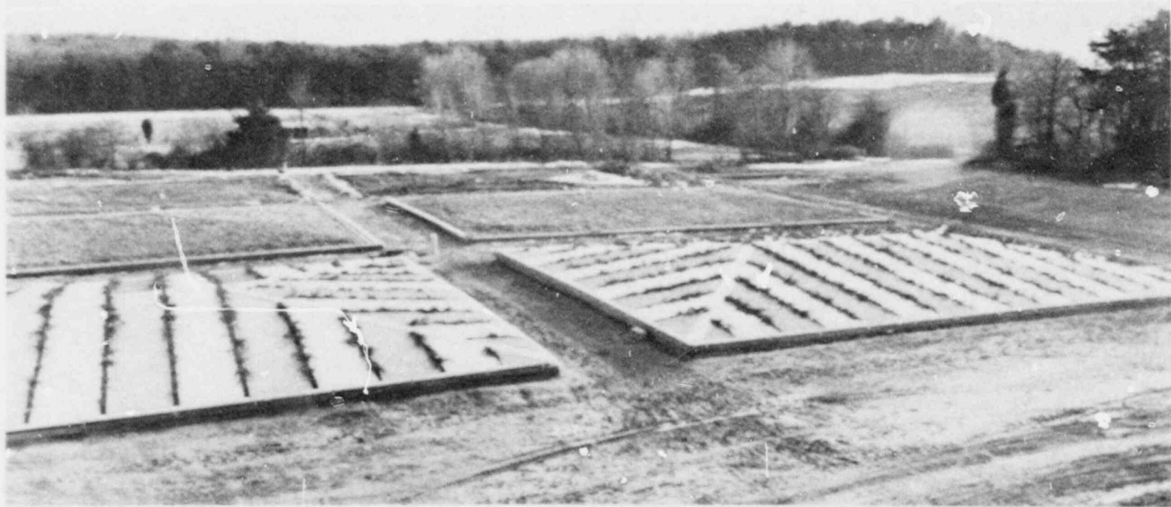
FIGURE 9. Large-scale bioengineering management lysimeters. Each cell (lysimeter or plot) is 14 m x 21 m with Pfitzer Juniper growing through the 4-inch gaps between panels. The light appearing panels are corrugated aluminum and the darker panels are corrugated green fiberglass panels. Two crowned lysimeters behind the bioengineered lysimeters are cropped to fescue grass for comparative purposes. Two lysimeters at the rear are reserved for future work.
