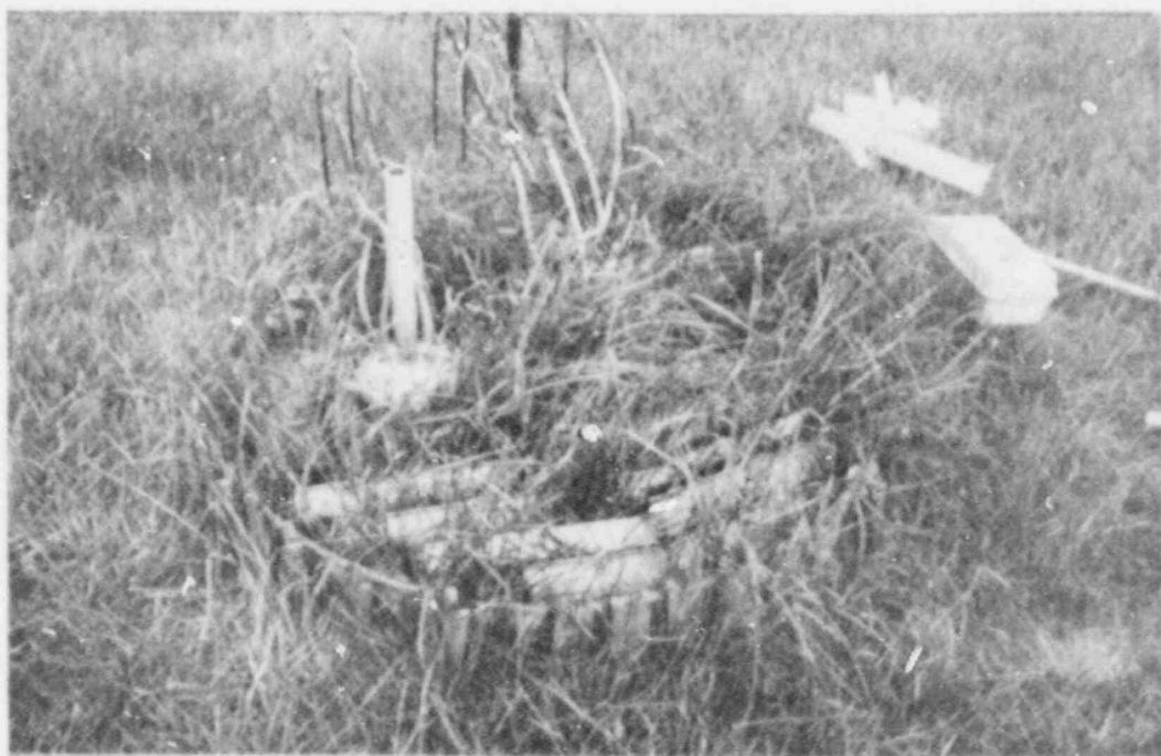
FIGURE 6. Lysimeter with Kentucky fescue grass one year after addition of enhanced run-off system. Grass has grown up between gutters and provides substantial evapotranspiration. 1985.
