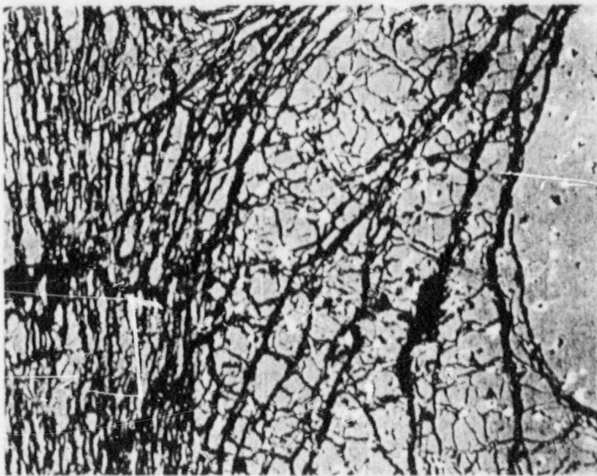
Figure 7. Photograph of prior molten debris from lower flow blockage region of the SFD 1-1 fuel bundle illustrating extensive cracking.
