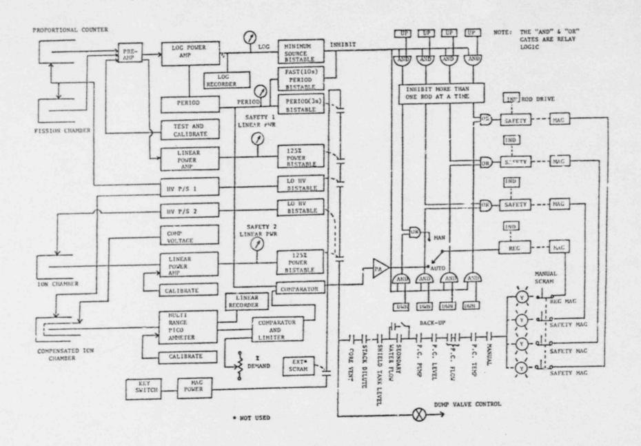
Figure 7-1, Overall UFTR Instrumentation and Scram Logic Diagram.
