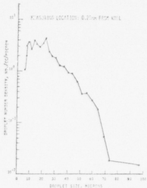
FIGURE 2. DROPLET SIZE AND NUMBER DENSITY DISTRIBUTIONS WITH LIQUID FILM ON WALL
