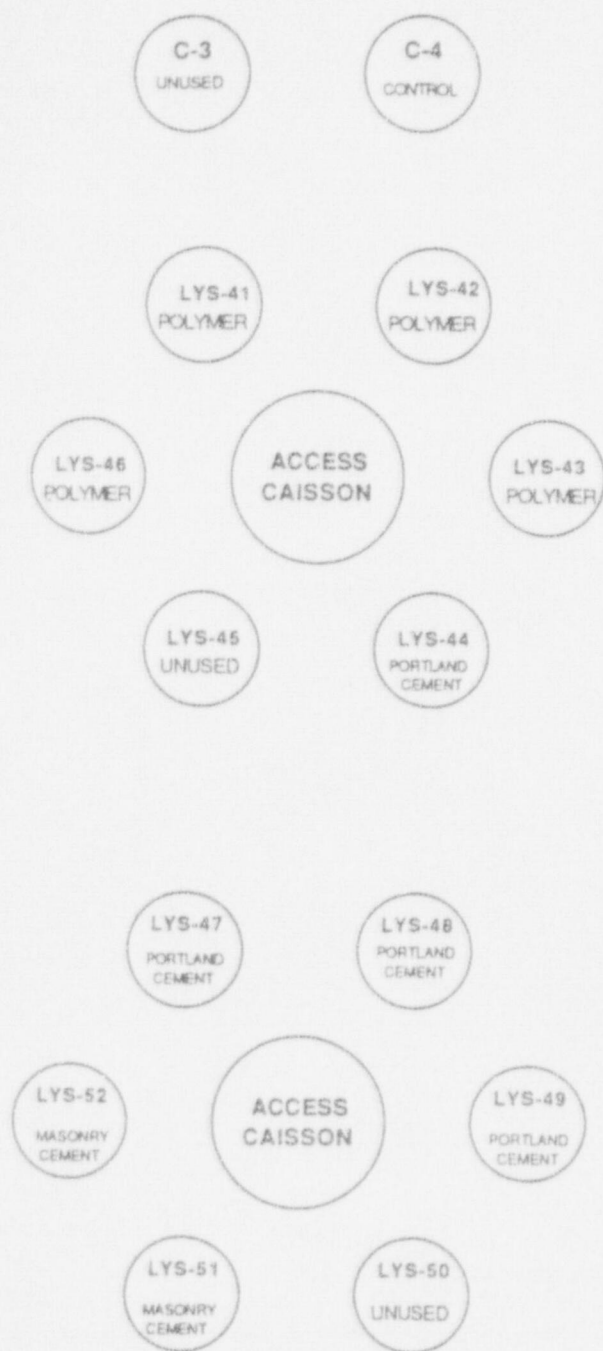
Figure 6. Arrangement of special waste form lysimeters in the SRS burial ground (McIntyre and Hawkins 1987).
