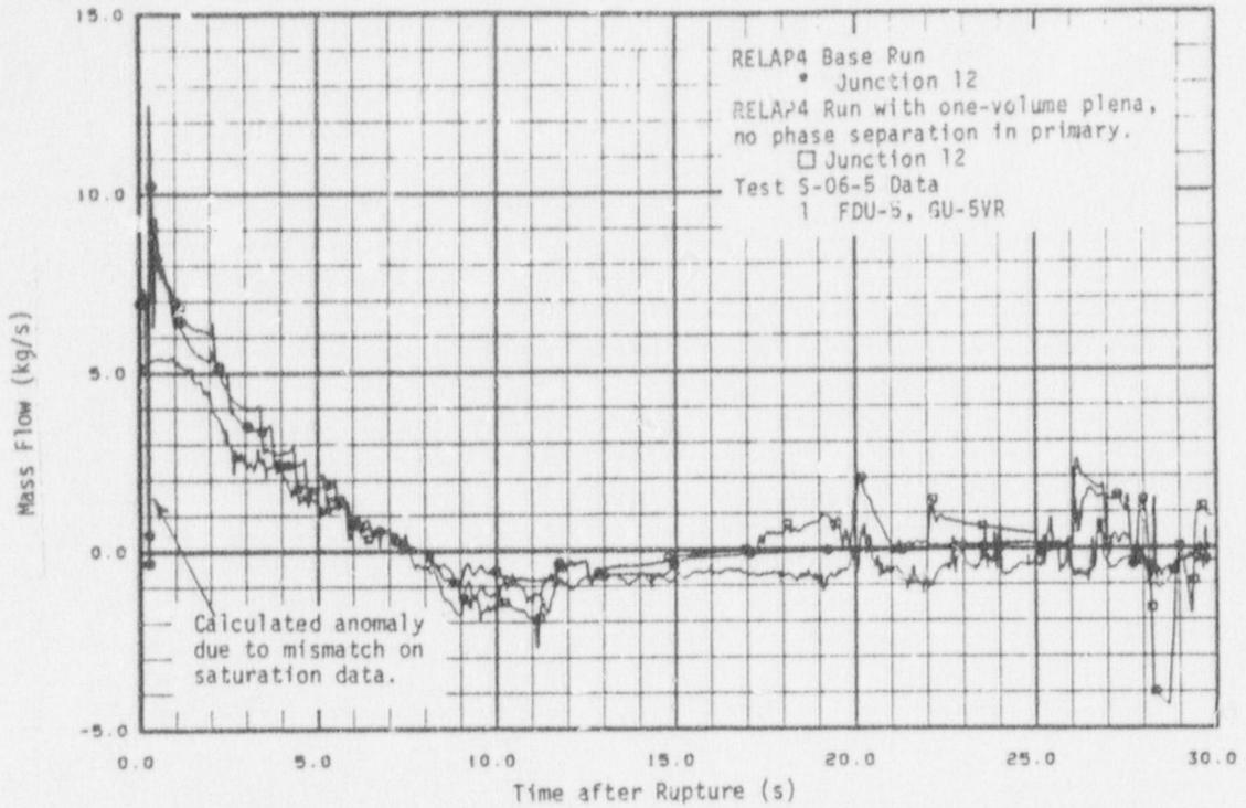
Fig. 35 Mass flow on pressurizer side - Test S-06-5 with one-volume plena, no phase separation in primary.
