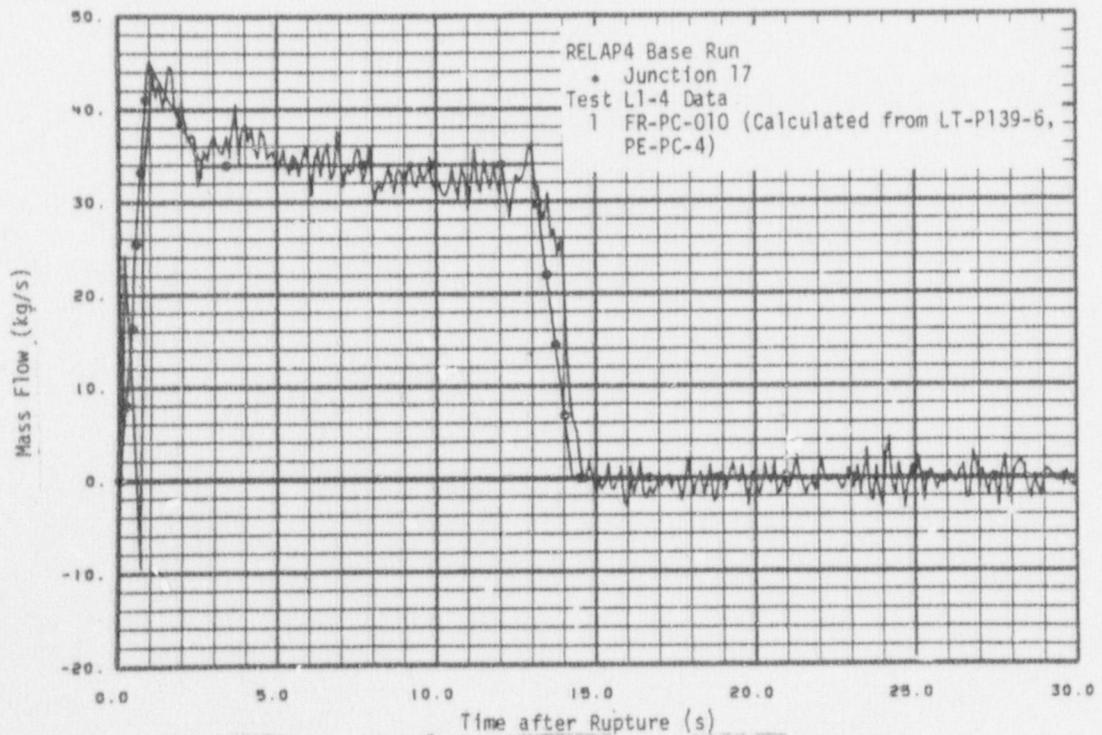
Fig. 20 Pressurizer mass flow - Test L1-4 boundary conditions.
