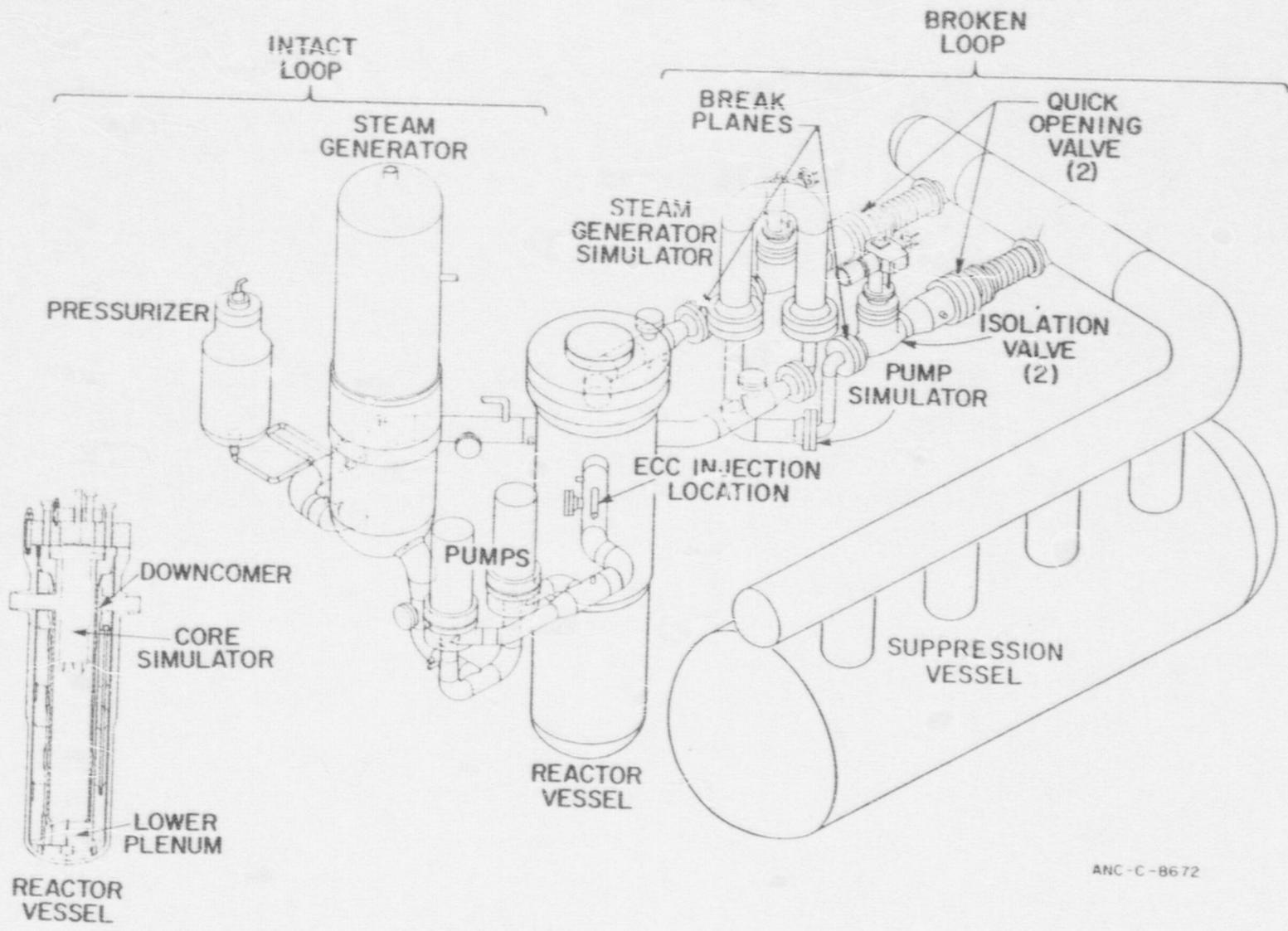
Fig. 3 LOFT system for cold leg break configuration - isometric.
