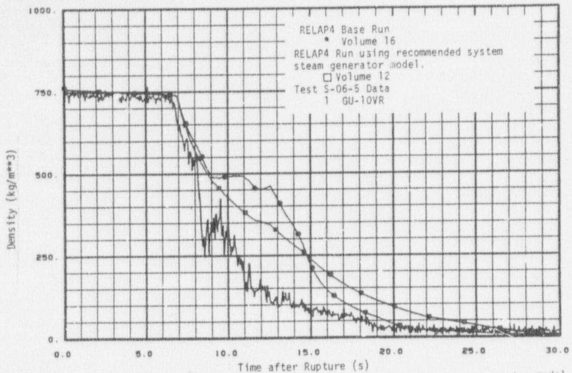
Fig. 47 Density on pump side - Test S-06-5 recommended system steam generator model.
