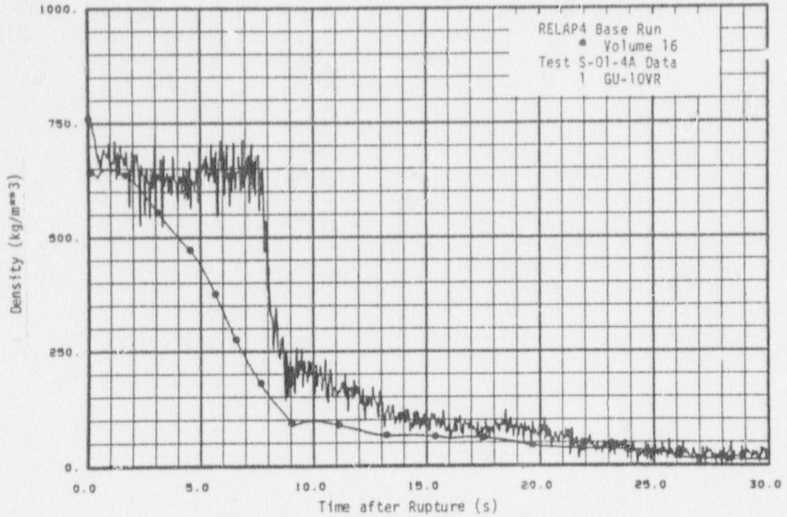
Fig. 25 Density on pump side - Test S-01-4A base run.
