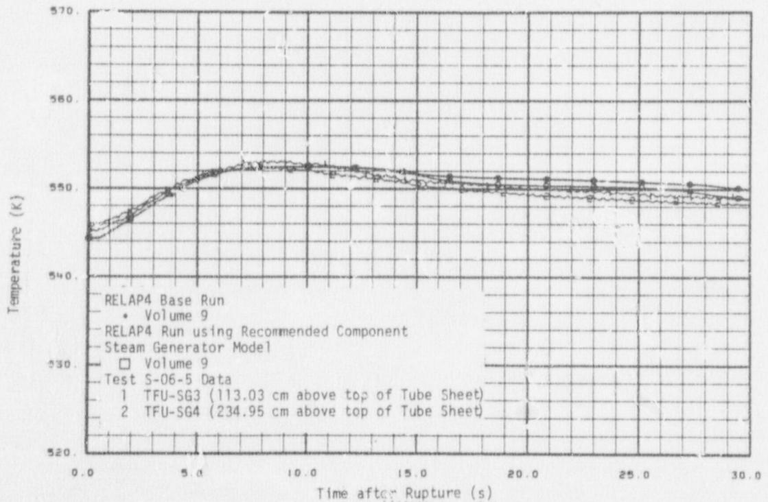
Fig. 46 Fluid temperature in steam generator secondary - Test S-06-5 recommended component steam generator model.
