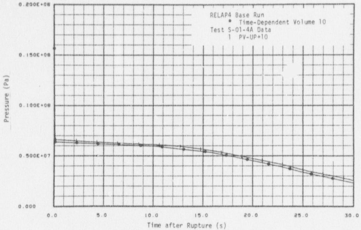
Fig. 15 Pressure on pressurizer side - Test S-01-4A boundary conditions.
