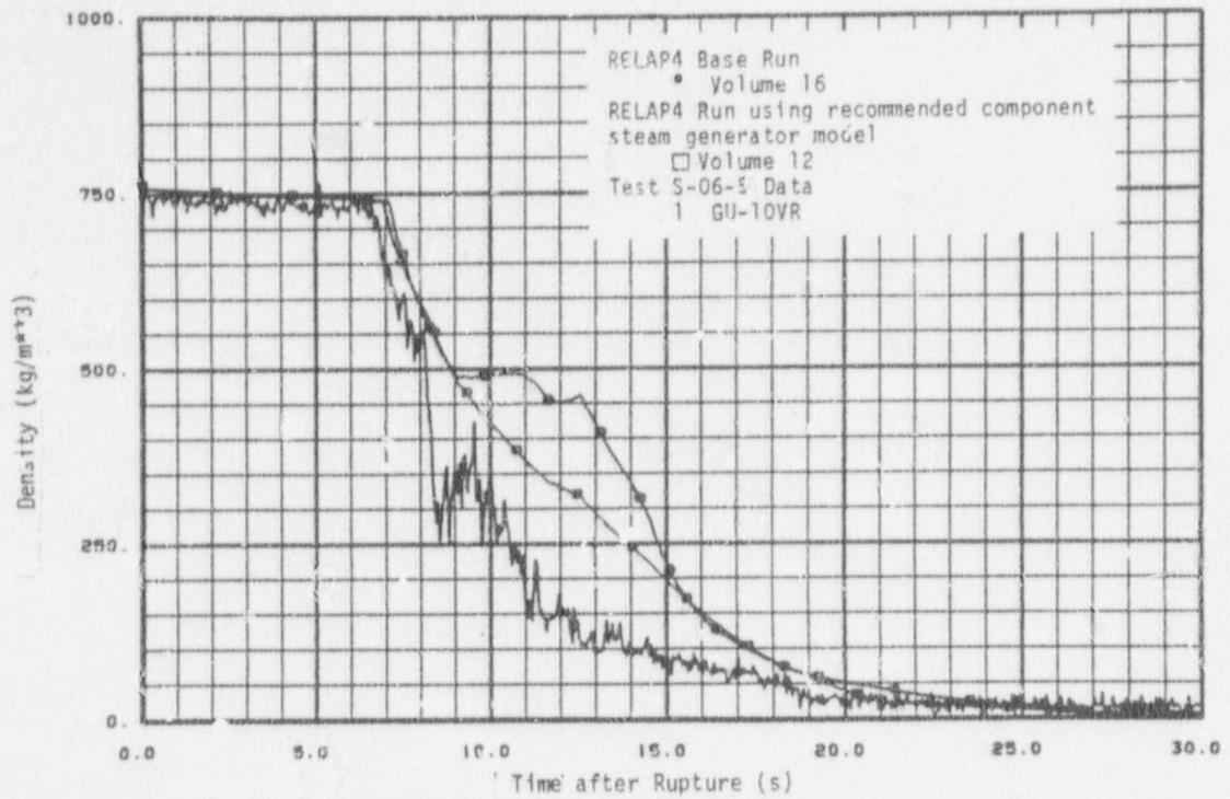
Fig. 45 Density on pump side - Test S-06-5 recommended component steam generator model.
