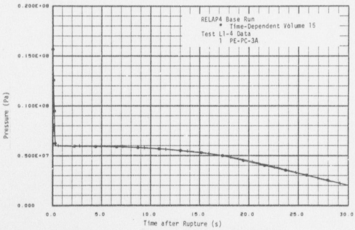
Fig. 18 Pressure on pump side - Test L1-4 boundary conditions.
