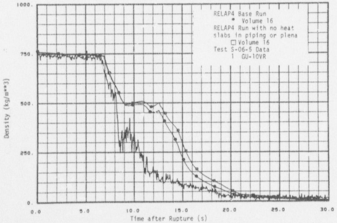
Fig. 30 Density on pump side - Test S-06-5 with no heat slabs in piping or plena.
