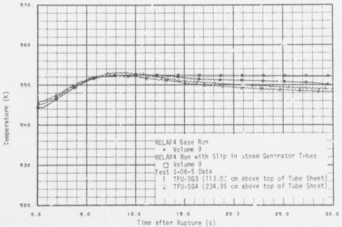
Fig. 38 Fluid temperature in steam generator secondary - Test S-06-5 with slip in steam generator tubes.
