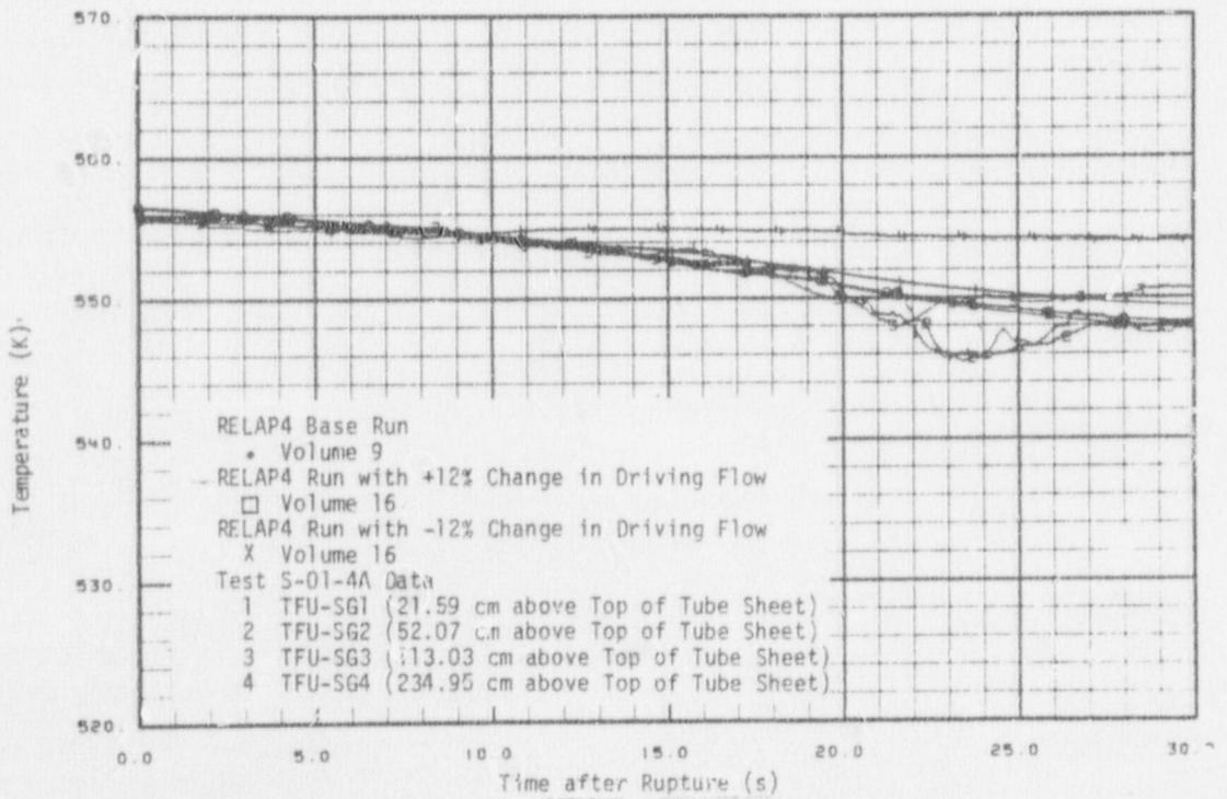
Fig. 50 Fluid temperature in steam generator secondary - Test S-01-4A with  $\pm 12\%$  change in driving flow.
