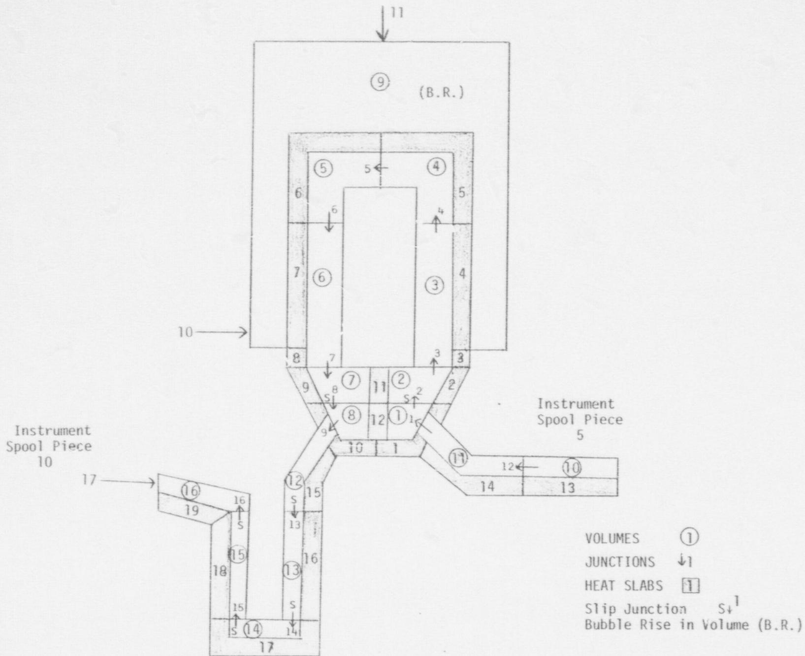
Fig. 7 Base run model of Semiscale steam generator.
