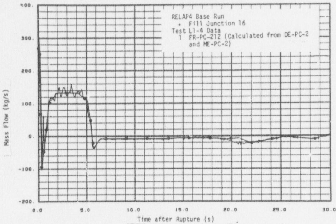
Fig. 17 Mass flow on core side - Test L1-4 boundary conditions.
