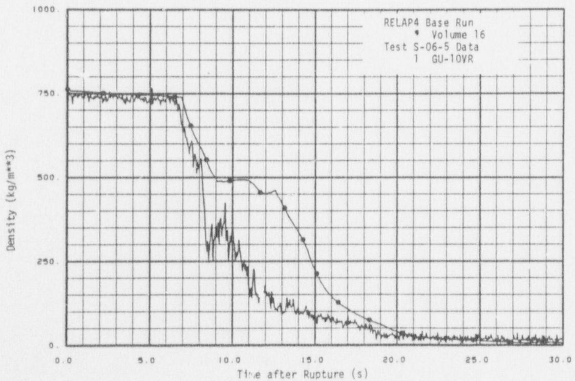
Fig. 22 Density on pump side - Test S-06-5 base run.
