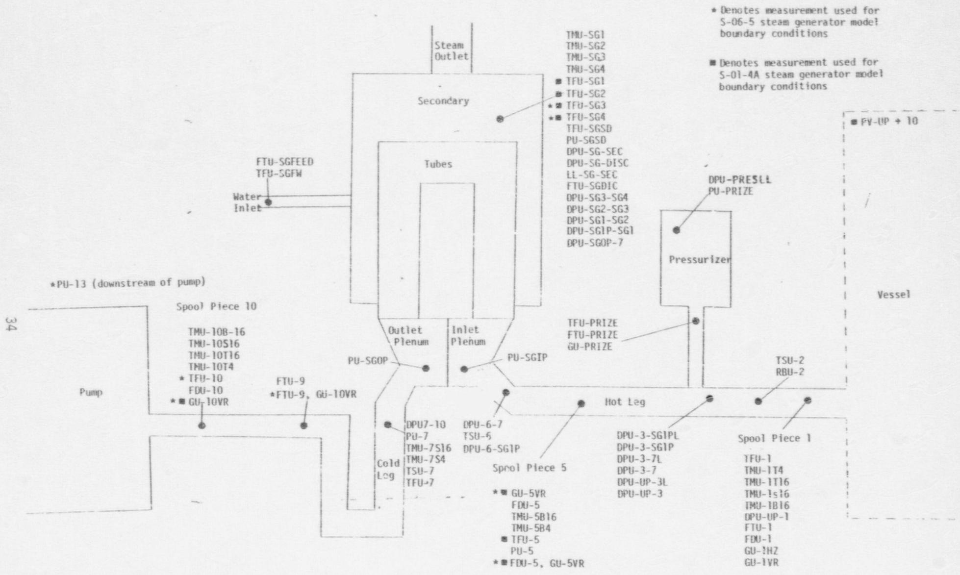
Fig. 2 Semiscale intact loop instrumentation between vessel and pump.
