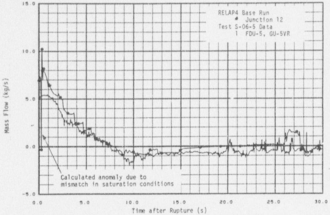
Fig. 21 Mass flow on pressurizer side - Test S-06-5 base run.
