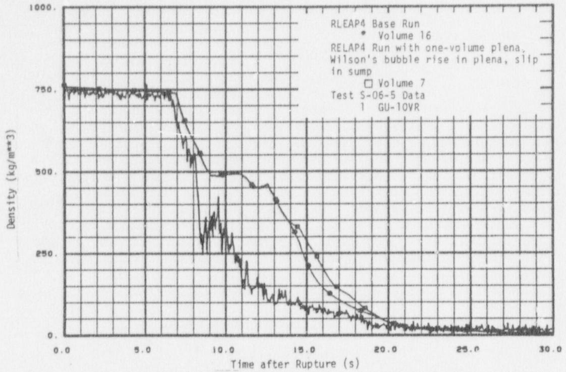
Fig. 33 Density on pump side - Test S-06-5 with one-volume plena, Wilson's bubble rise in plena, slip in sump.
