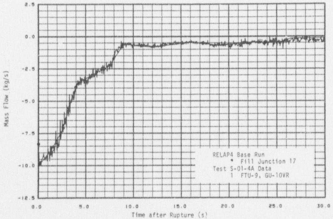
Fig. 14 Mass flow on pump side - Test S-01-4A boundary conditions.
