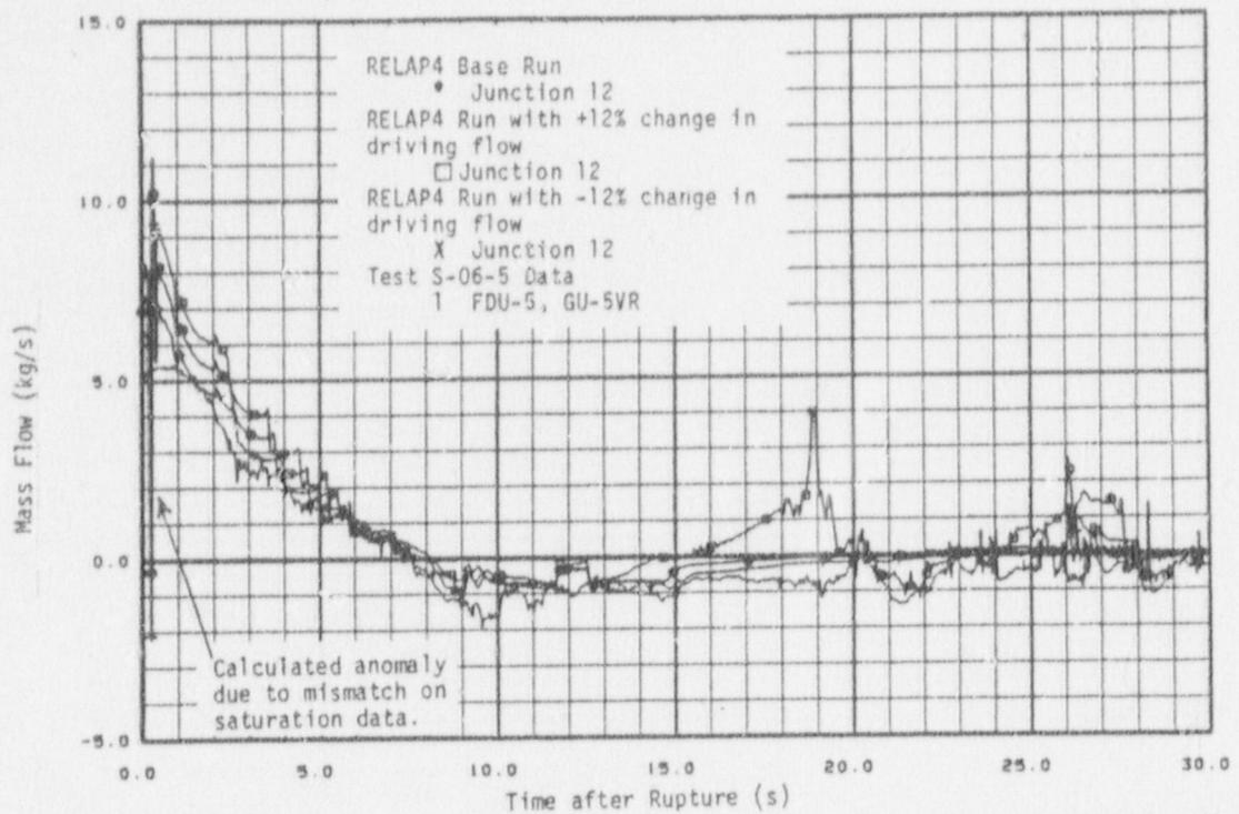
Fig. 39 Mass flow on pressurizer side - Test S-06-5 with  $\pm 12\%$  change in driving flow.
