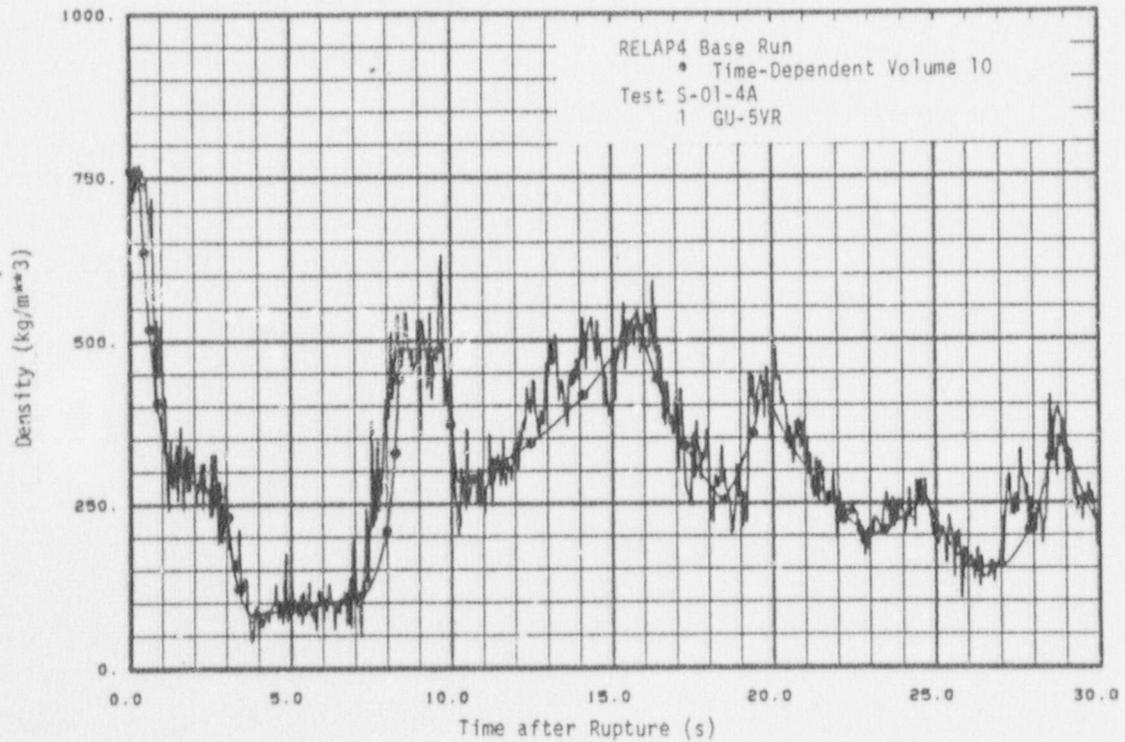
Fig. 16 Density on pressurizer side - Test S-01-4A boundary conditions.
