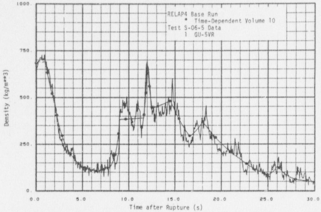
Fig. 11 Density on pressurizer side - Test S-06-5 boundary conditions.
