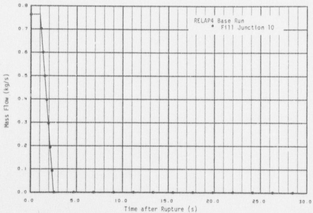
Fig. 12 Calculated mass flow at steam generator secondary inlet - Test S-06-5 boundary conditions.
