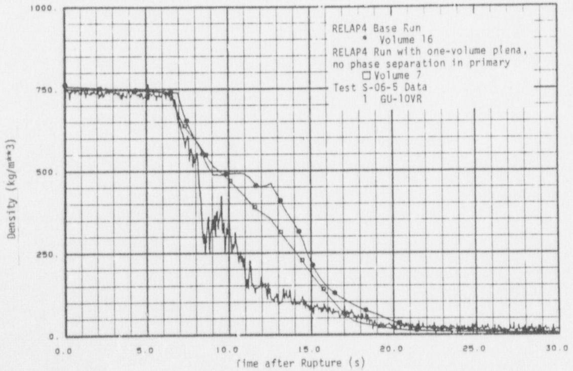
Fig. 36 Density on pump side - Test S-06-5 with one-volume plena, no phase separation in primary.
