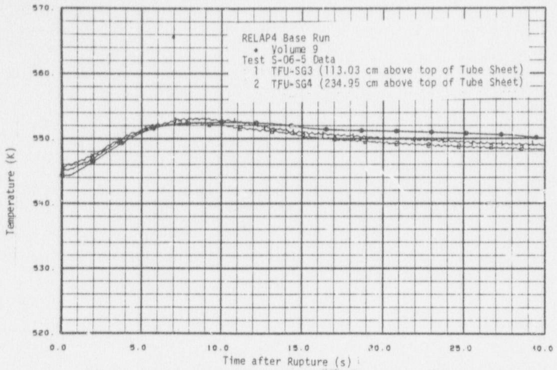
Fig. 23 Fluid temperature in steam generator secondary - Test S-06-5 base run.
