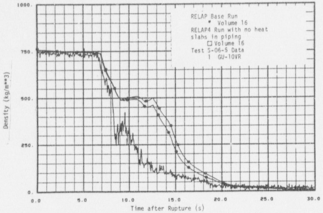
Fig. 29 Density on pump side - Test S-06-5 with no heat slabs in piping.
