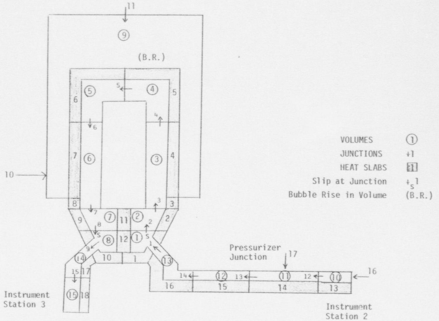
Fig. 8 Base run model of LOFT steam generator.
