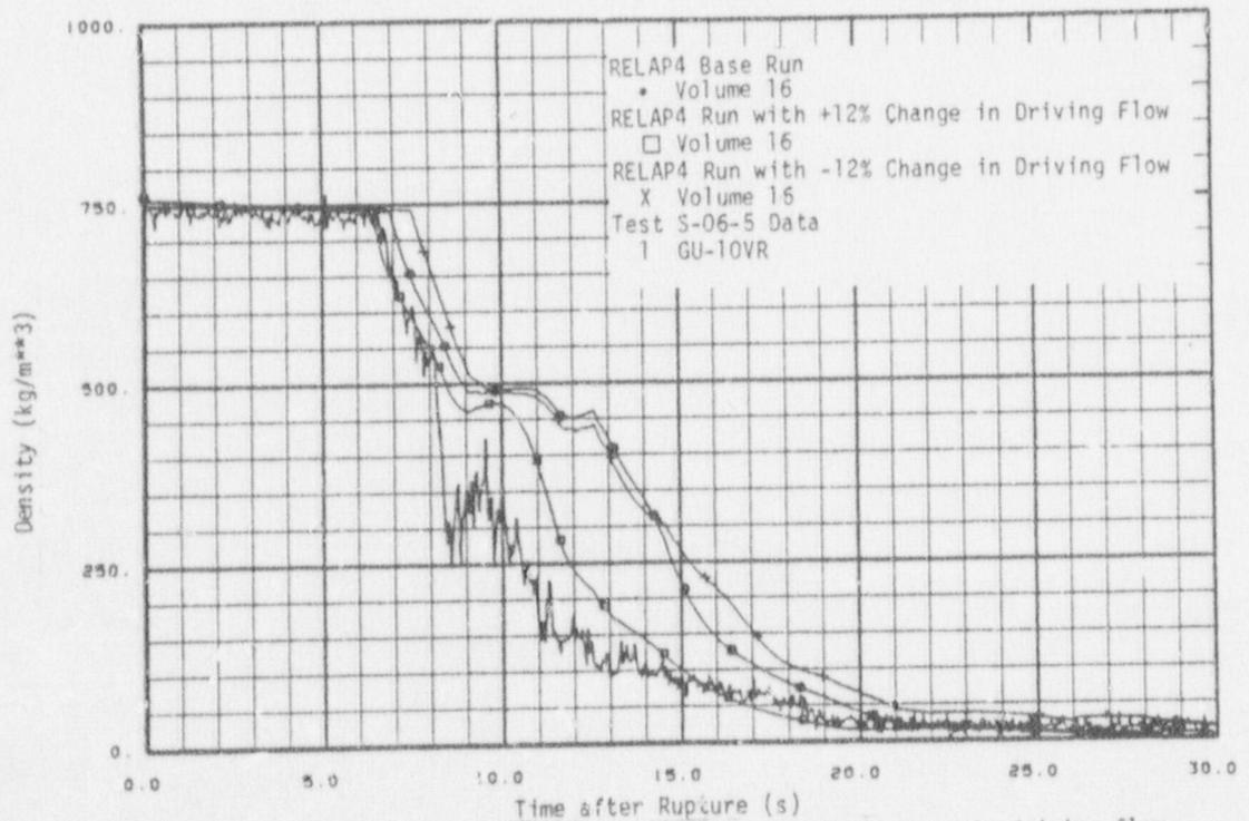
Fig. 40 Density on pump side - Test S-06-5 with  $\pm 12\%$  change in driving flow.
