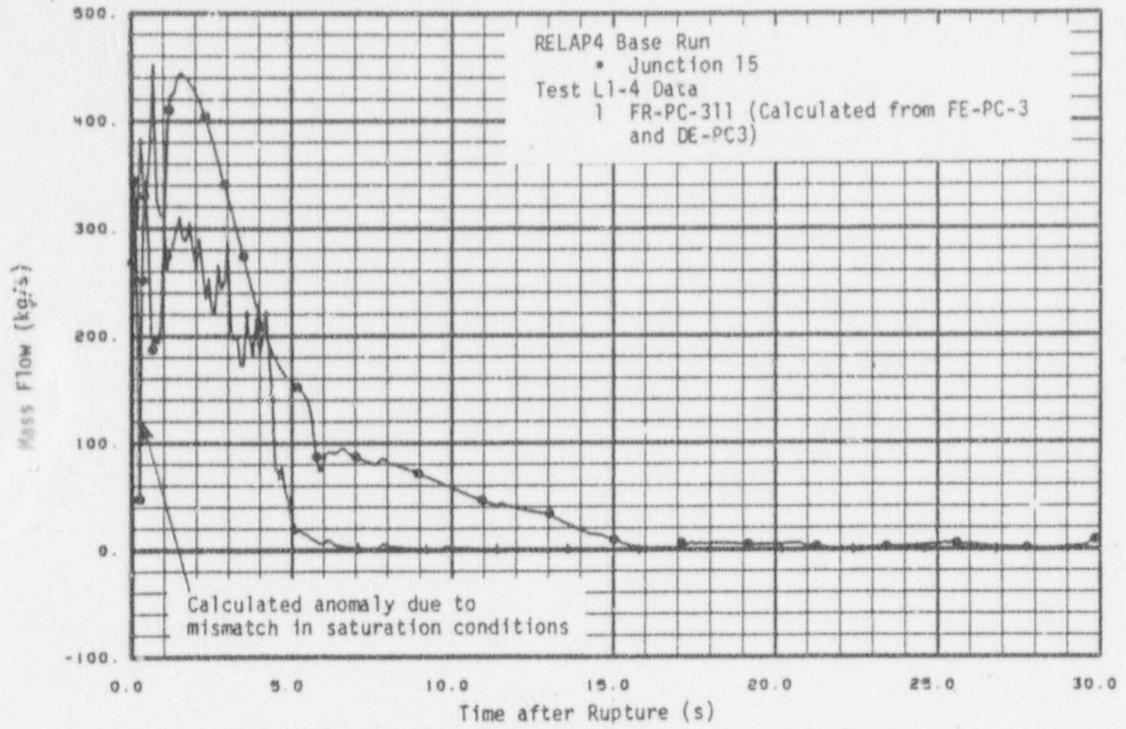
Fig. 27 Mass flow on pump side - Test L1-4 base run.
