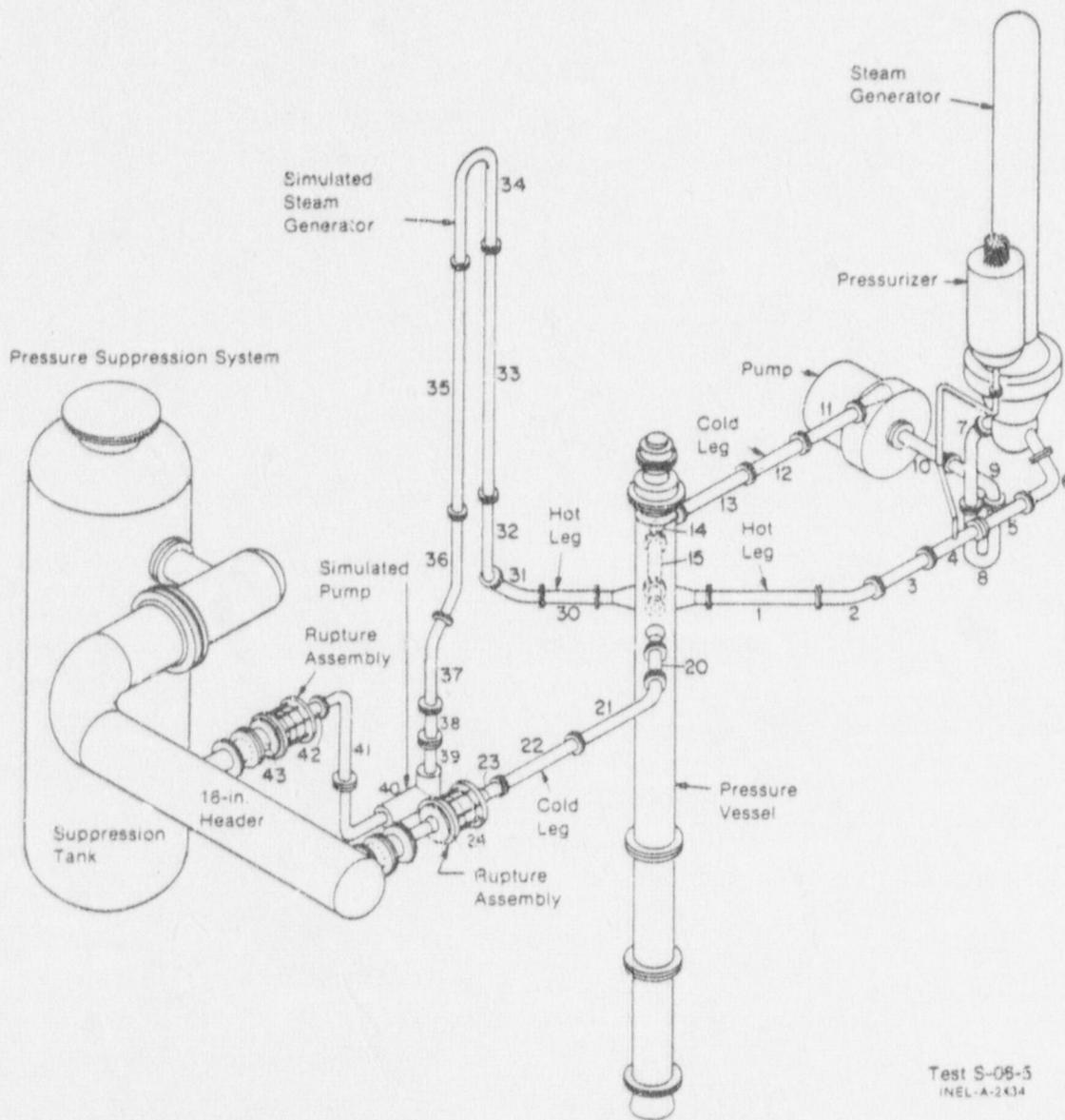
Fig. 1 Semiscale Mod-1 system for cold leg break configuration - isometric.
