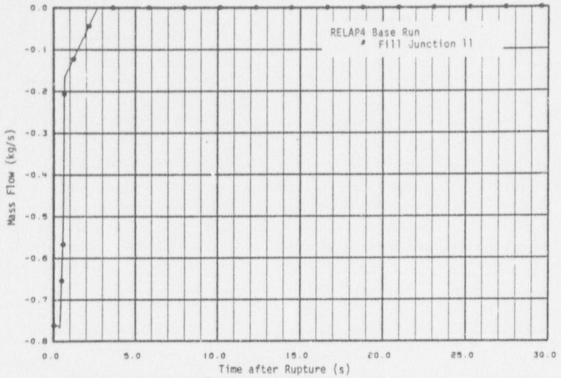
Fig. 13 Calculated mass flow at steam generator secondary outlet - Test S-06-5 boundary conditions.
