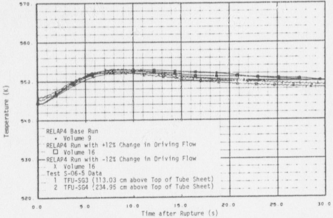
Fig. 41 Fluid temperature in steam generator secondary - Test S-06-5 with  $\pm 12\%$  change in driving flow.
