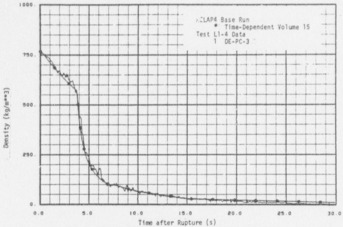
Fig. 19 Density on pump side - Test L1-4 boundary conditions.
