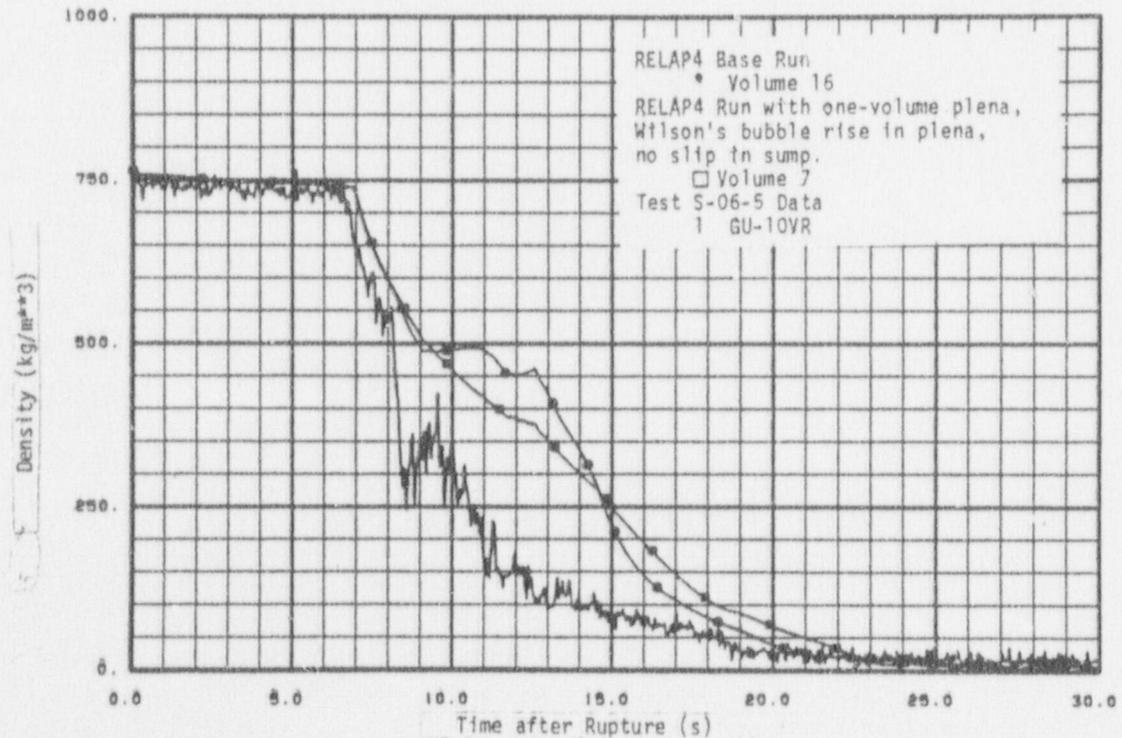
Fig. 34 Density on pump side - Test S-06-5 with one-volume plena, Wilson's bubble rise in plena, no slip in sump.
