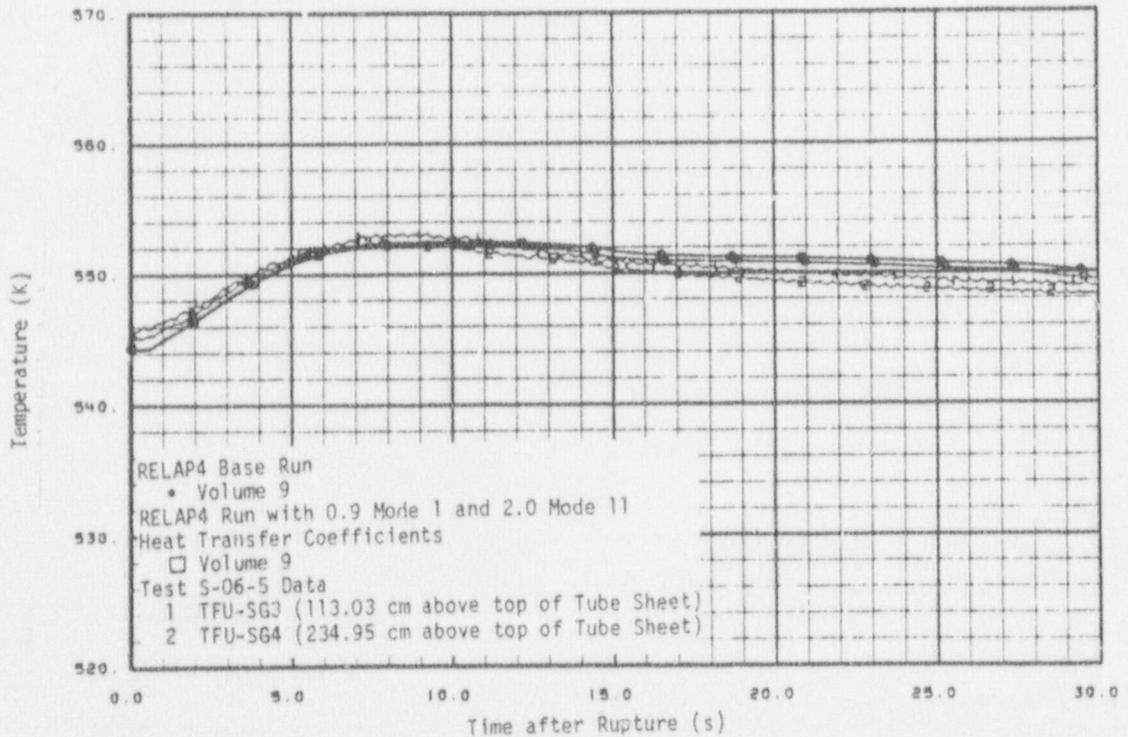
Fig. 42 Fluid temperature in steam generator secondary - Test S-06-5 with  $0.9 \times$  Mode 1 and  $2.0 \times$  Mode 11 heat transfer coefficients.
