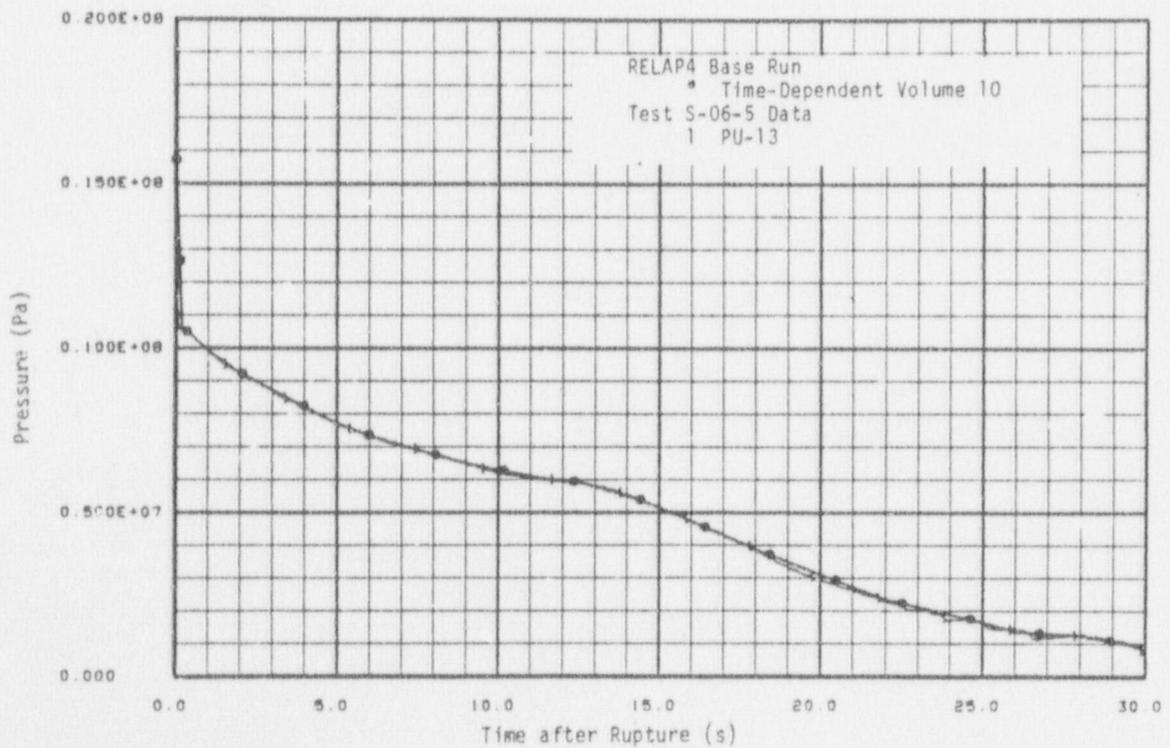
Fig. 10 Pressure on pressurizer side - Test S-06-5 boundary conditions.
