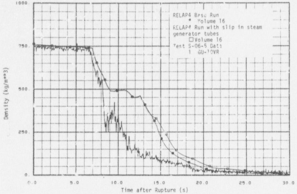
Fig. 37 Density on pump side - Test S-06-5 with slip in steam generator tubes.
