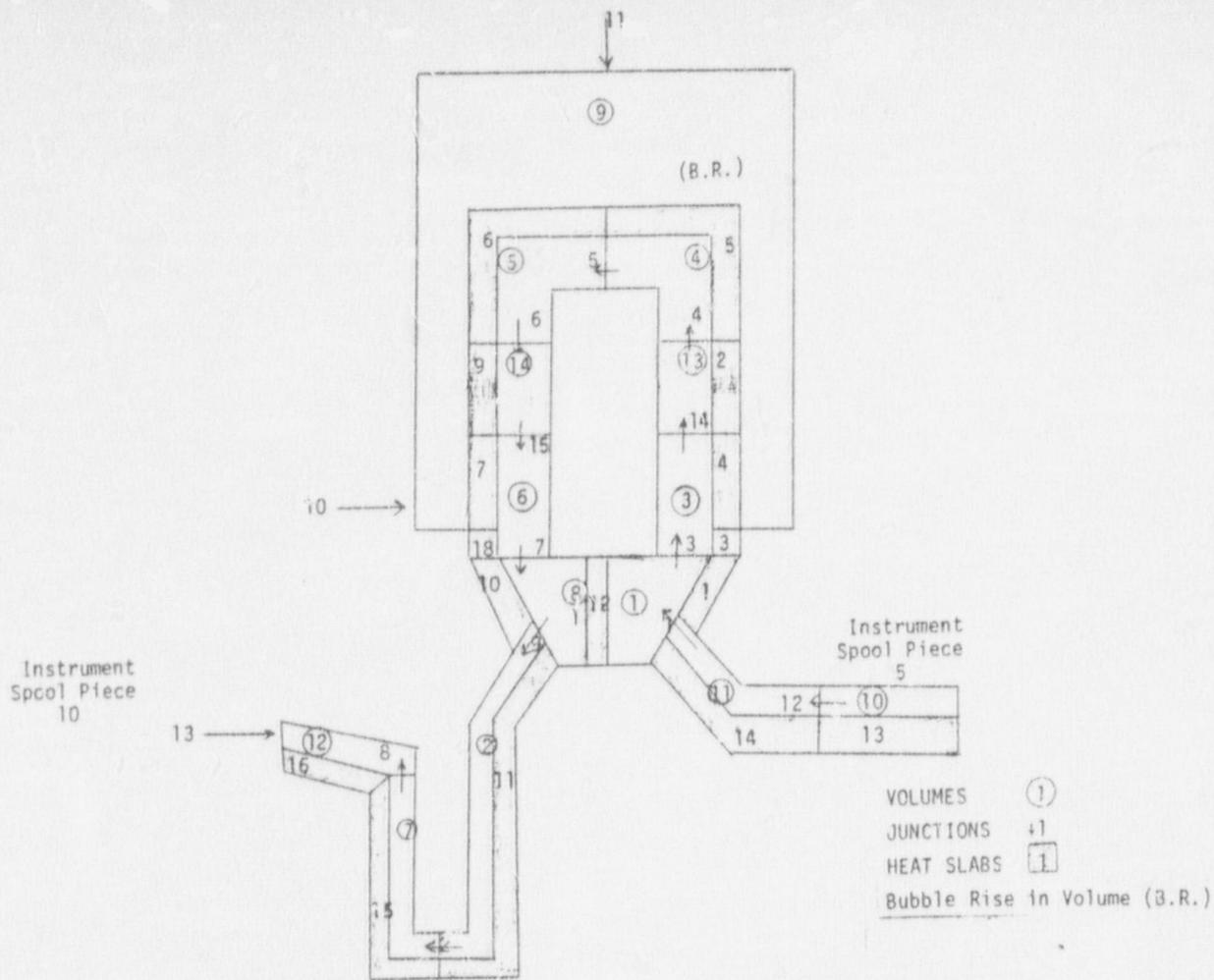
Fig. 43 Recommended component model of Semiscale steam generator for a heated blowdown.
