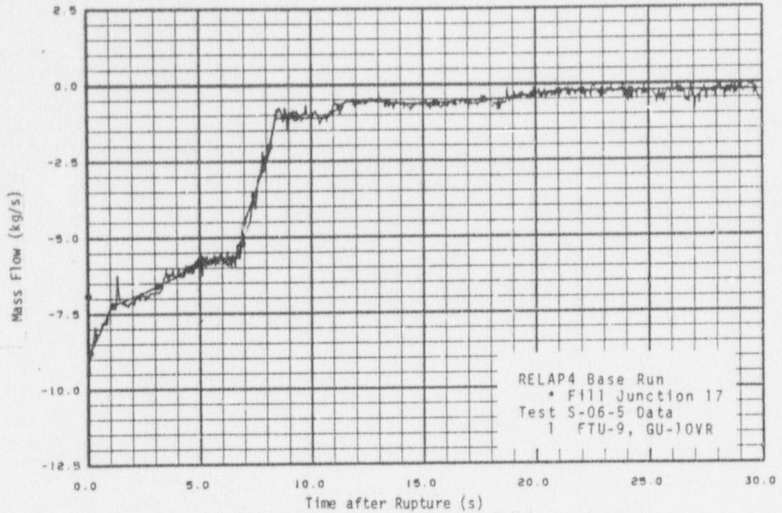
Fig. 9 Mass flow on pump side - Test S-06-5 boundary conditions.
