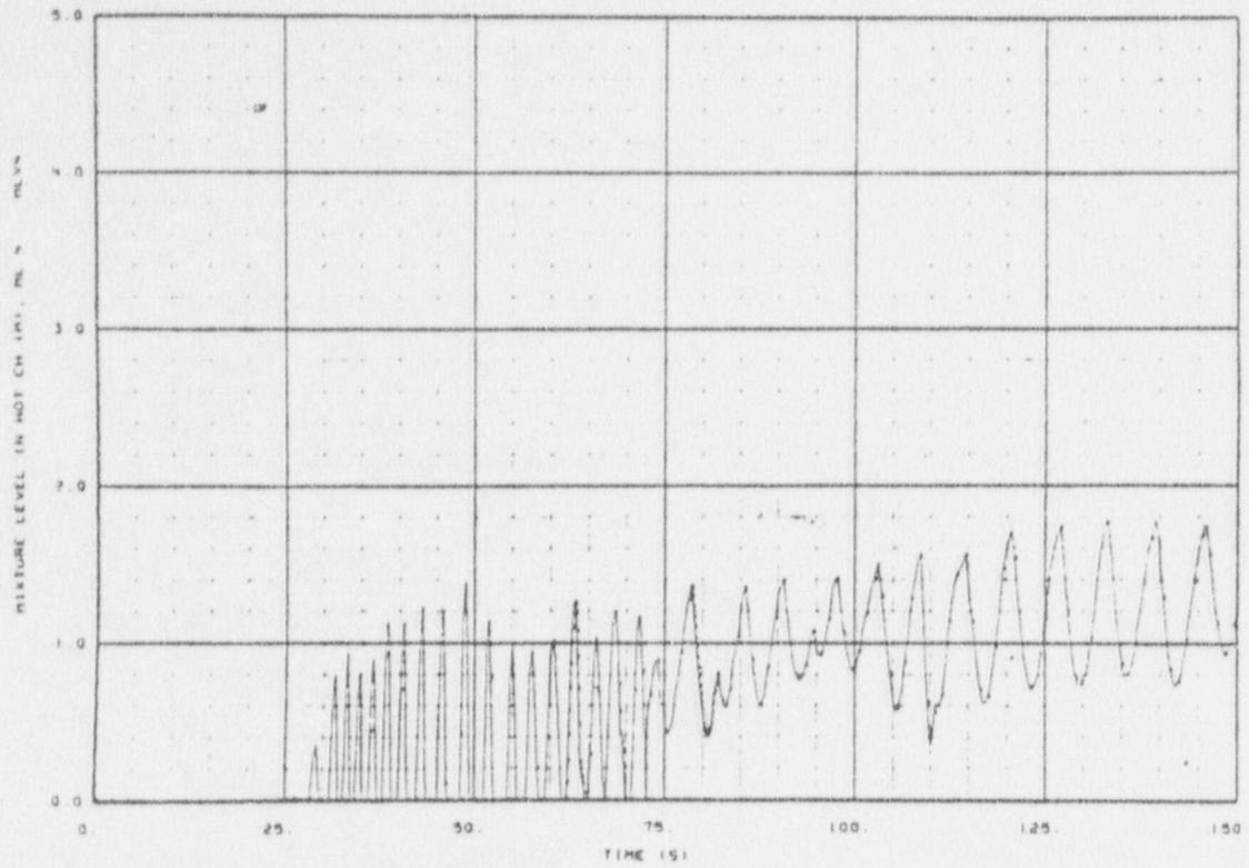
Fig. 64 Core hot-channel mixture-level history when undivided steam-generator inlet-side primary volumes were used.
