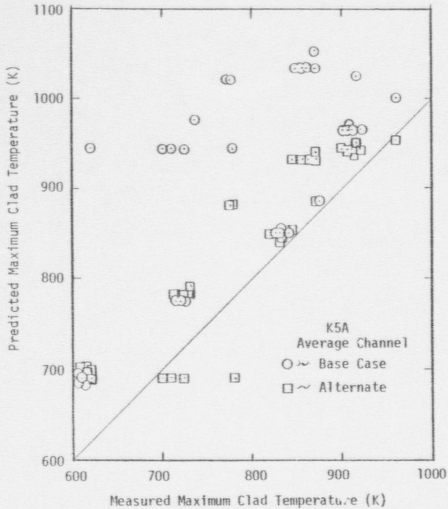
Fig. 17 Predicted vs. measured rod surface temperature, K5A average channel.
