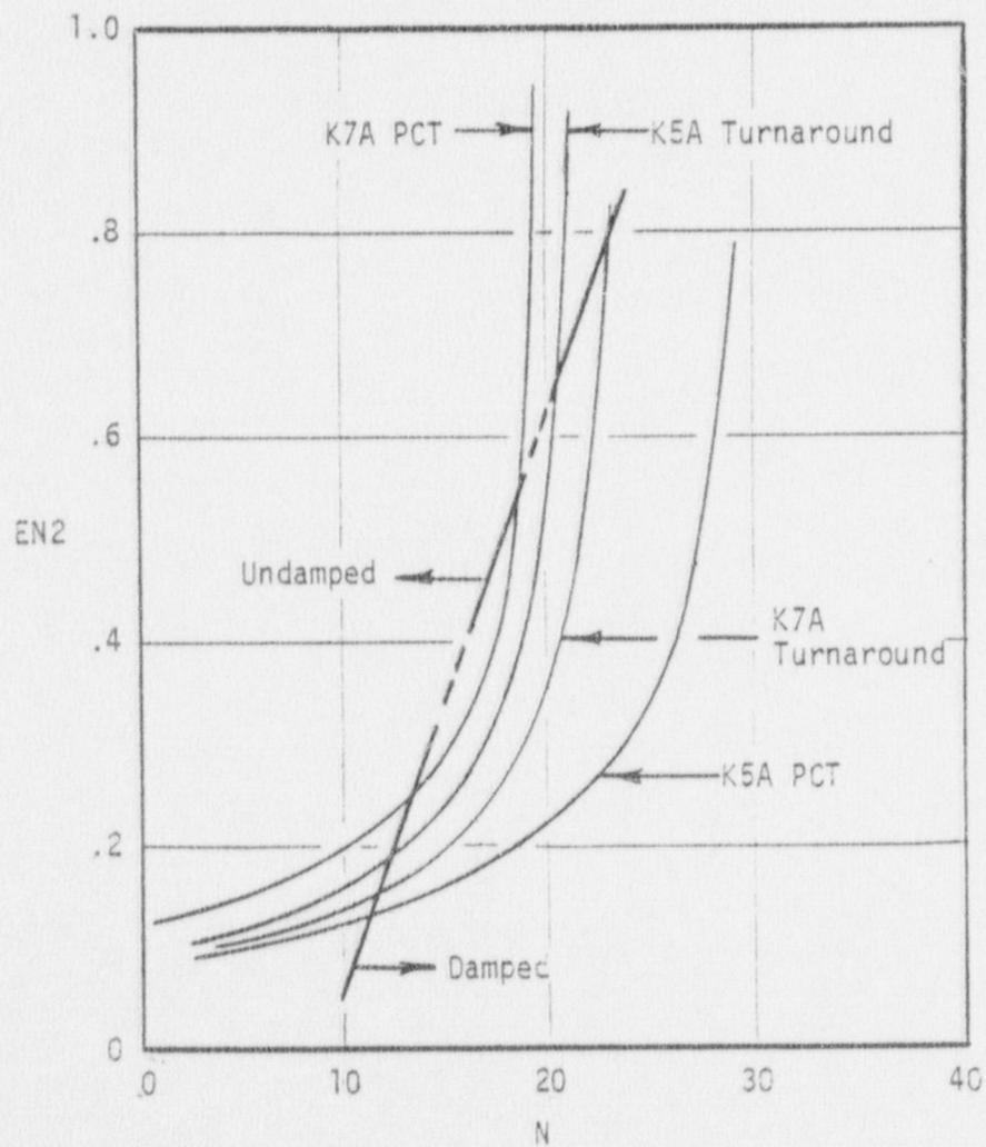
Fig. 68 N and EN2 relationships for PKL tests
