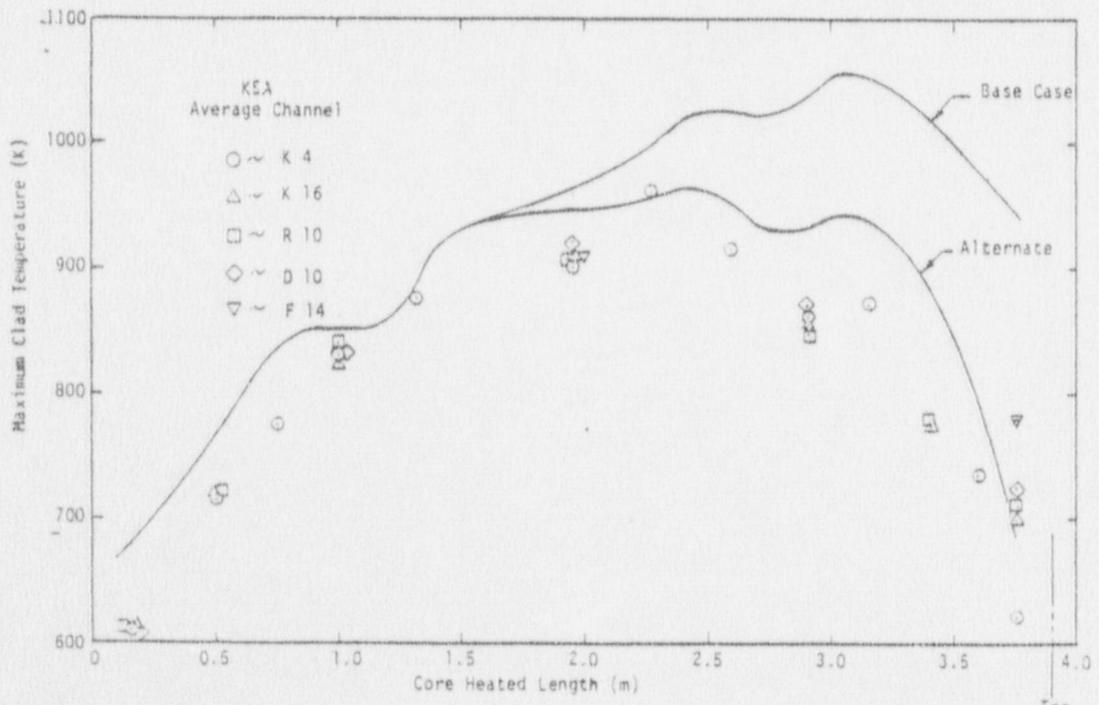
Fig. 14 Maximum rod surface temperature distribution over the core heated length, KSA average channel.
