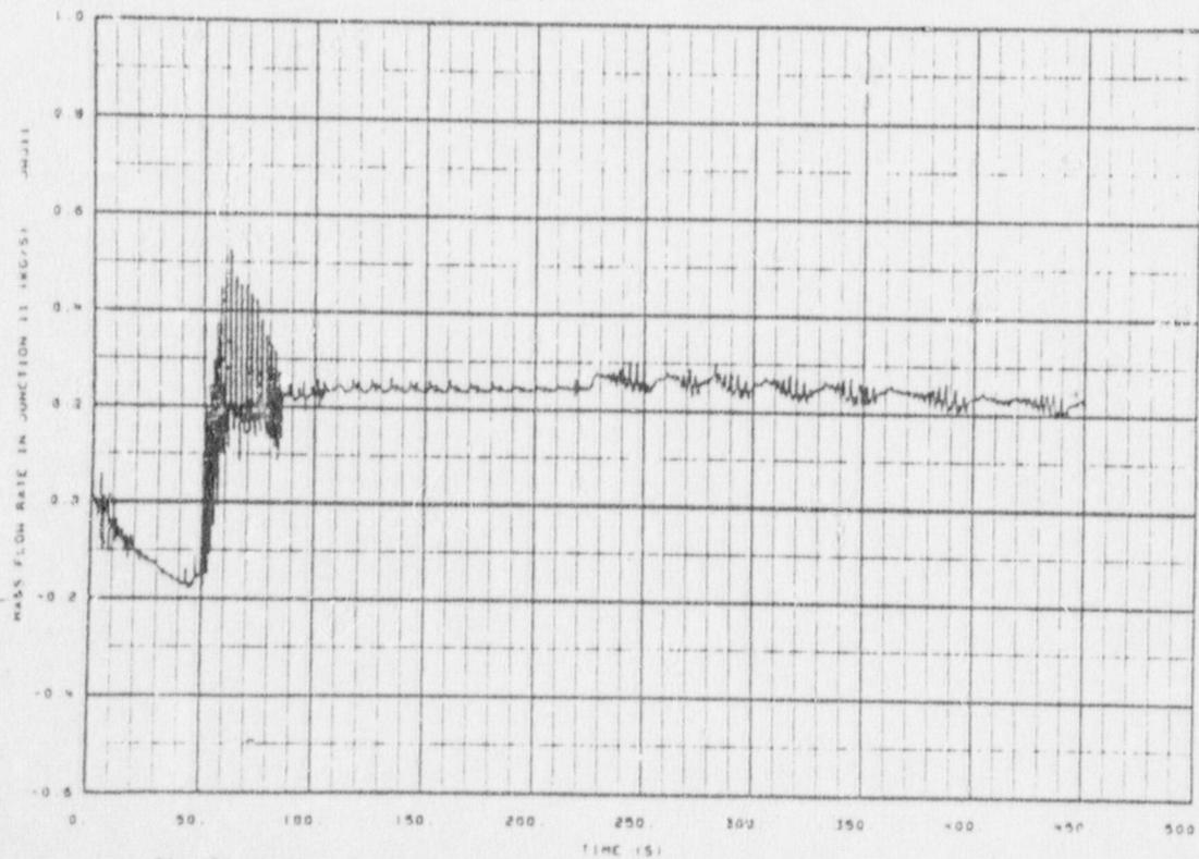
Fig. 57 Broken-loop cold-leg mass-flow-rate history as calculated by RELAP4/MOD6 (3) for Test K7A.
