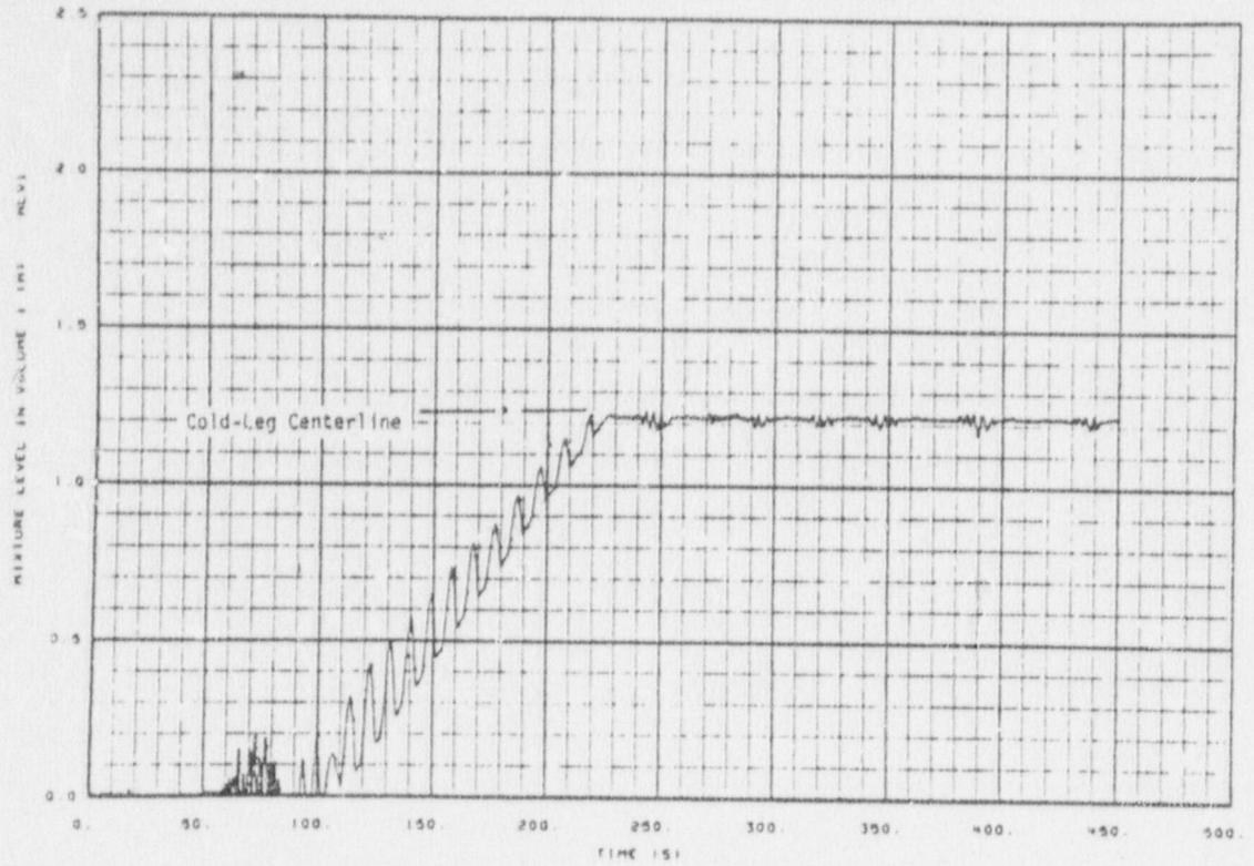
Fig. 54 Mixture level history in the upper annulus as calculated by RELAP4/MOD6 (3) for Test K7A.
