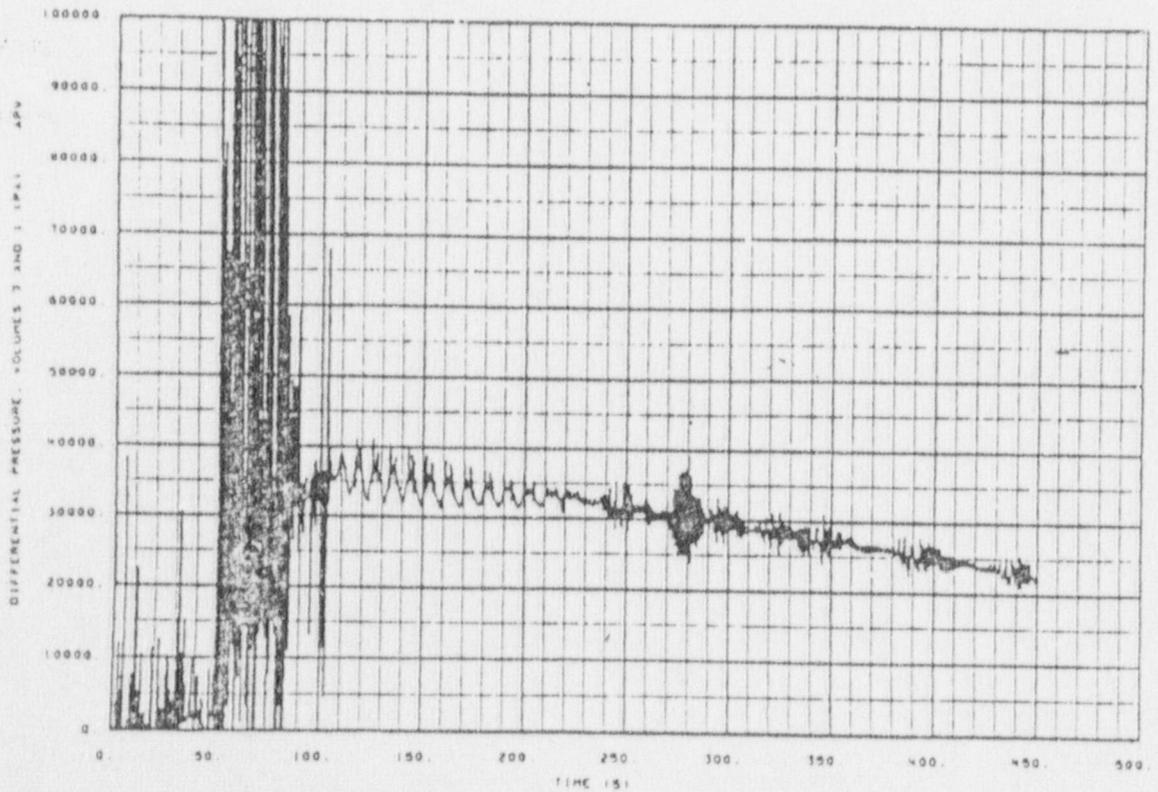
Fig. 63 Differential pressure between upper plenum and upper annulus as calculated by RELAP4/MOD6 (3) for Test K7A.
