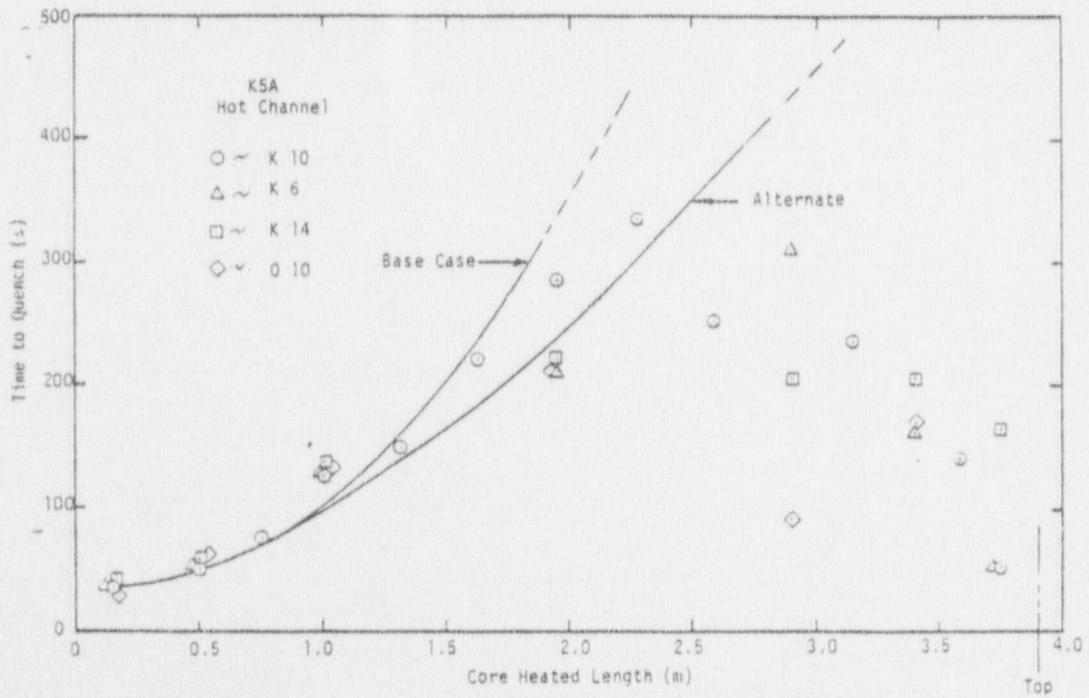
Fig. 22 Time to quench vs. core heated length, K5a hot channel.
