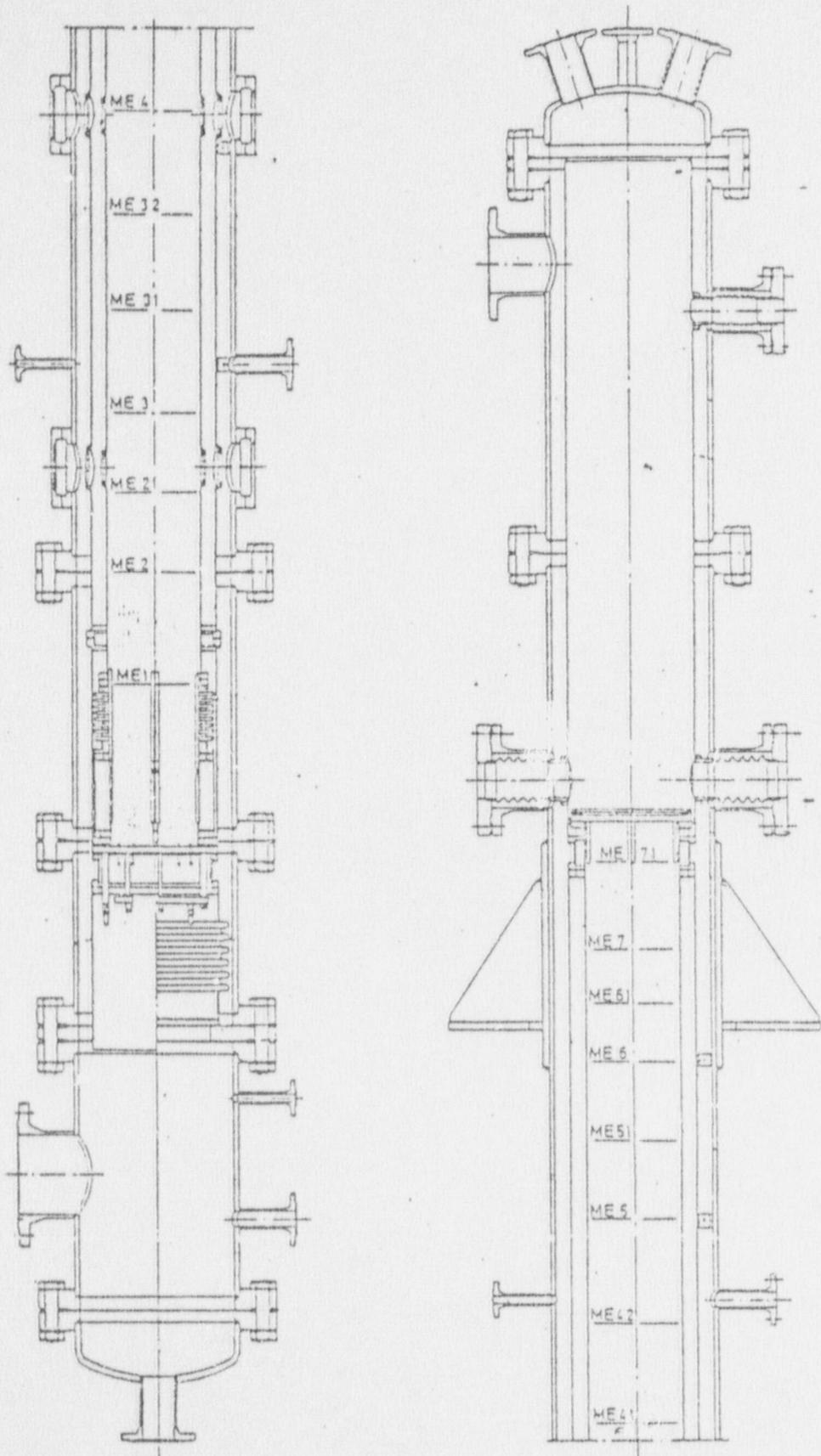
Fig. 7 Vessel layout showing core cladding thermocouple locations
