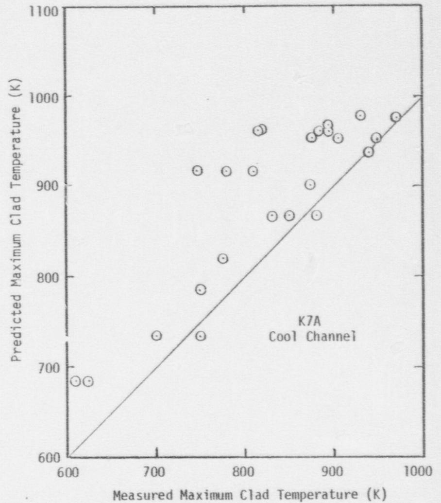
Fig. 44 Predicted vs. measured rod surface temperature, K7A cool channel.
