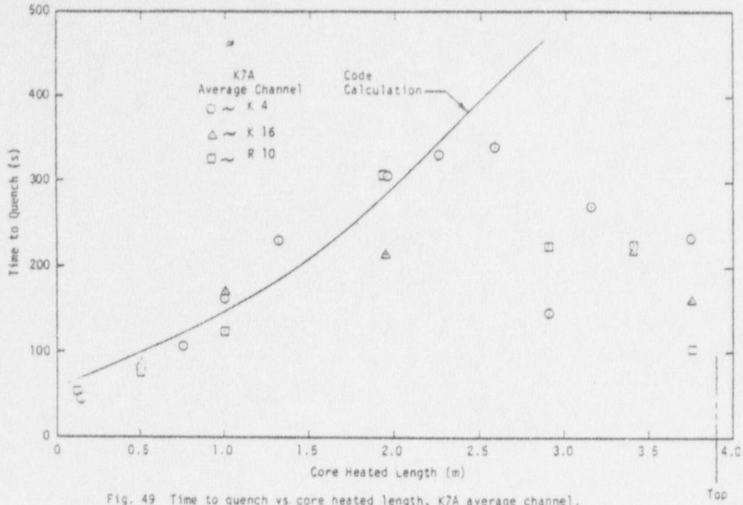
Fig. 49 Time to quench vs core heated length, K7A average channel.
