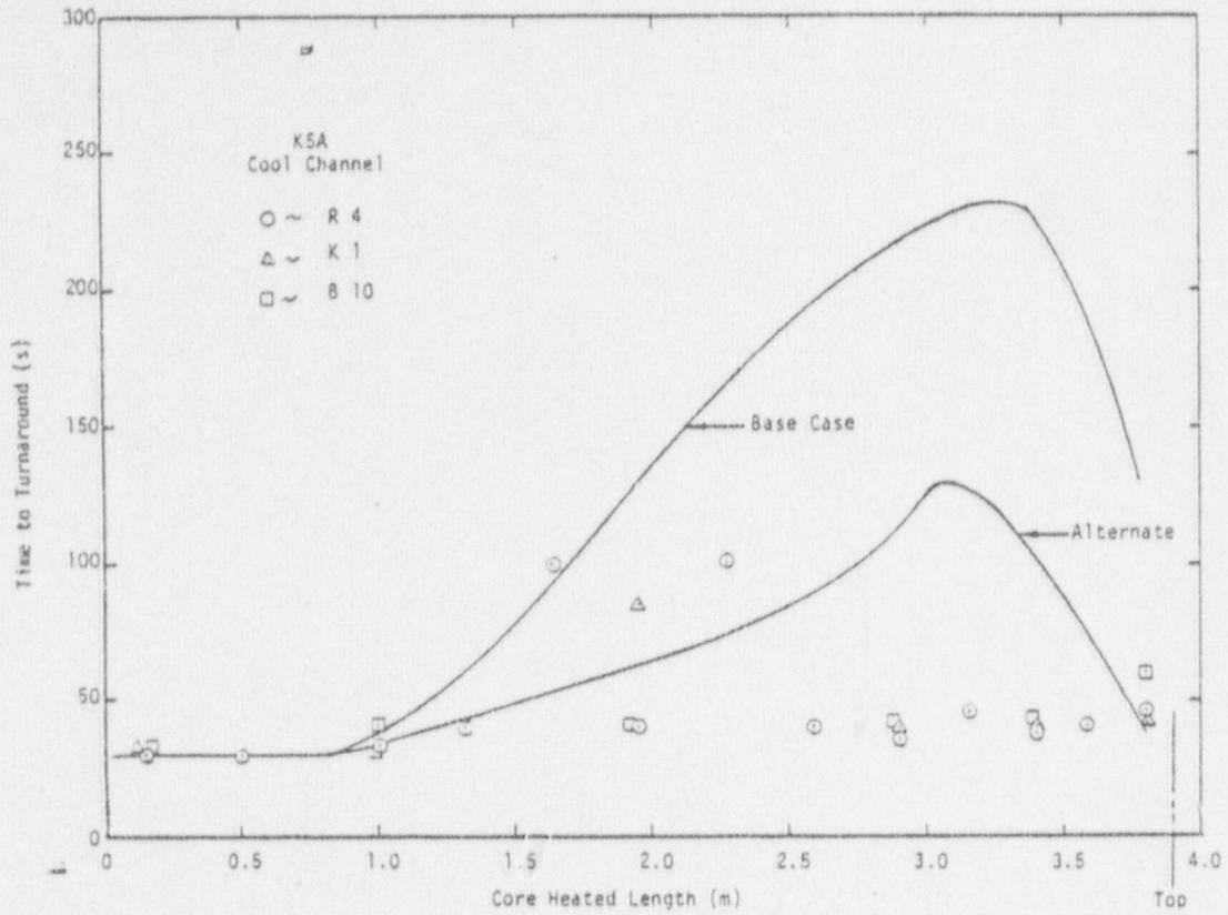
Fig. 21 Time to turnaround vs. core heated length, K5a cool channel.
