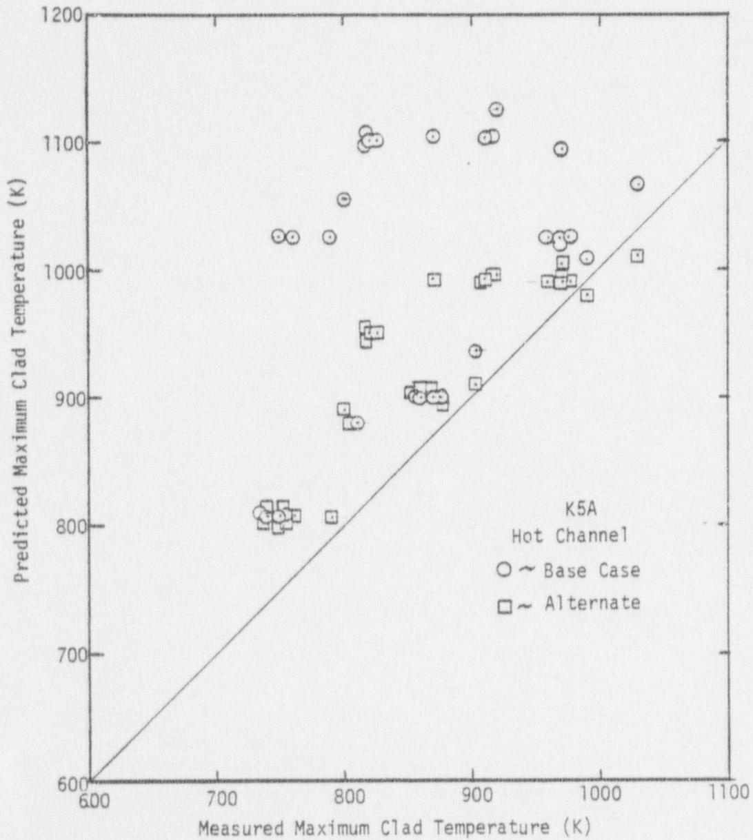
Fig. 16 Predicted vs. measured rod surface temperature, K5A hot channel.
