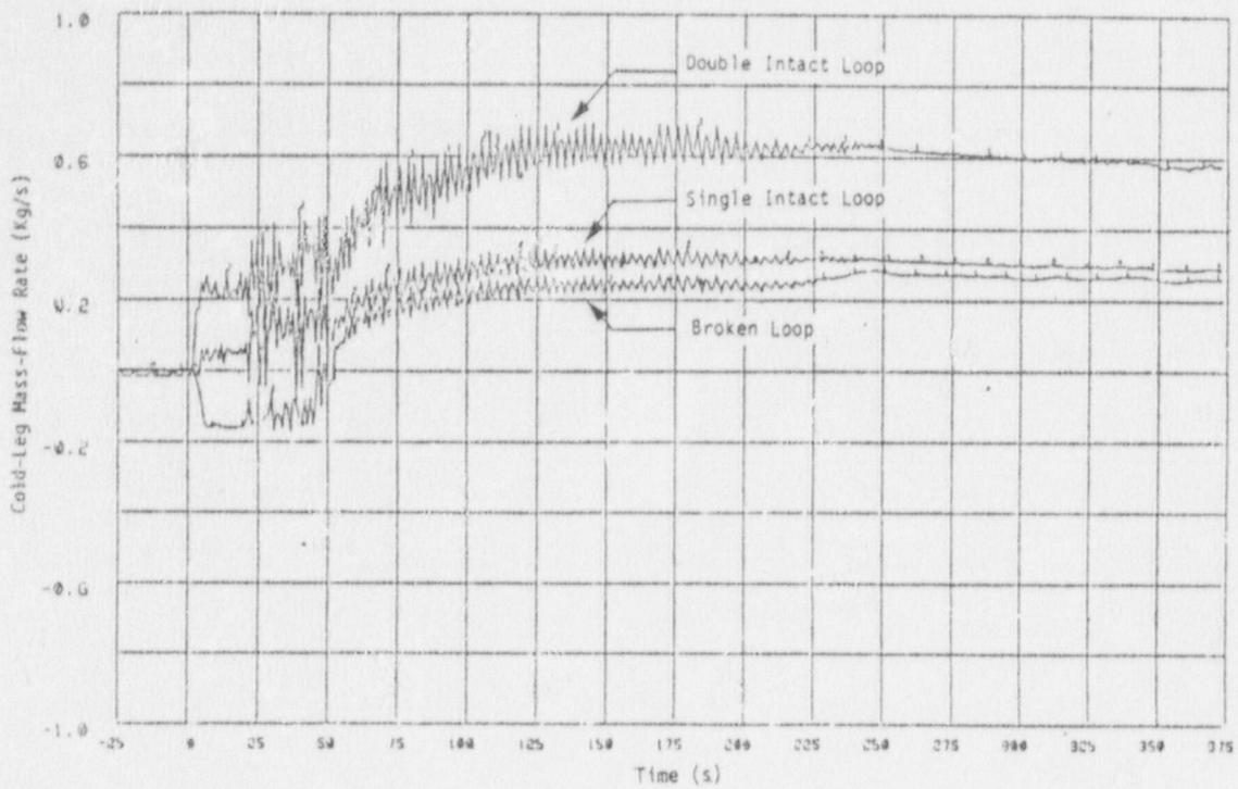
Fig. 56 Experimental cold-leg mass-flow-rate history for Test K7A.
