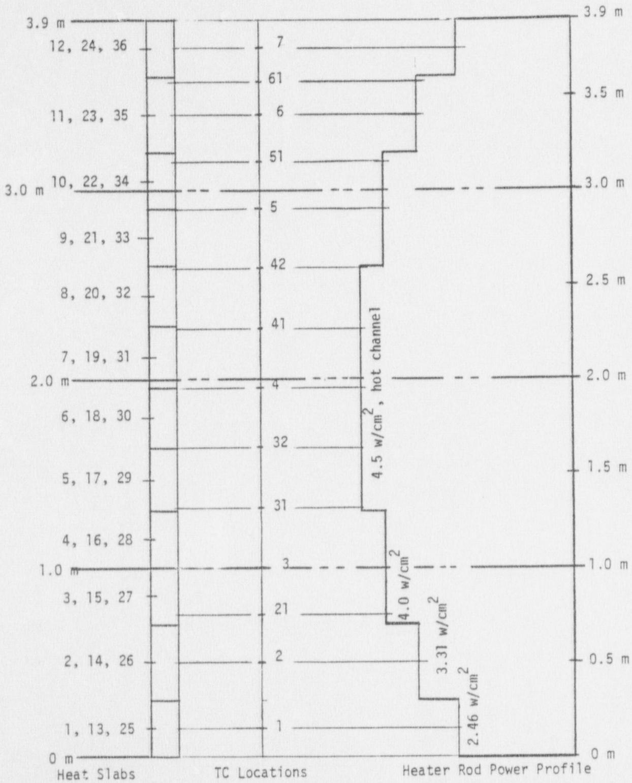
Fig. 10 Relationship of heat-slab centers to rod thermocouple locations.
