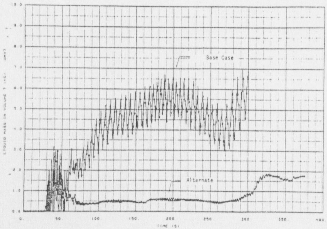
Fig. 27 Total mass in the upper plenum as calculated by RELAP4/MO06 (3) for Test K5A.
