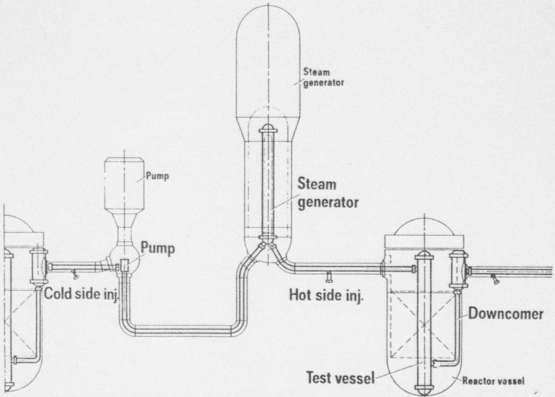
Fig. 2 Simulation concept for the PKL vessel and loops.
