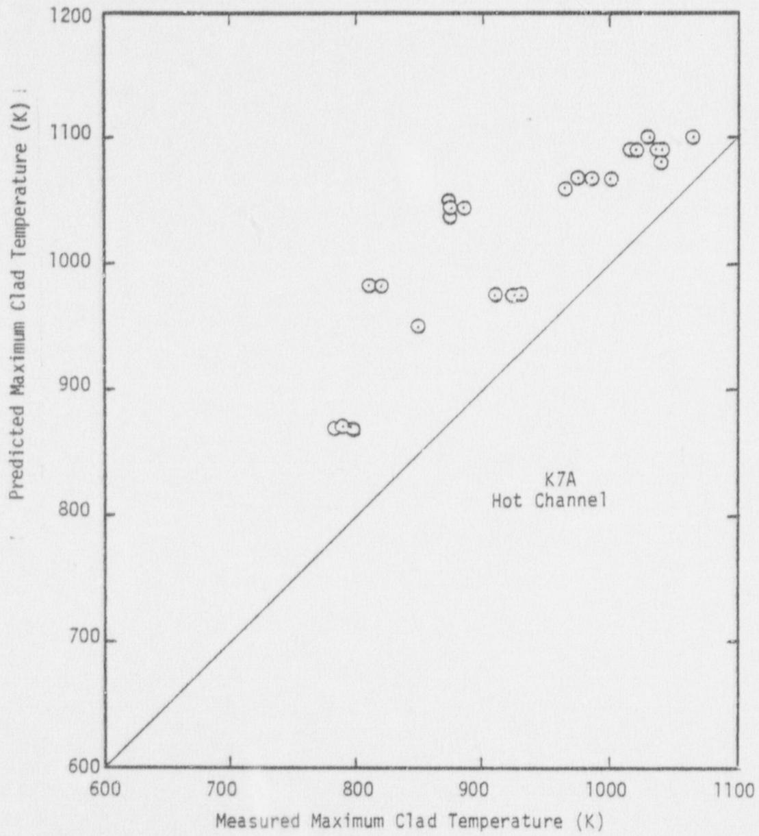
Fig. 42 Predicted vs. measured rod surface temperature, K7A hot channel.
