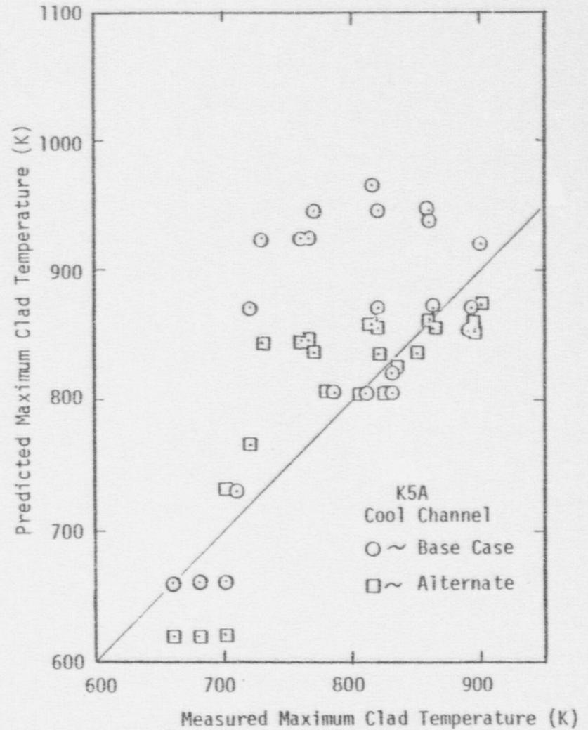
Fig. 18 Predicted vs. measured rod surface temperature, K5A cool channel.
