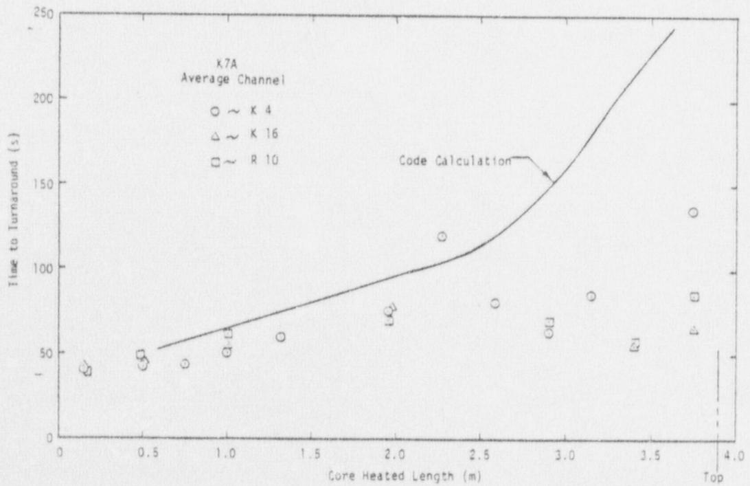
Fig. 46 Time to turnaround vs. core heated length, K7A average channel.
