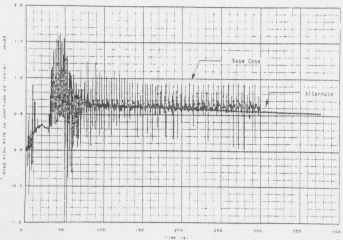
Fig. 33 Double-intact-loop cold-leg mass-flow-rate history as calculated by RELAP4/MOD6 (3) for Test KSA.
