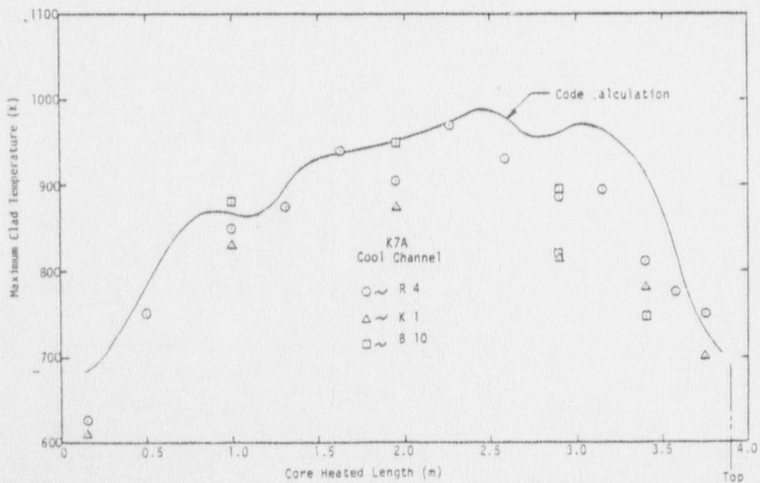
Fig. 41 Maximum rod surface temperature distribution over the core heated length, K7A cool channel.
