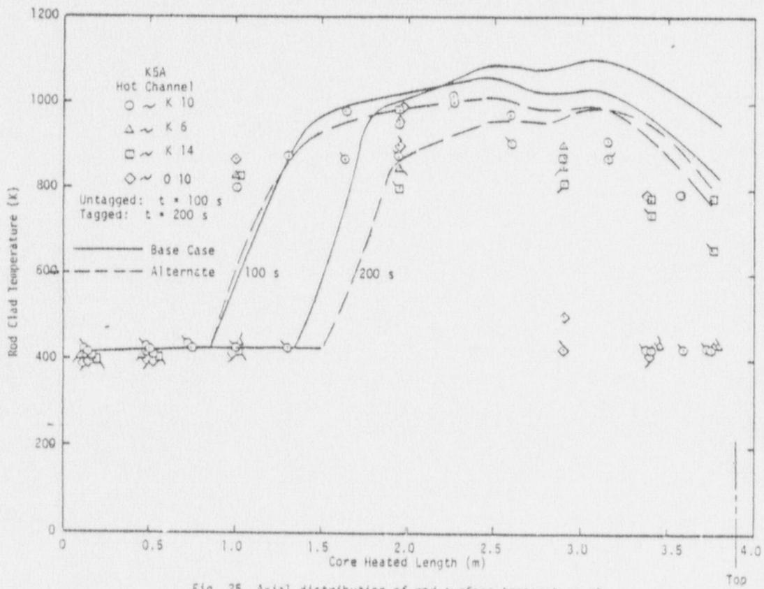
Fig. 25 Axial distribution of rod surface temperature at 100 s and 200 s, K5A hot channel.
