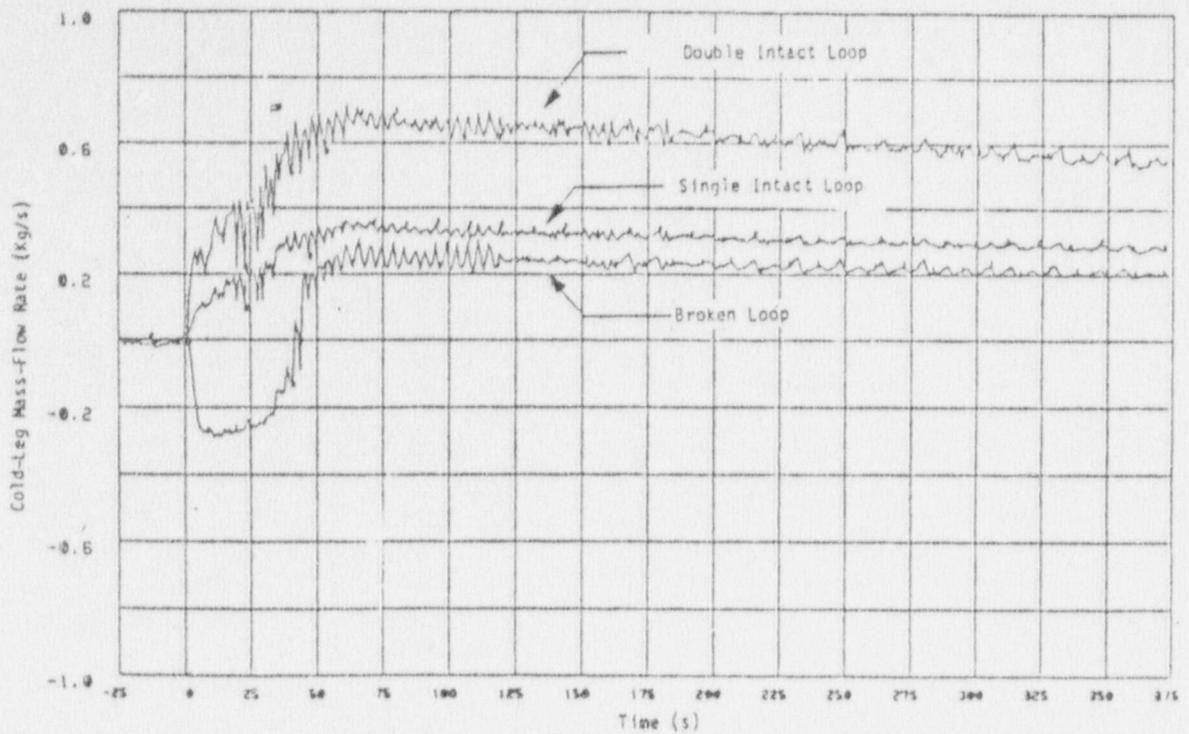
Fig. 30 Experimental cold-leg mass-flow-rate histories for Test K5A.
