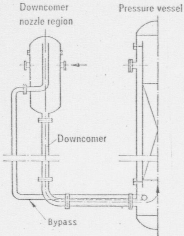
Fig. 5 Installation of downcomer steam bypass.
