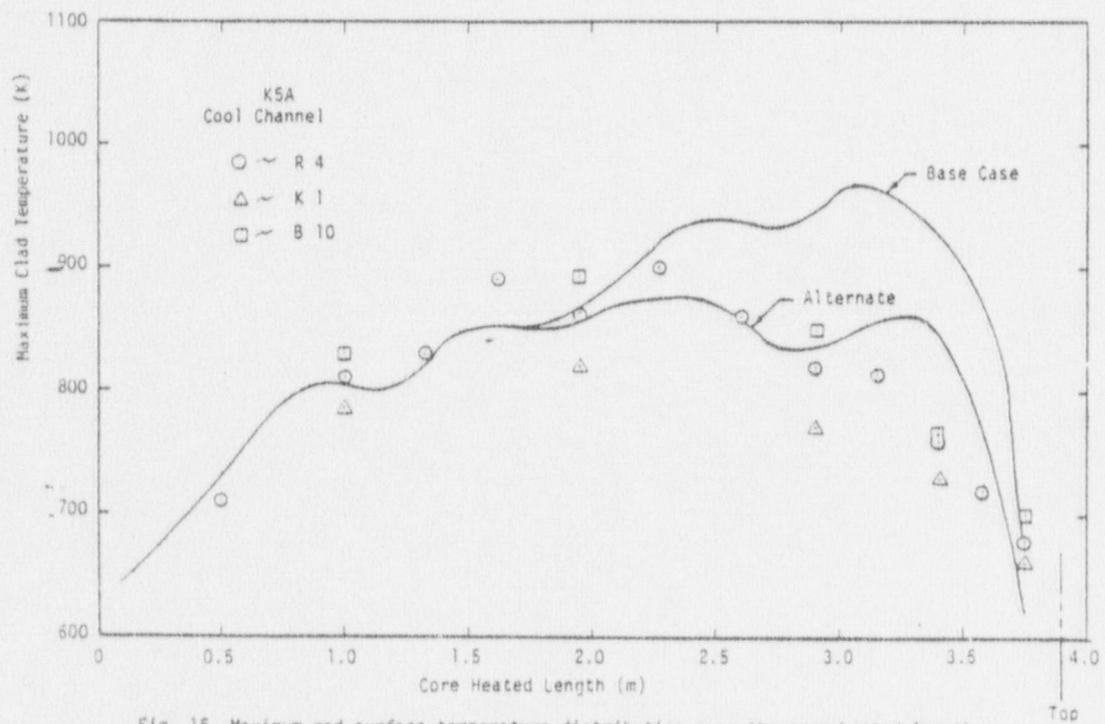
Fig. 15 Maximum rod surface temperature distribution over the core heated length, KSA cool channel.
