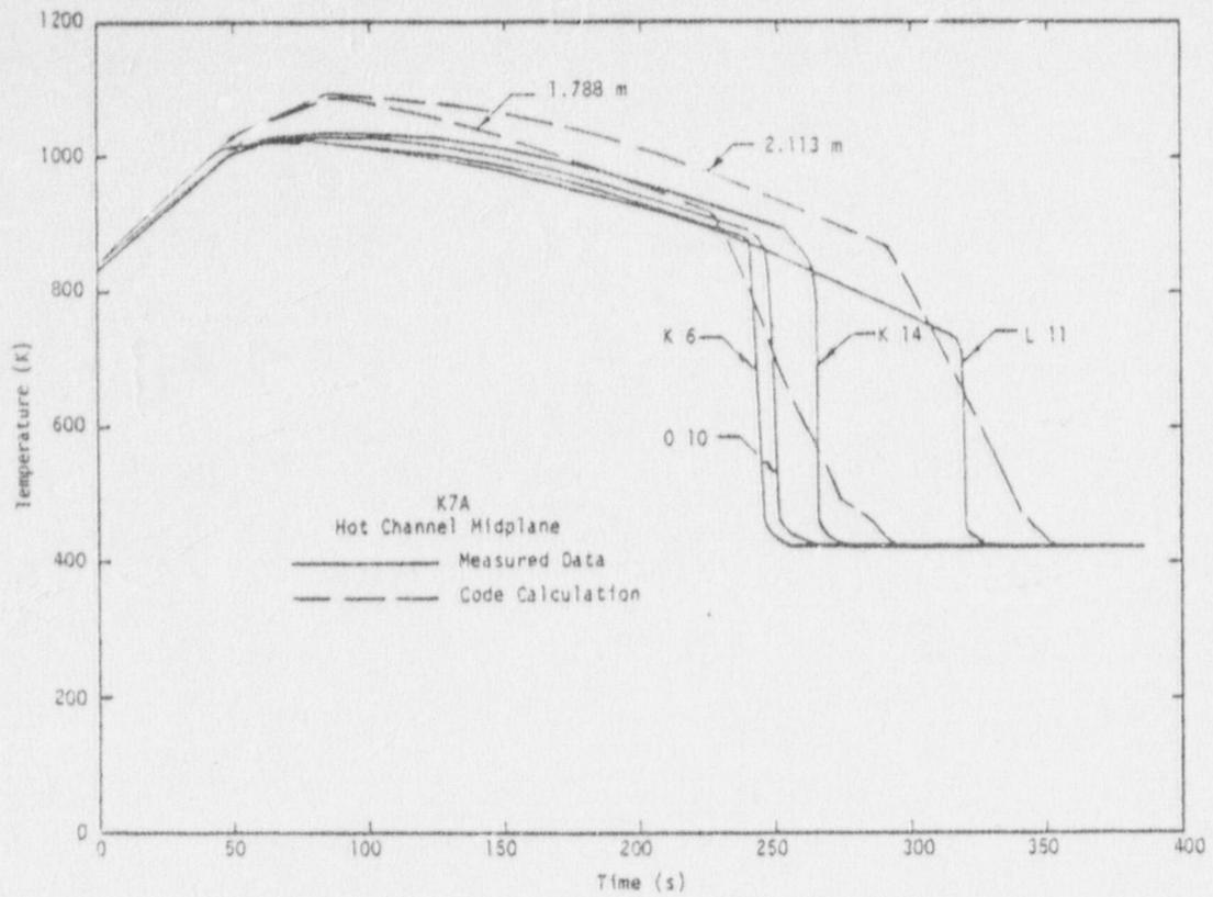
Fig. 38 Comparison of cladding temperature history at the midplane, Test K7A.
