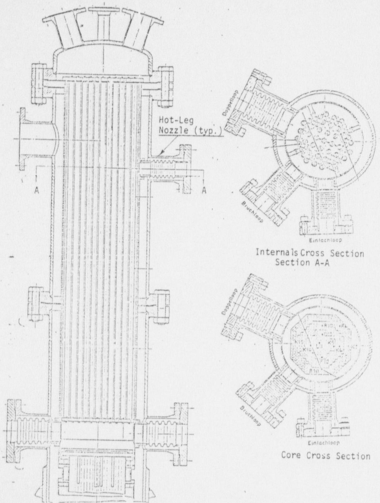
Fig. 4 Vessel upper plenum internals simulation.
