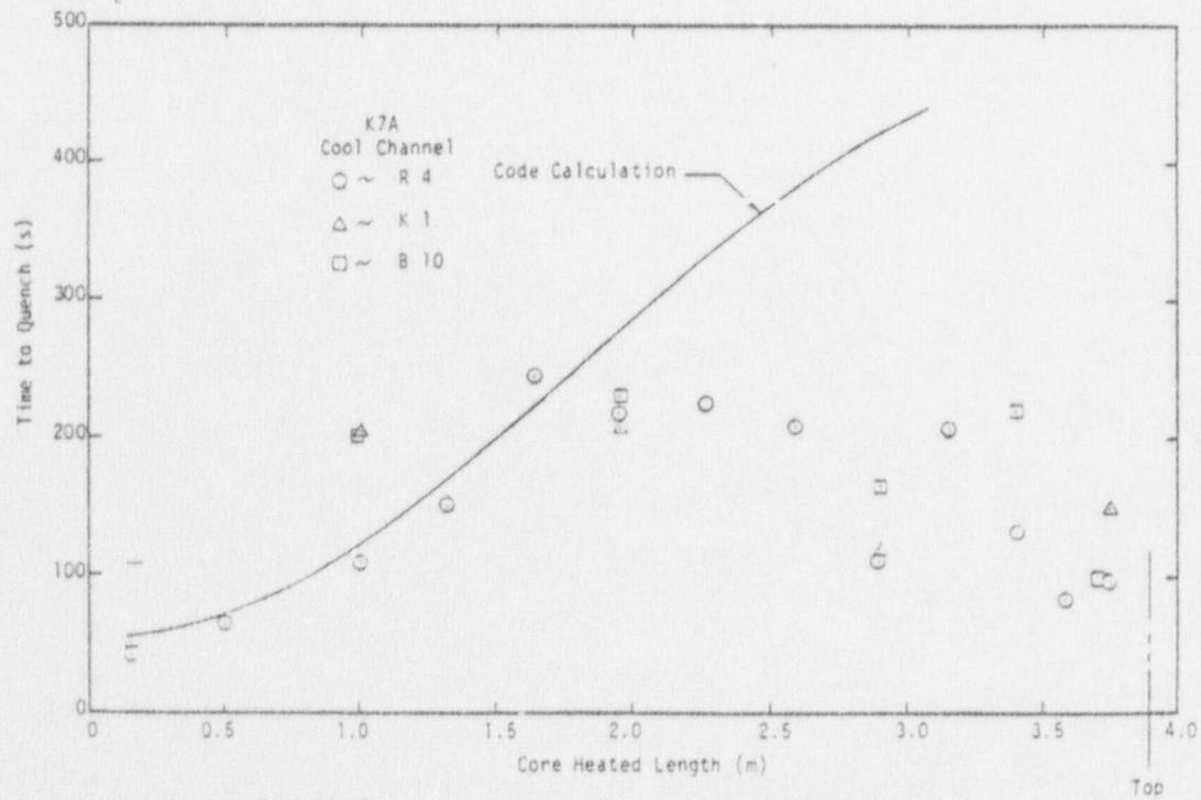
Fig. 50 Time to quench vs core heated length, K7A cool channel.
