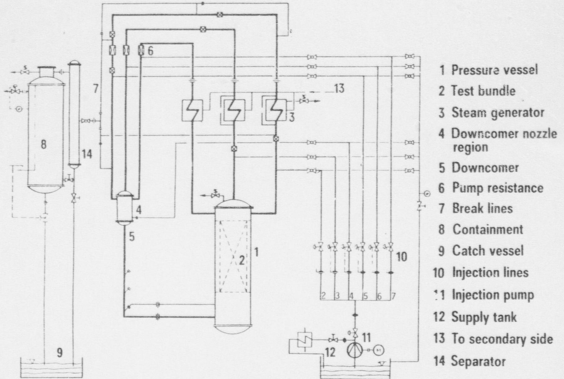
Fig. 1 Schematic of the PKL test facility.
