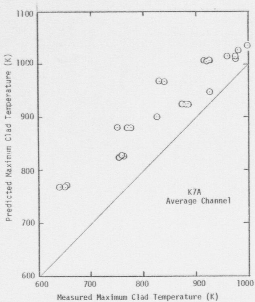
Fig. 43 Predicted vs. measured rod surface temperature, K7A average channel.
