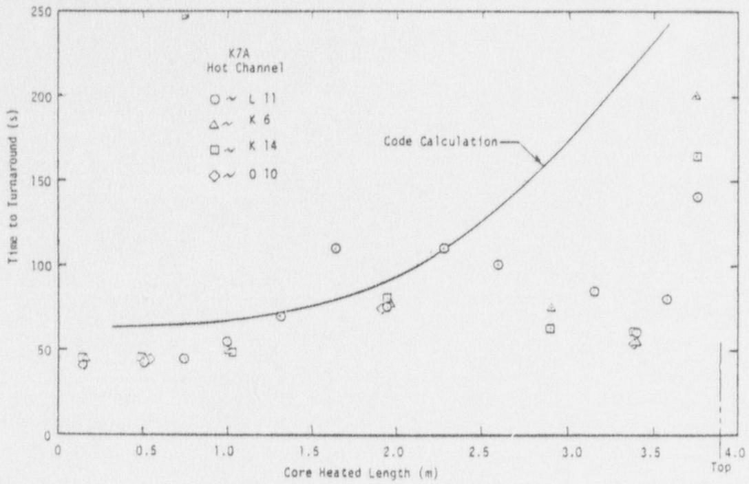
Fig. 45 Time to turnaround vs. core heated length, K7A hot channel.
