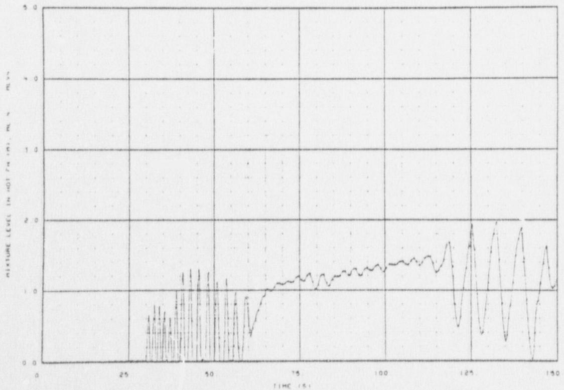
Fig. 65 Core hot-channel mixture-level history when steam-generator inlet-side primary volumes were divided in half.
