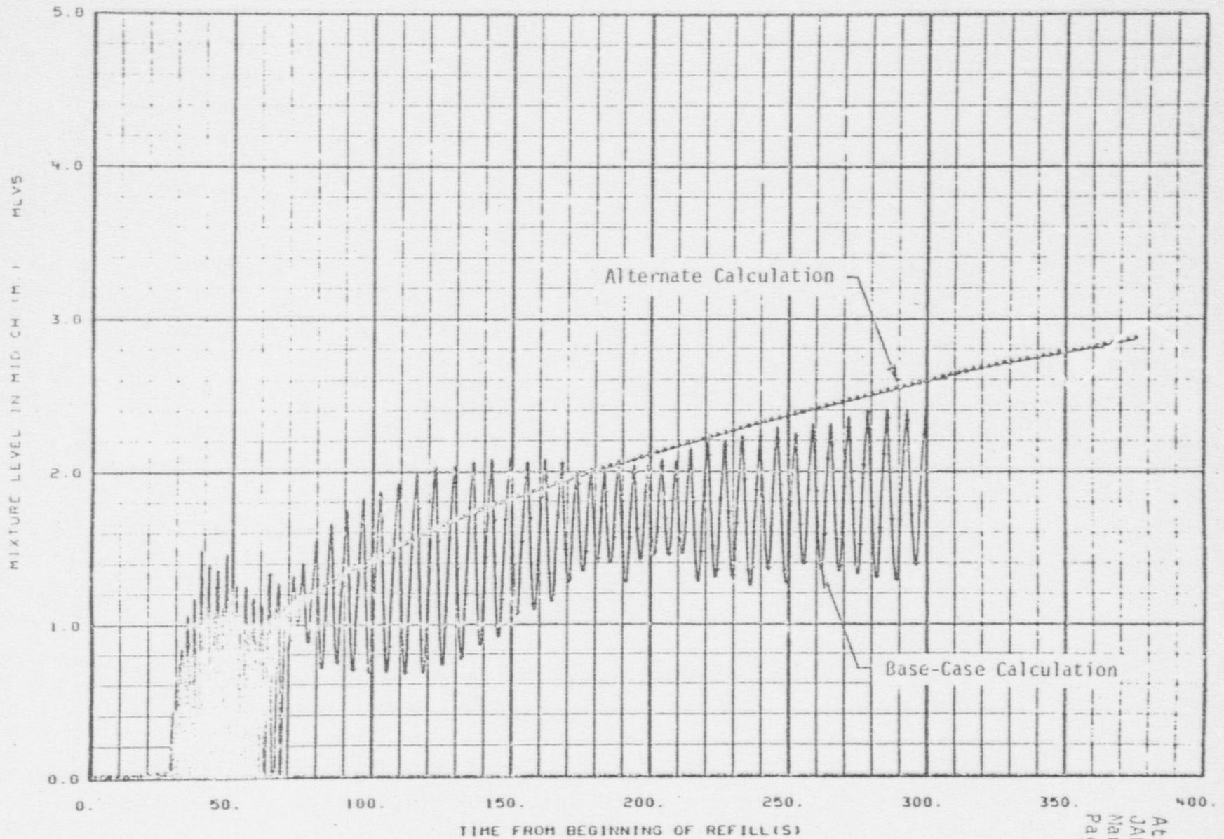
Fig. 19 Average channel mixture level vs. time.
