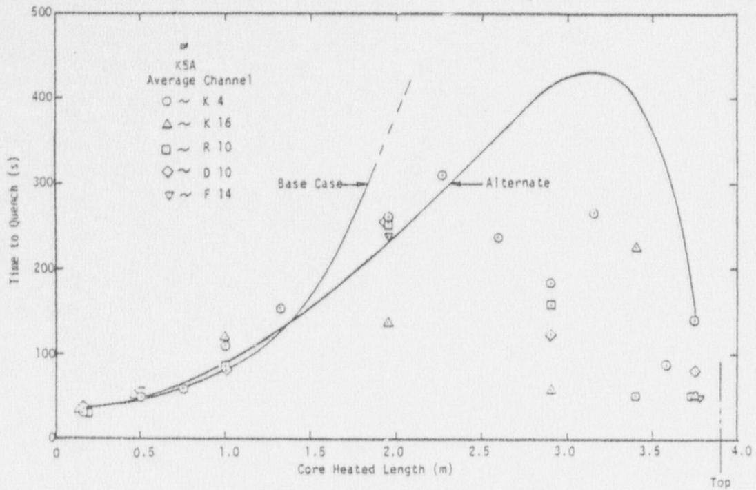
Fig. 23 Time to quench vs. core heated length, K5A average channel.
