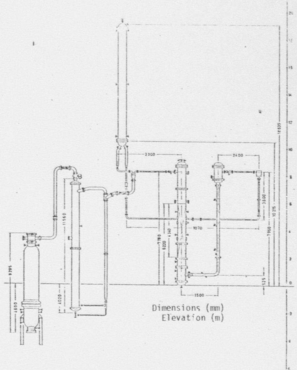
Fig. 6 Elevation details for the PKL broken loop.
