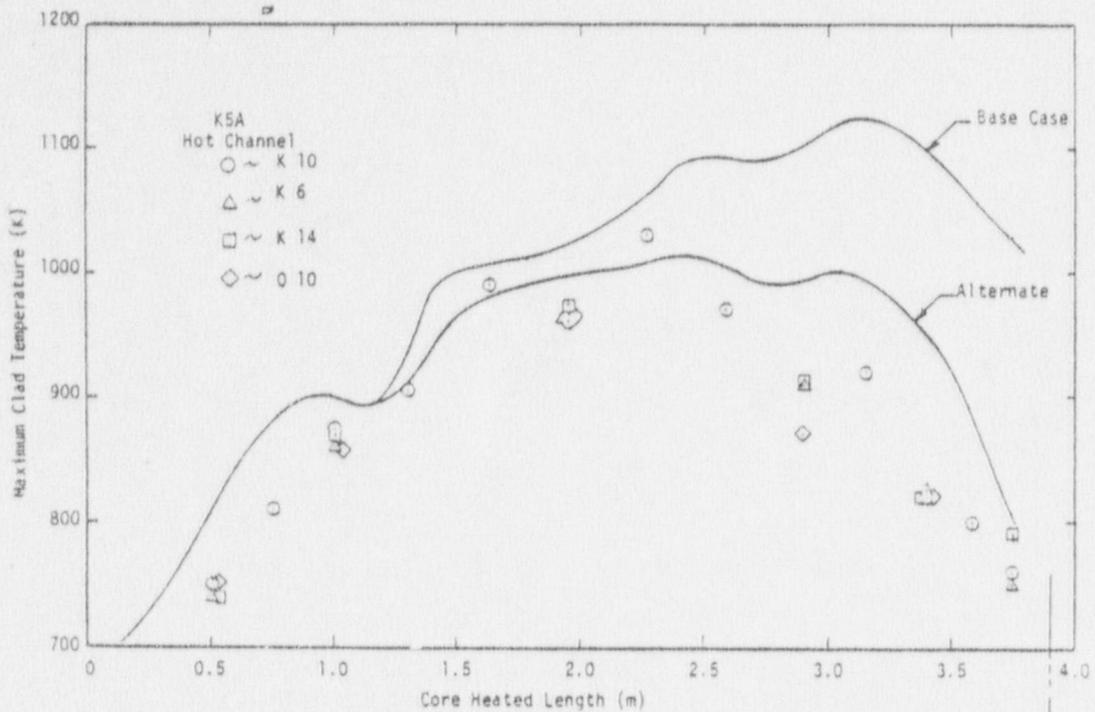
Fig. 13 Maximum rod surface temperature distribution over the core heated length, KSA hot channel.
