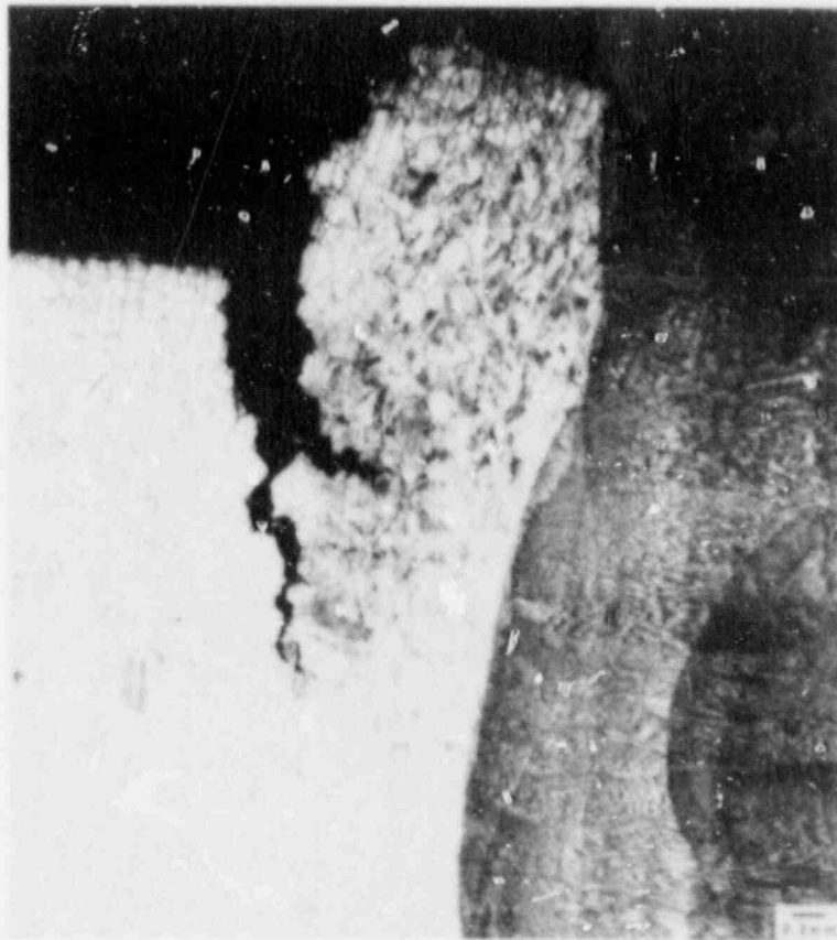
Fig. 5. Cross Section of a 1TCT Weld Overlay Specimen Showing Crack Branching and Propagation in the Base Material near the Weld Fusion Line.
