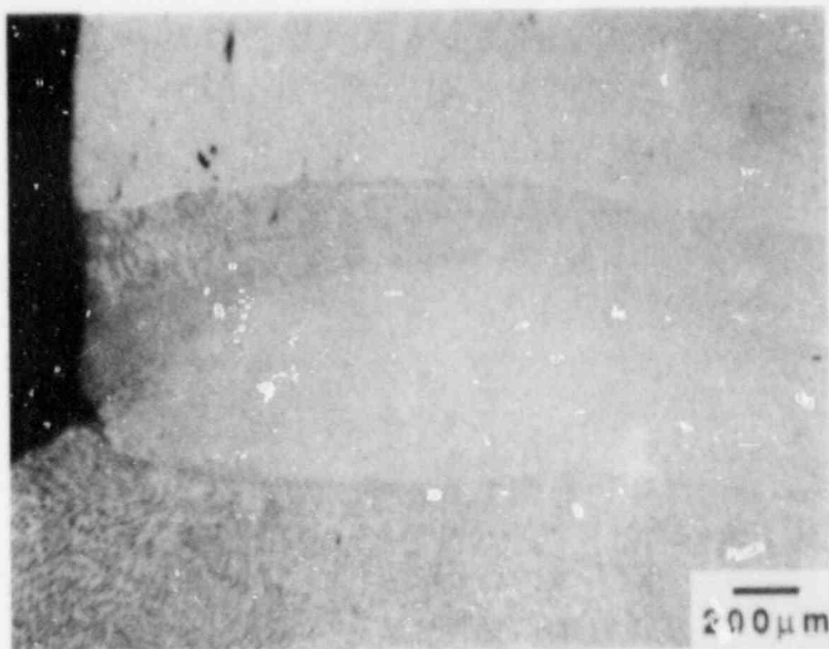
Fig. 11. Cross Section of Weld Showing the Crack and the Metallurgical Changes in the Heat-Affected Zone.
