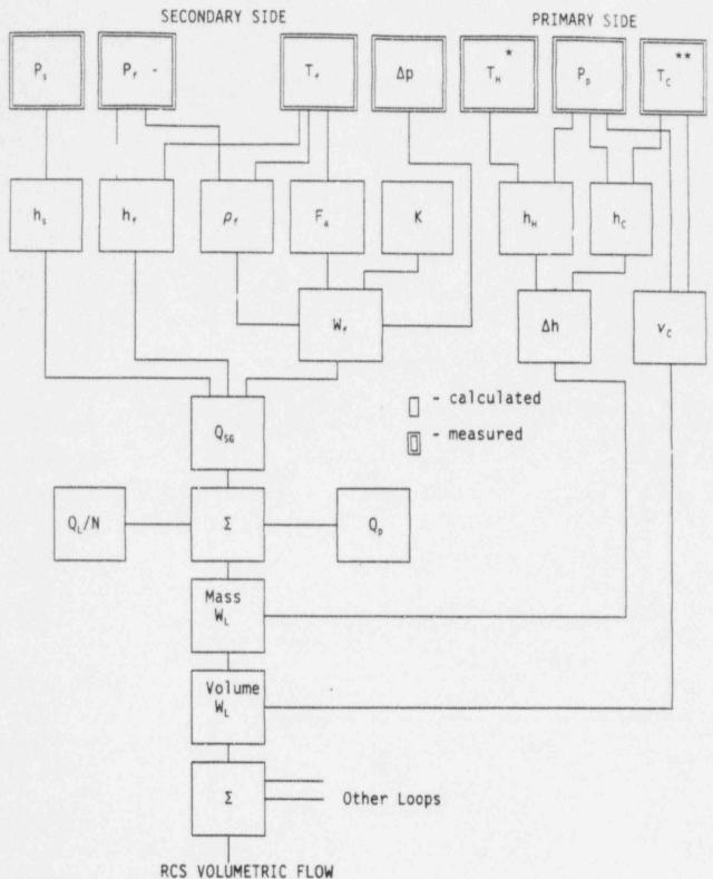
\* Three hot leg temperatures per loop are measured and averaged.
