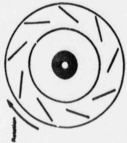
BACKWARD INCLINED (forward curved) FAN INVENTED BY WESTINGHOUSE
