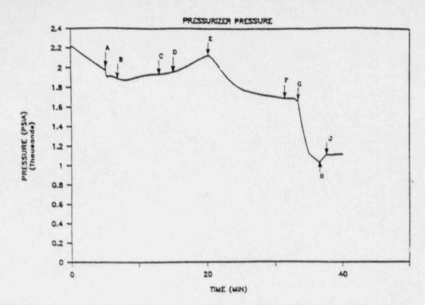
FIGURE 10-1. CPSES1 Design-Basis SGTR, Overfill - Pressurizer Pressure
