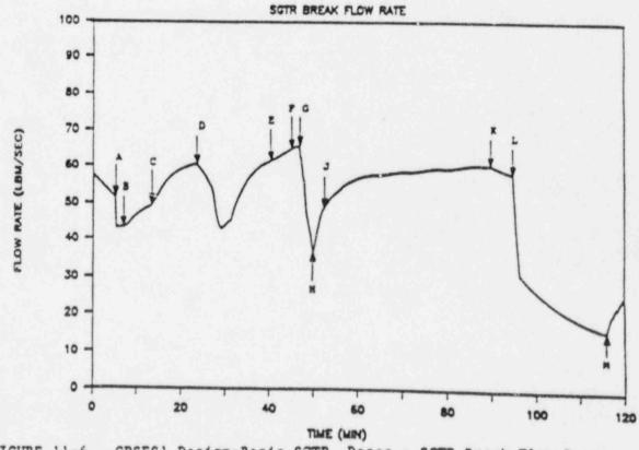
FIGURE 11-6. CPSES1 Design-Basis SGTR, Doses - SGTR Break Flow Rate
