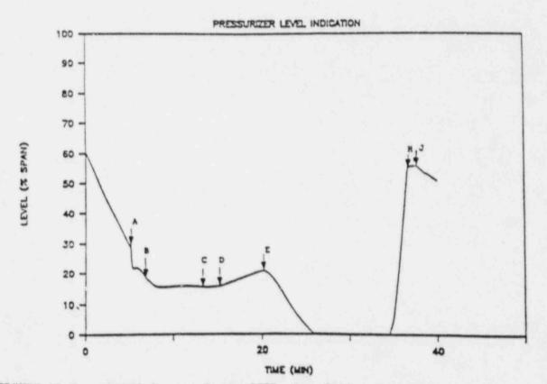
FIGURE 10-2. CPSES1 Design-Basis SGTR, Overfill - Pressurizer Level
