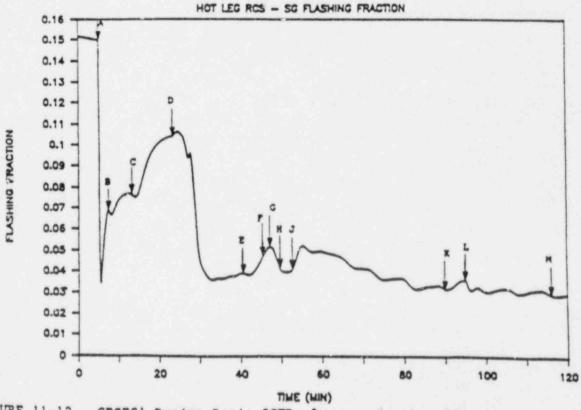
FIGURE 11-12. CPSES1 Design-Fasis SGTR, Doses - Hot Leg Flashing Fraction 11-37
