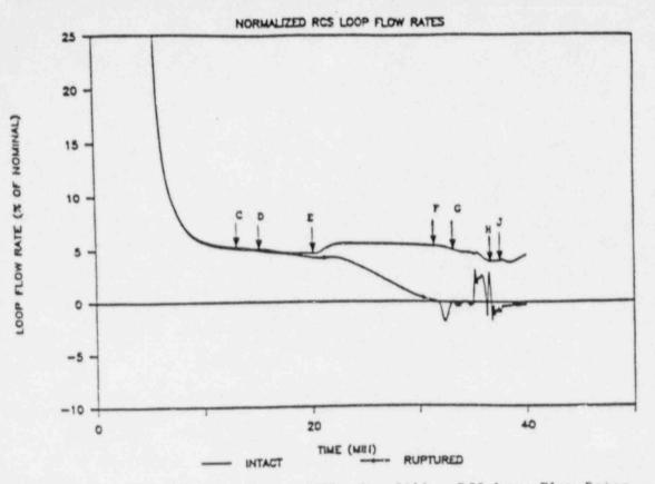
FIGURE 10-9. CPSES1 Design-Basis SGTR, Overfill - RCS Loop Flow Rates
