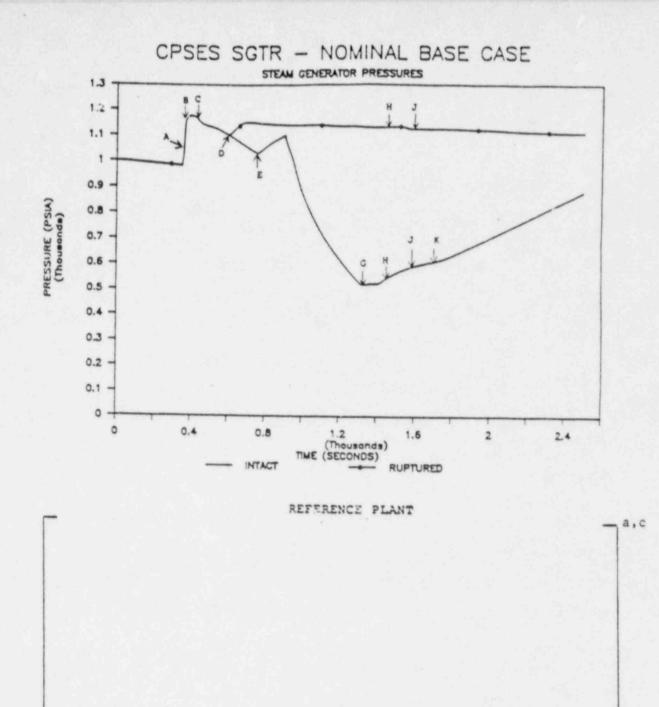
FIGURE 6-6. Nominal Base Case Comparison - Steam Generator Pressures
