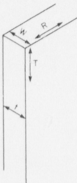
Fig. 19. Through-the-thickness depth location notations in AQ 03 and AQ 04 plates.
