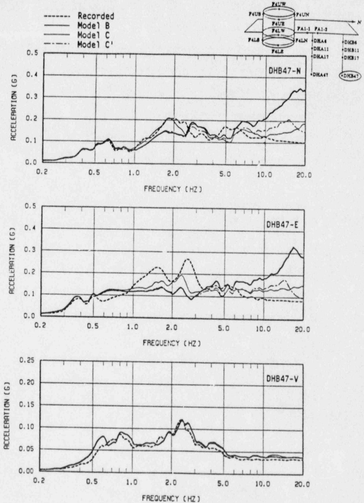
Figure 16. Acceleration Response Spectra at DHB47 for May 20, 1986 Earthquake ( $\lambda=5\%$ )
