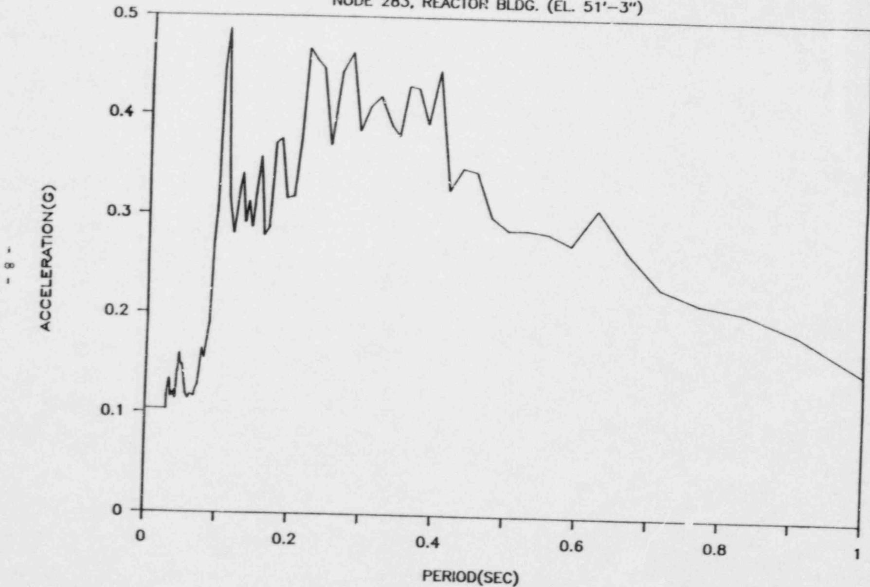
FIGURE 5 RAW ENVELOPED VERTICAL SSE SPECTRUM FOR SLAB PANEL BETWEEN COLUMN LINES RA/RB AND R3/R4, EL. 51'-3" OF THE REACTOR BUILDING
