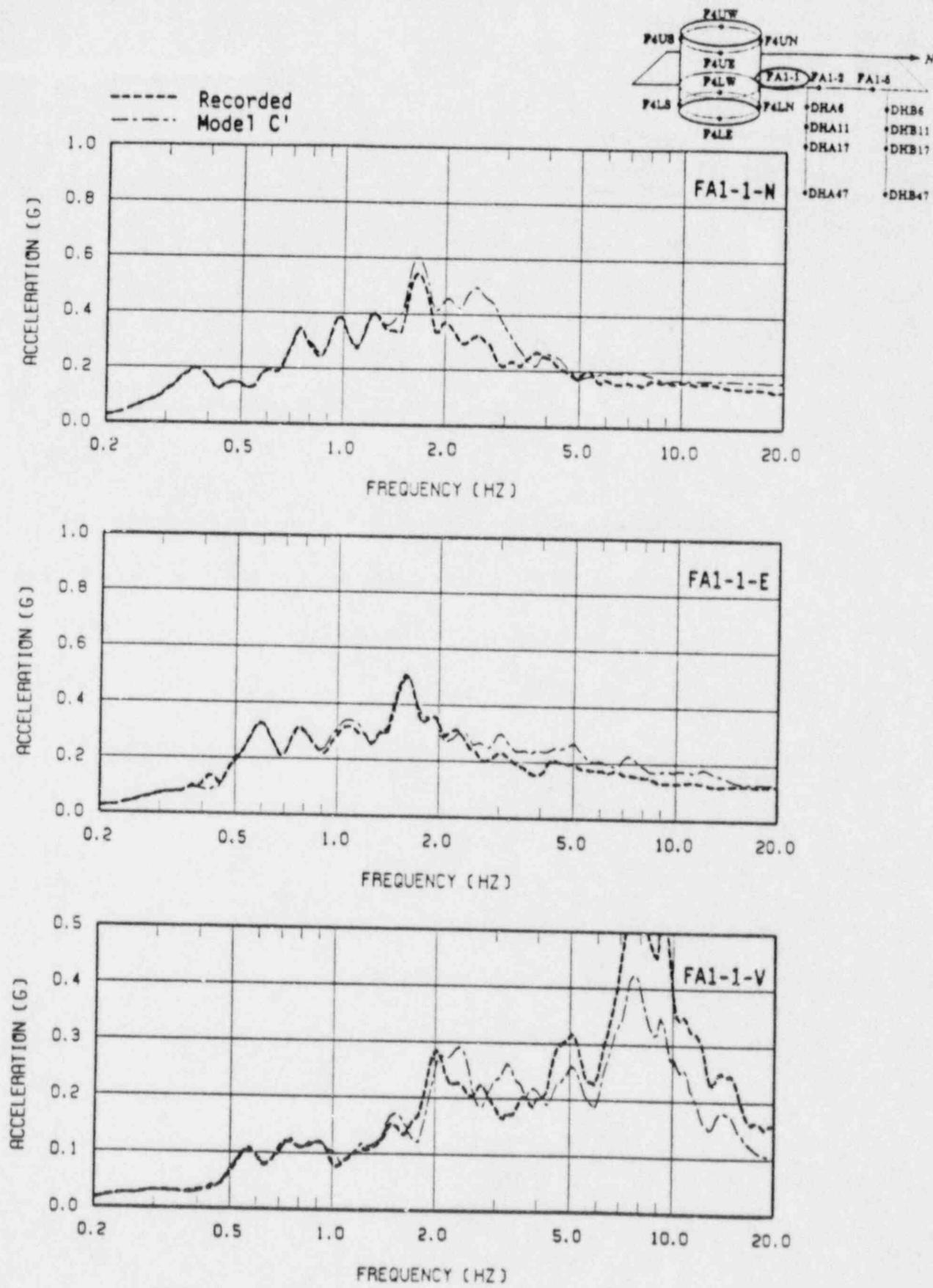
Figure 33. Acceleration Response Spectra at FA1-1 for Nov. 14, 1986 Earthquake ( $\lambda=5\%$ )
