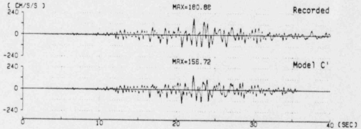
Figure 36. Acceleration Time Histories of F4US-E for Nov. 14, 1986 Earthquake
