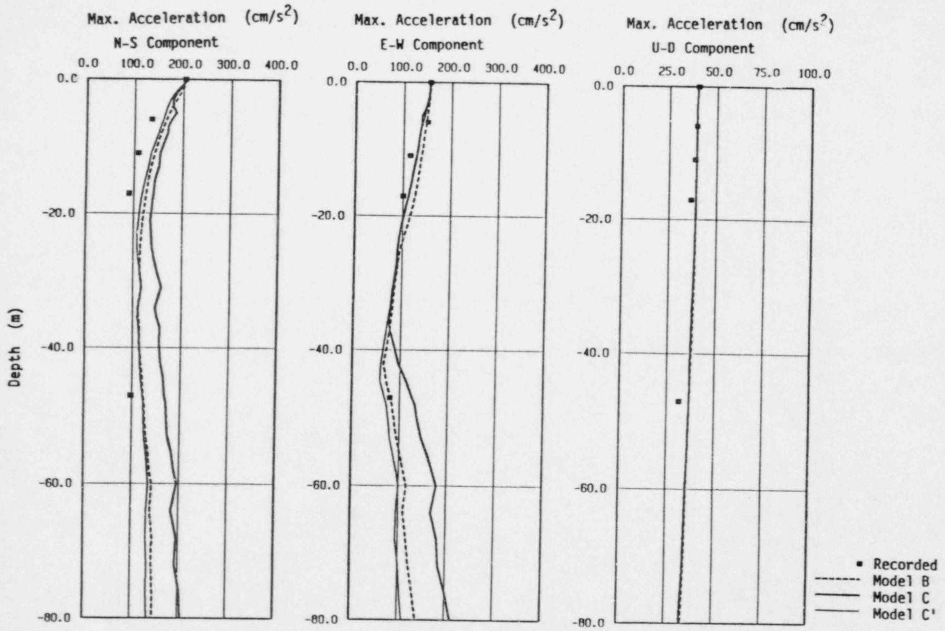
Figure 14. Maximum Ground Acceleration for May 20, 1986 Earthquake
