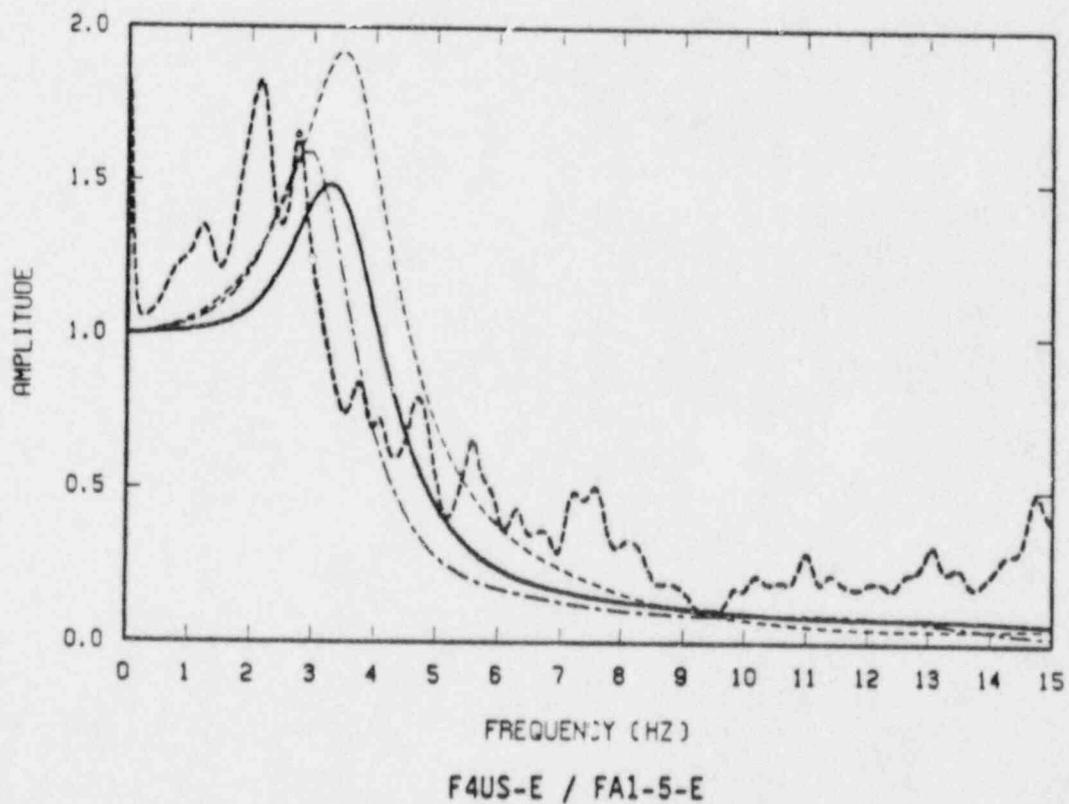
Figure 20. Transfer Functions for May 20, 1986 Earthquake (F4US-E/FA1-5-E)
