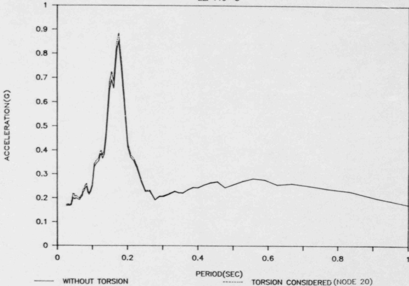
Figure 2 Floor Response Spectra at Operating Floor.(El. +119'-3")
