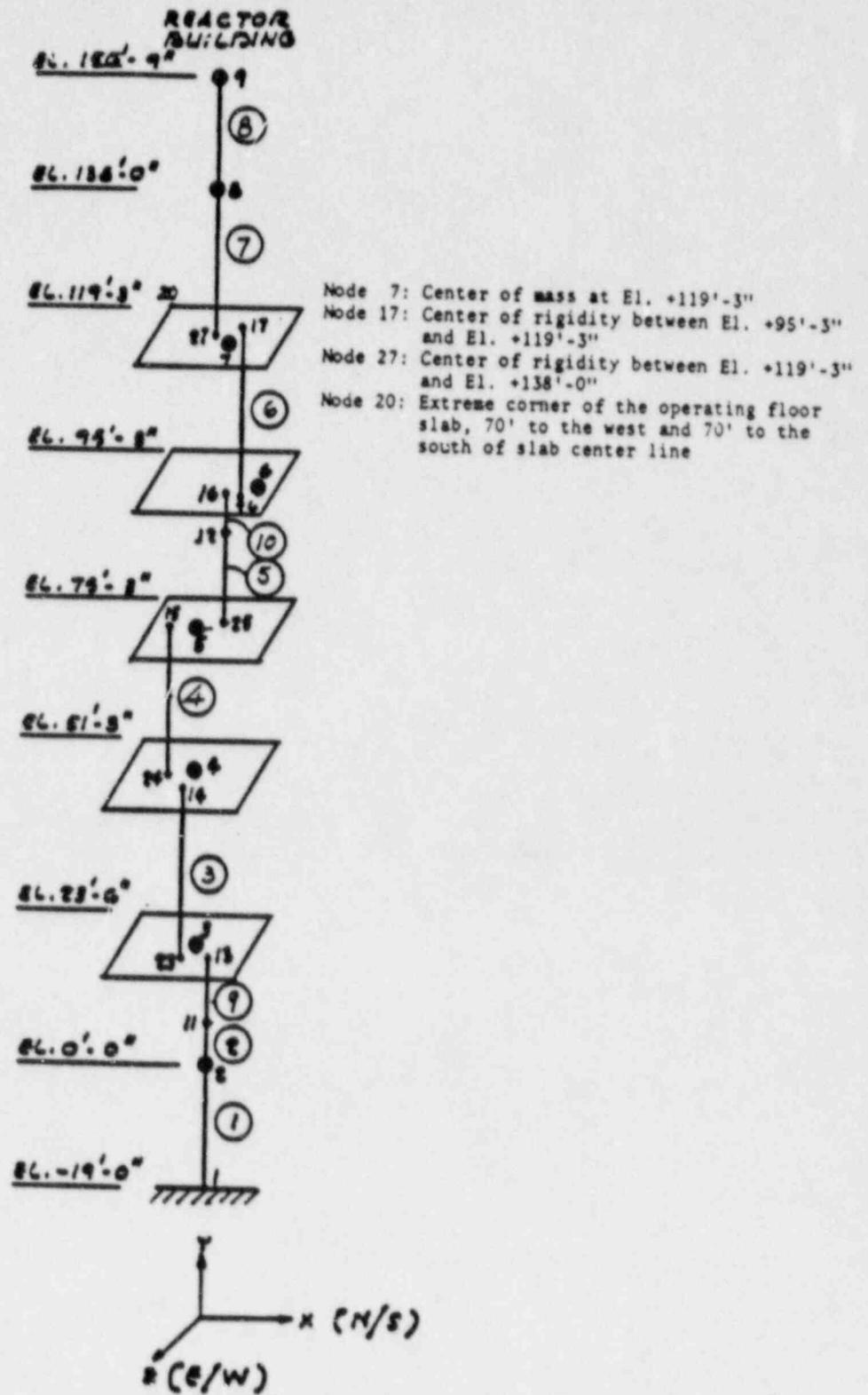
Figure 1 3-D Lumped-mass Model of Reactor Building
