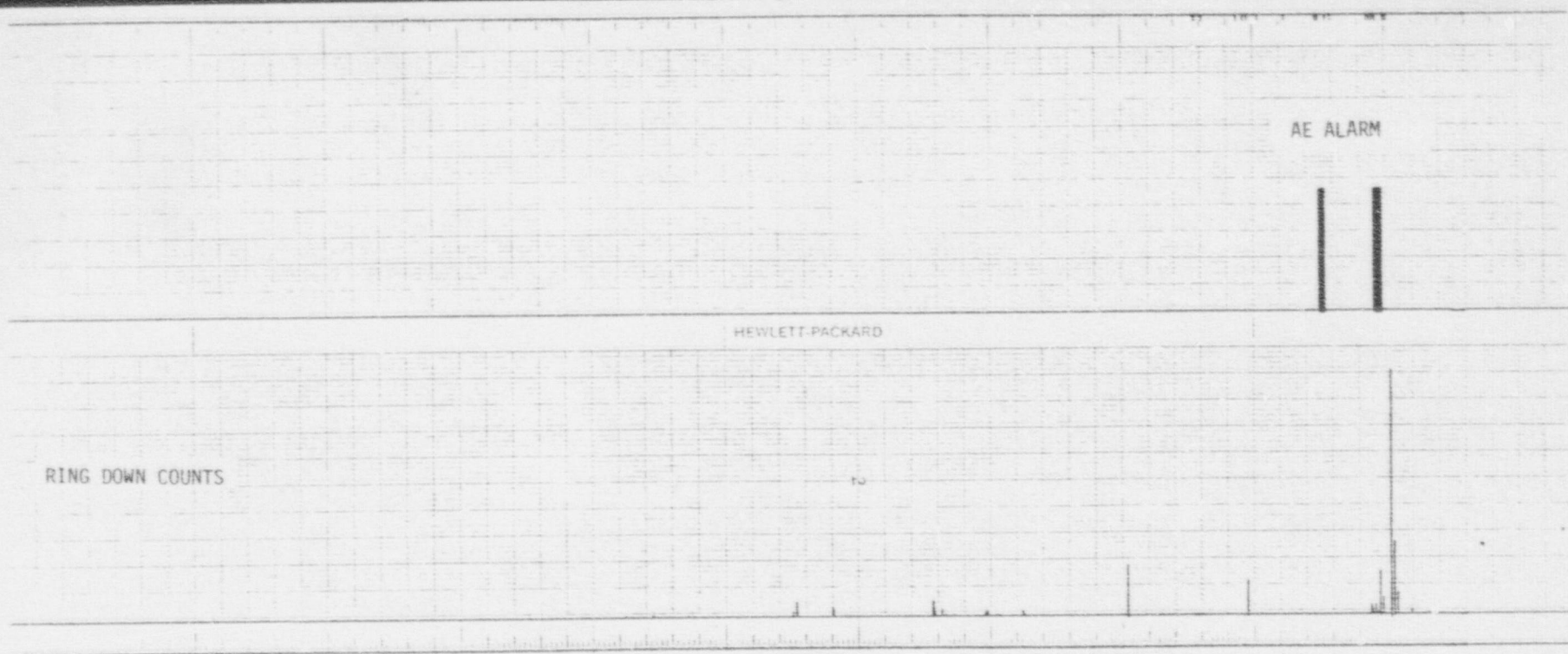
Figure 5-12 SHOWING AE STRIP CHART RECORD FOR B&W NOZZLE WELD CHART SPEED, 1 MM/SEC.
