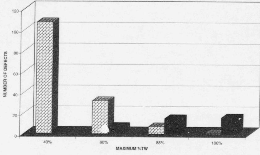
Pulled Tube Defects ARC (planned)
