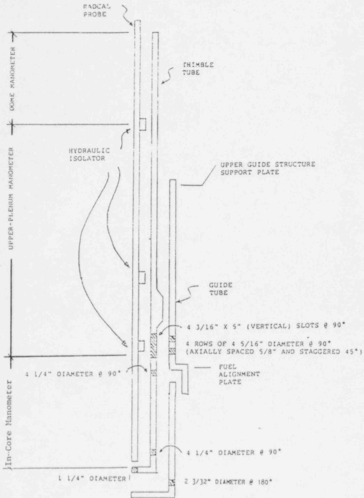
Figure 1 Schematic of the as-installed ANO-2 ICC system showing the axial locations of pertinent components.
