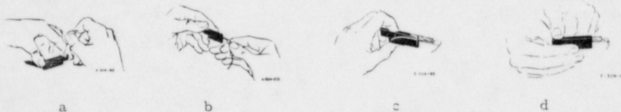
Fig. 7 - Installing Ink Capsule
