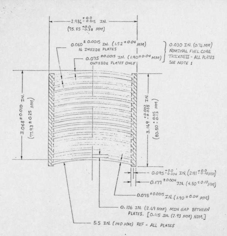
NOTE 1: MINIMUM CLADDING THICKNESS ON INSIDE PLATES 0.010 IN. (0.25 MM)
