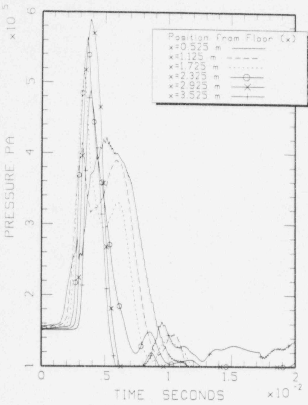
Figure 1 Local Explosion Pressure (3.89 m Pool Depth)
