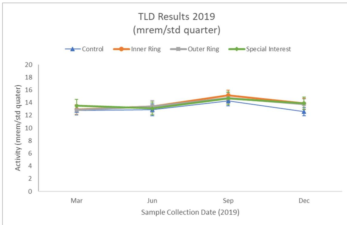
Figure 4.10.1-1: Graph of Direct Gamma Radiation Measurements
