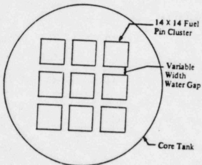
FIGURE 5 Typical Core Loading Diagram (Plan View)
