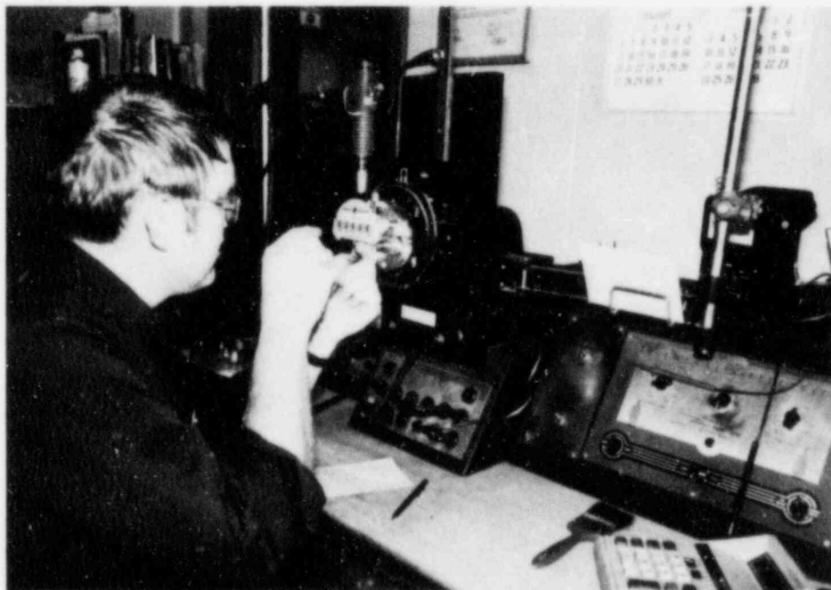
SERVICE RELIABILITY REINFORCED—Michael Brown completes precision testing of meters, a continuing requirement to assure meter accuracy.
