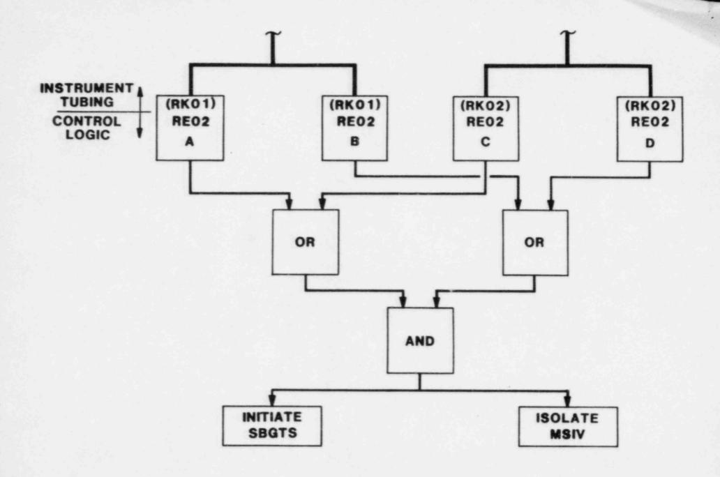
LO-LO WATER LEVEL TUBING & CONTROL LOGIC SET-UP
