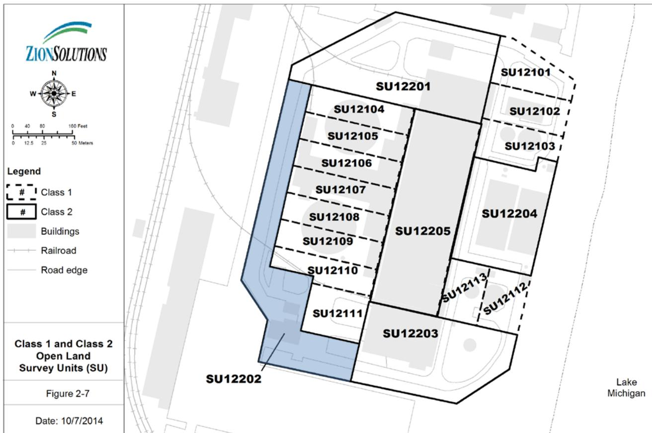
The HSA states that this area contained the Dry Active Waste (DAW) Storage Building, Illinois Department of Nuclear Safety (IDNS) Building, Meeting Trailers, Security Office and Gate House. Also, the area between the Fuel Handling Building (FHB) and Unit 2 Containment was a storage area for radioactive waste containers awaiting shipment. The HSA also notes that there were several instances of contaminated materials being found in the area. The most significant
