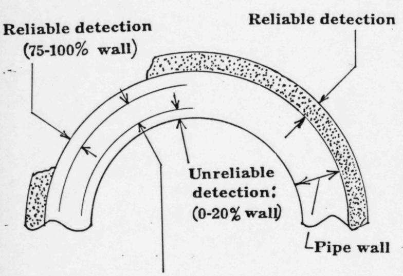
Insufficient data: (20-75%Through-wall)
