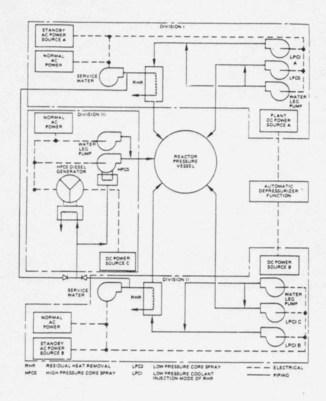
Figure 5.2 Emergency Cooling System Network for BWR/5
