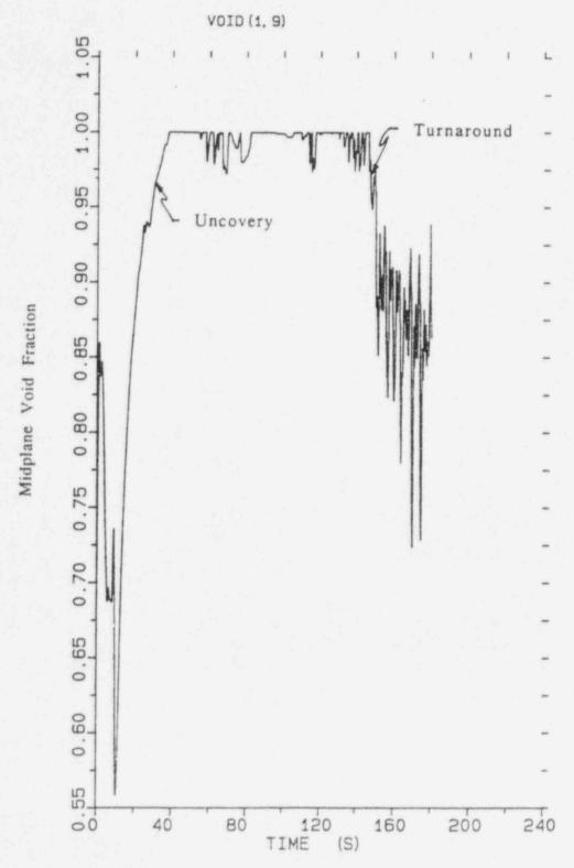
Figure 5.17 Hot Assembly Midplane Void Fraction
