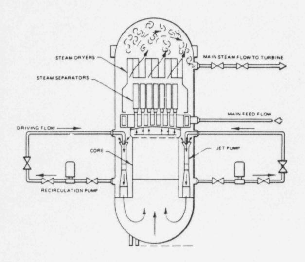
Figure 5.1 Jet Pump Boiling Water Reactor
