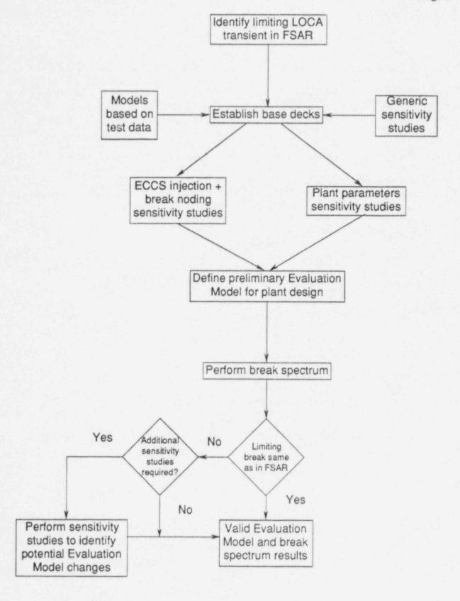
Figure 1.1 Method Used to Define LOCA Evaluation Model
