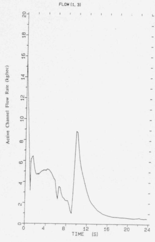
Figure 5.16 Hot Assembly Active Channel Inlet Flow
