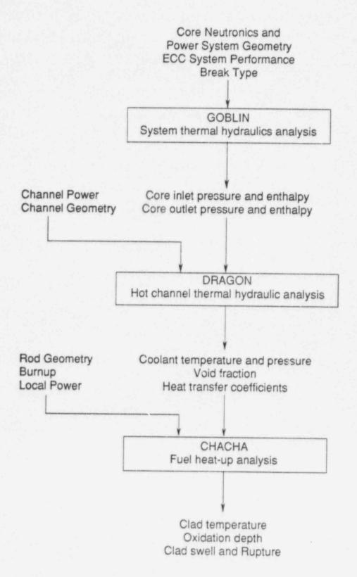
Figure 2.1 Flow of Information Between Computer Codes
