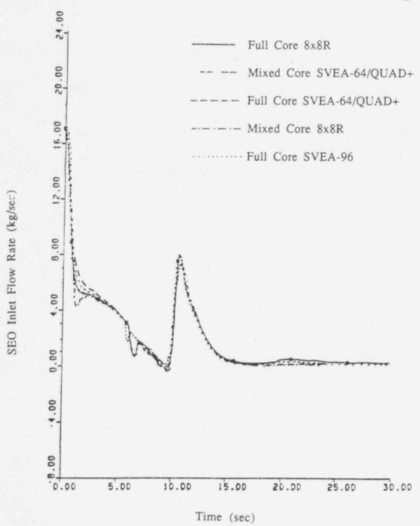
Figure 8.1 Side Entry Orifice Flow per Assembly for Each Fuel Type
