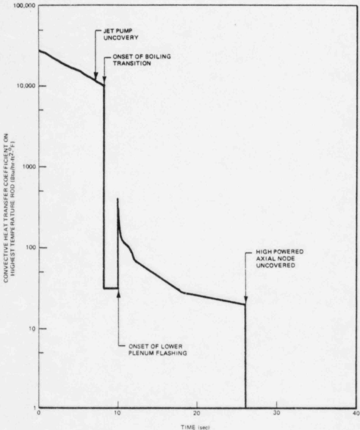
Figure 3a. Fuel Rod Convective Heat Transfer Coefficient During Blowdown at the High Power Axial Node Following a Maximum Recirculation Line Suction Break, LPCI Injection Valve Failure, Break Area = 4.2 ft<sup>2</sup>
