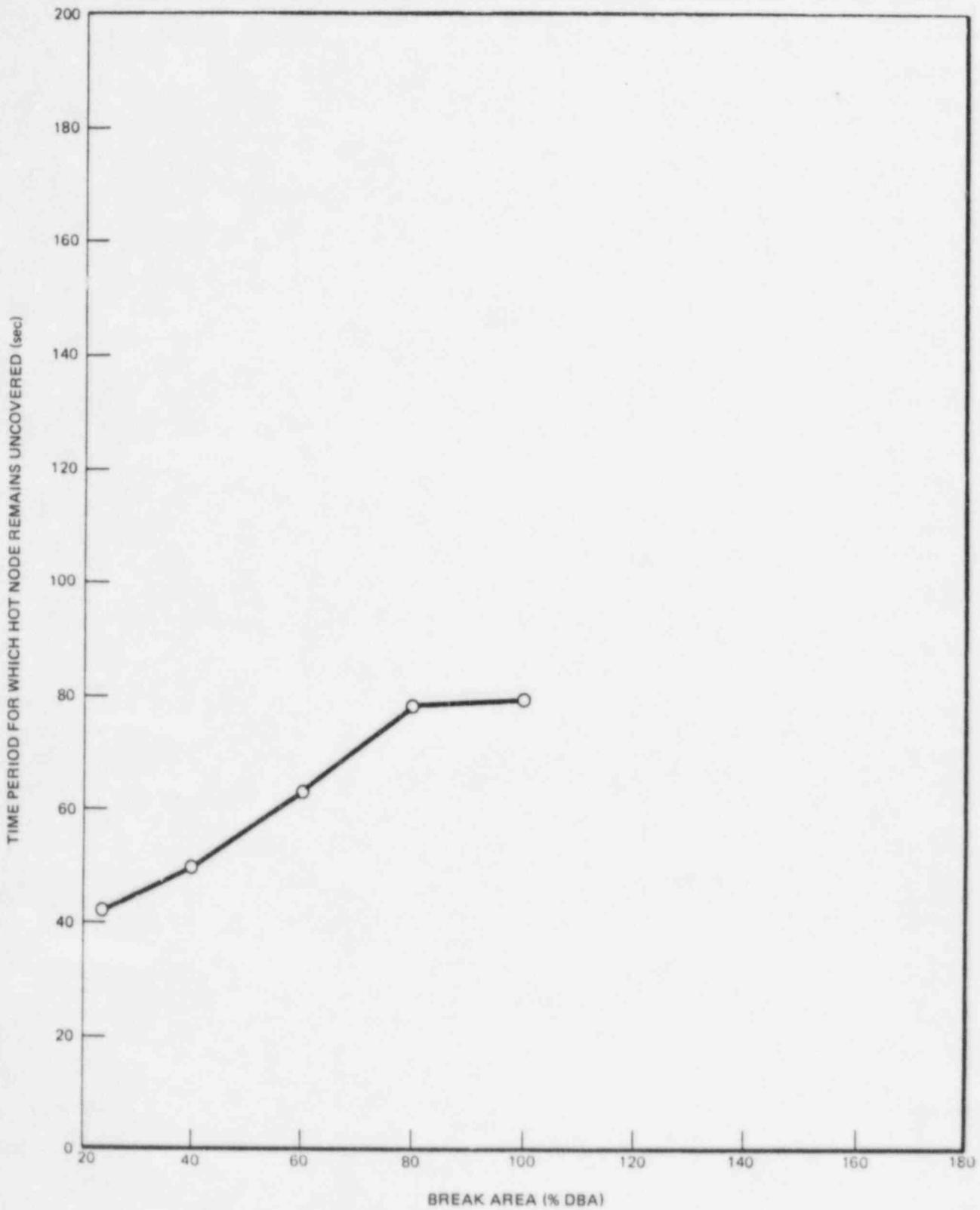
Figure 6b. Variation with Break Area of Time for Which Hot Node Remains Uncovered (Suction)
