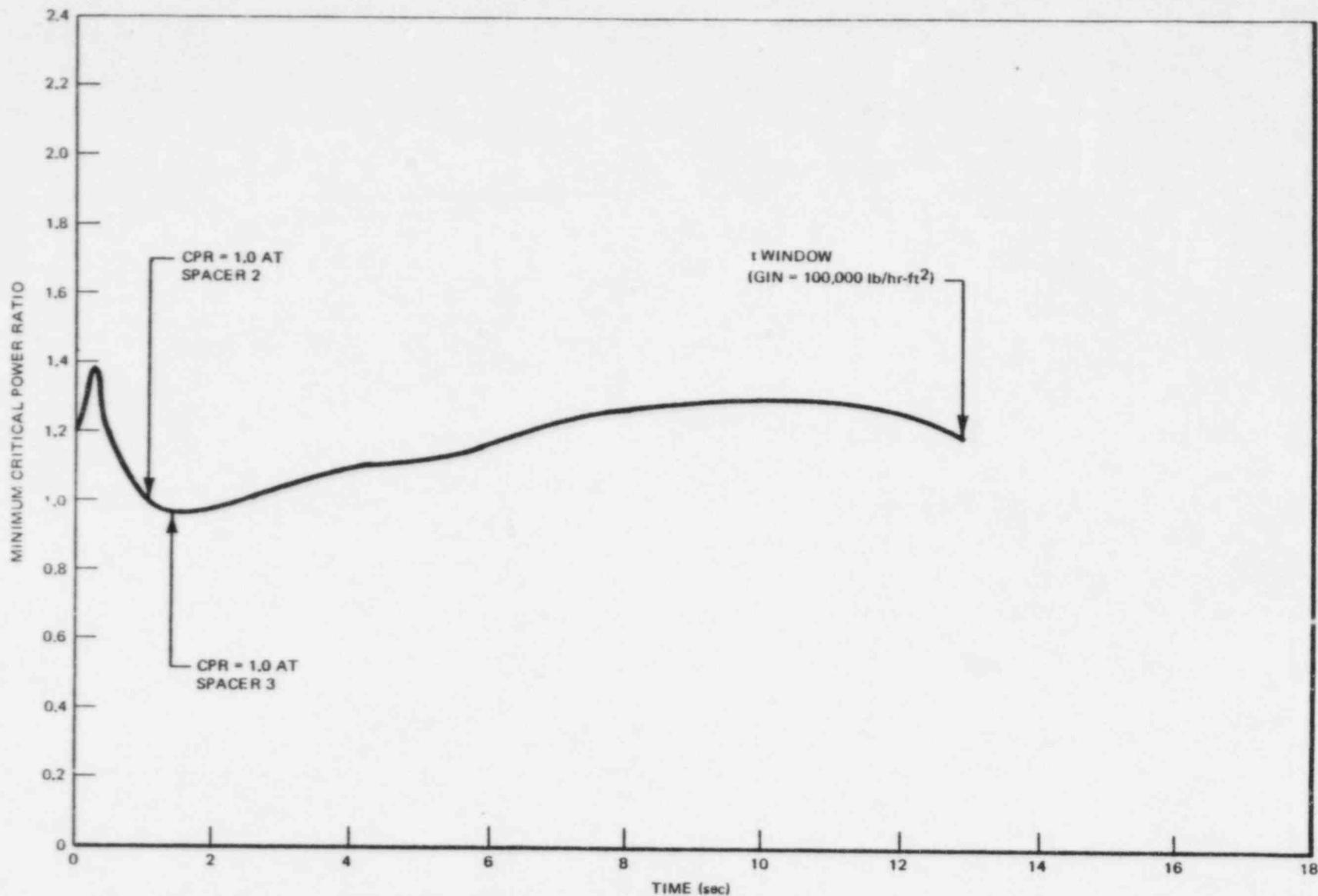
Figure 5b. Minimum Critical Power Ratio Following a Maximum Recirculation Line Discharge Break, Break Area = 1.9 ft<sup>2</sup>
