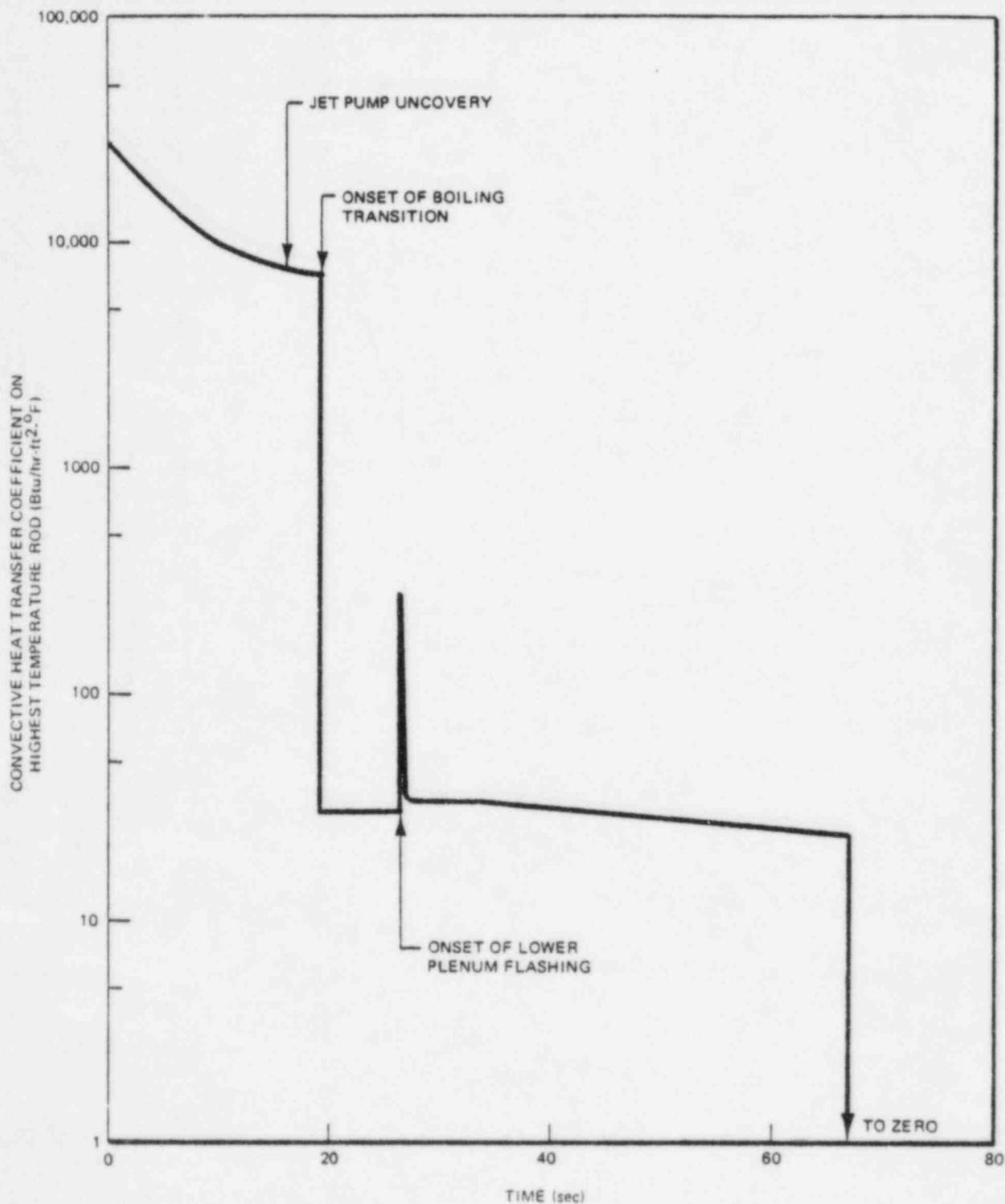
Figure 3c. Fuel Rod Convective Heat Transfer Coefficient During Blowdown at the High Power Axial Node Following a Recirculation Line Discharge Break, LPCI Injection Valve Failure, Break Area = 1.3 ft<sup>2</sup> (66% DBA)
