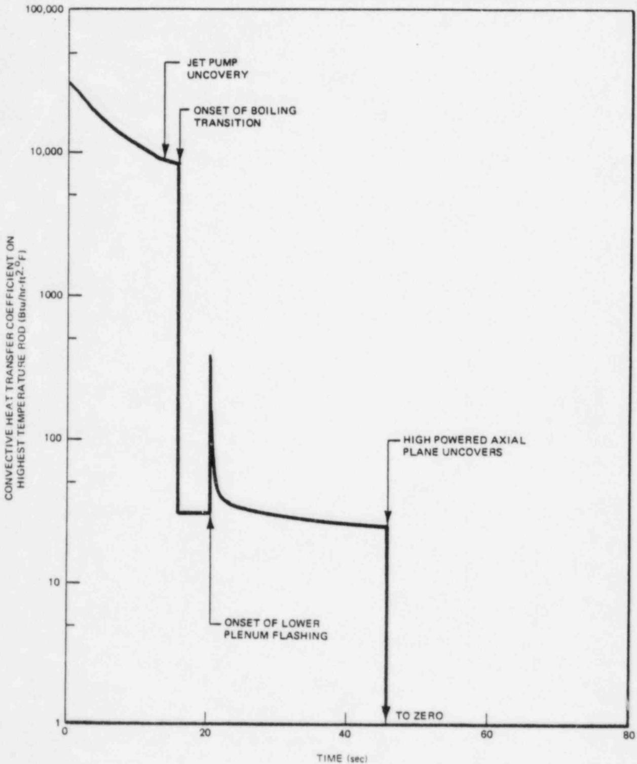
Figure 3b. Fuel Rod Convective Heat Transfer Coefficient During Blowdown at the High Power Axial Node Following a Maximum Recirculation Line Discharge Break, LPCI Injection Valve Failure, Break Area = 1.9 ft<sup>2</sup>
