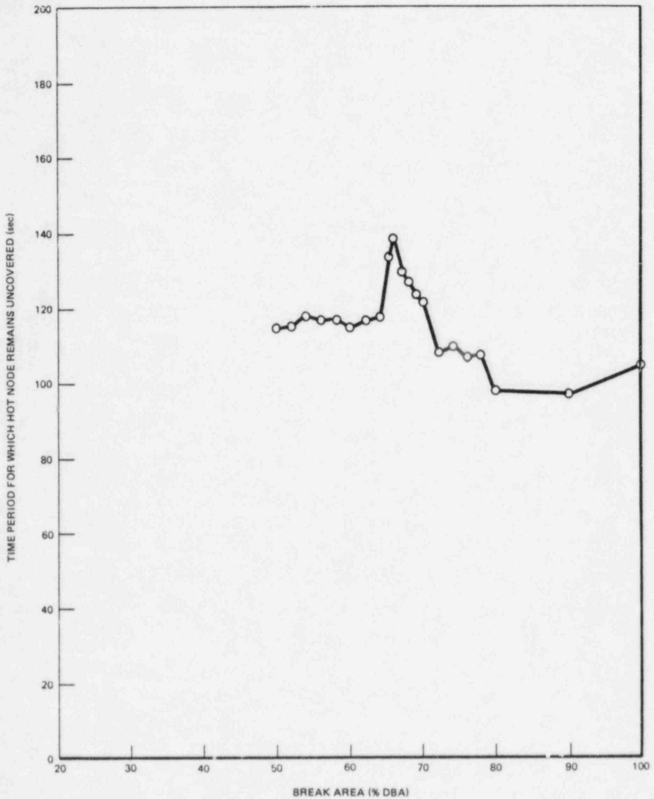
Figure 6a. Variation With Break Area of Time for Which Hot Node Remains Uncovered (Discharge)
