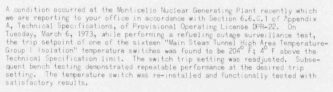
The sixteen temperature switches are connected in a "one of two twice" logic scheme at four locations in the steam tunnel. Redundant temperature switches at the same location would have provided the desired trip action at the desired trip setting, had a steam line break occurred during reactor operation.
