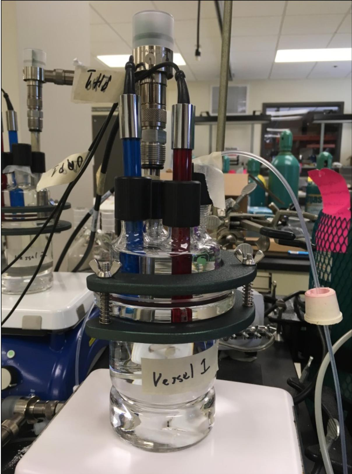
**Figure 2-1. 4-port reaction vessel used for grout and cementitious material water-conditioning tests**
