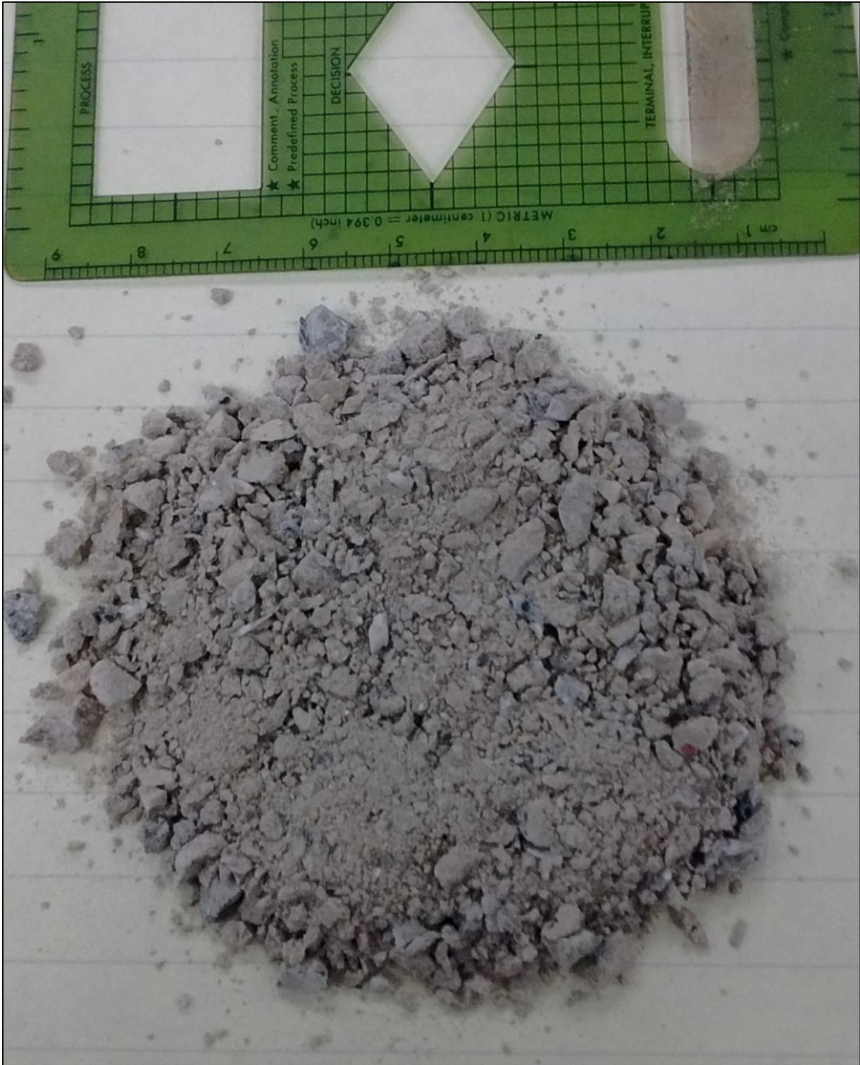
**Figure 3-1. Photograph of pulverized reducing tank grout used in pulverized-grout water-conditioning tests**
