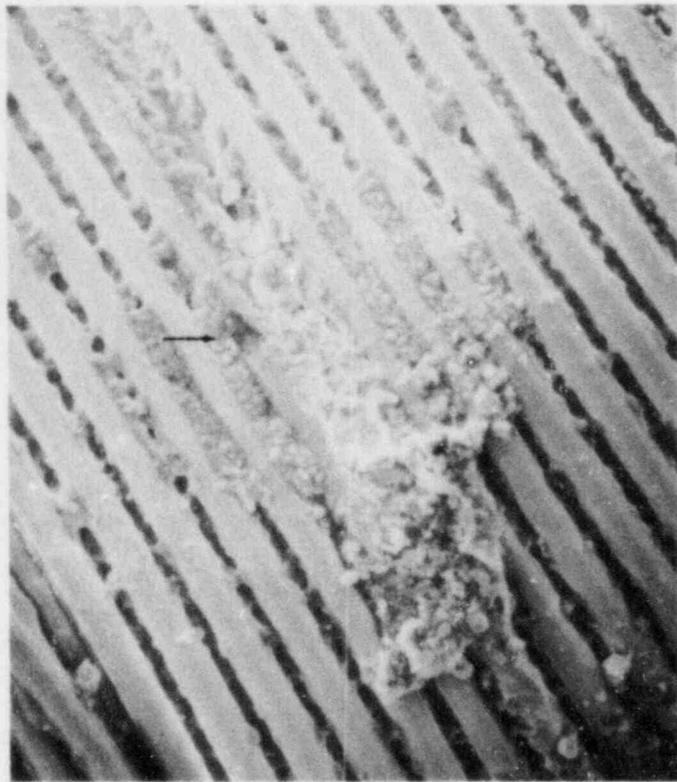
Figure 9-10 SEM of Foreign Material Found Near Wire Break Shown in Figure 9-5 (150x). Partially corroded winding is indicated by arrow.
