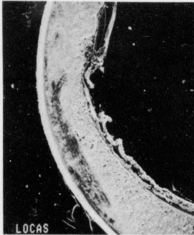
Figure 9-1 Scanning Electron Micrograph (SEM) of C-Ring (20x)
