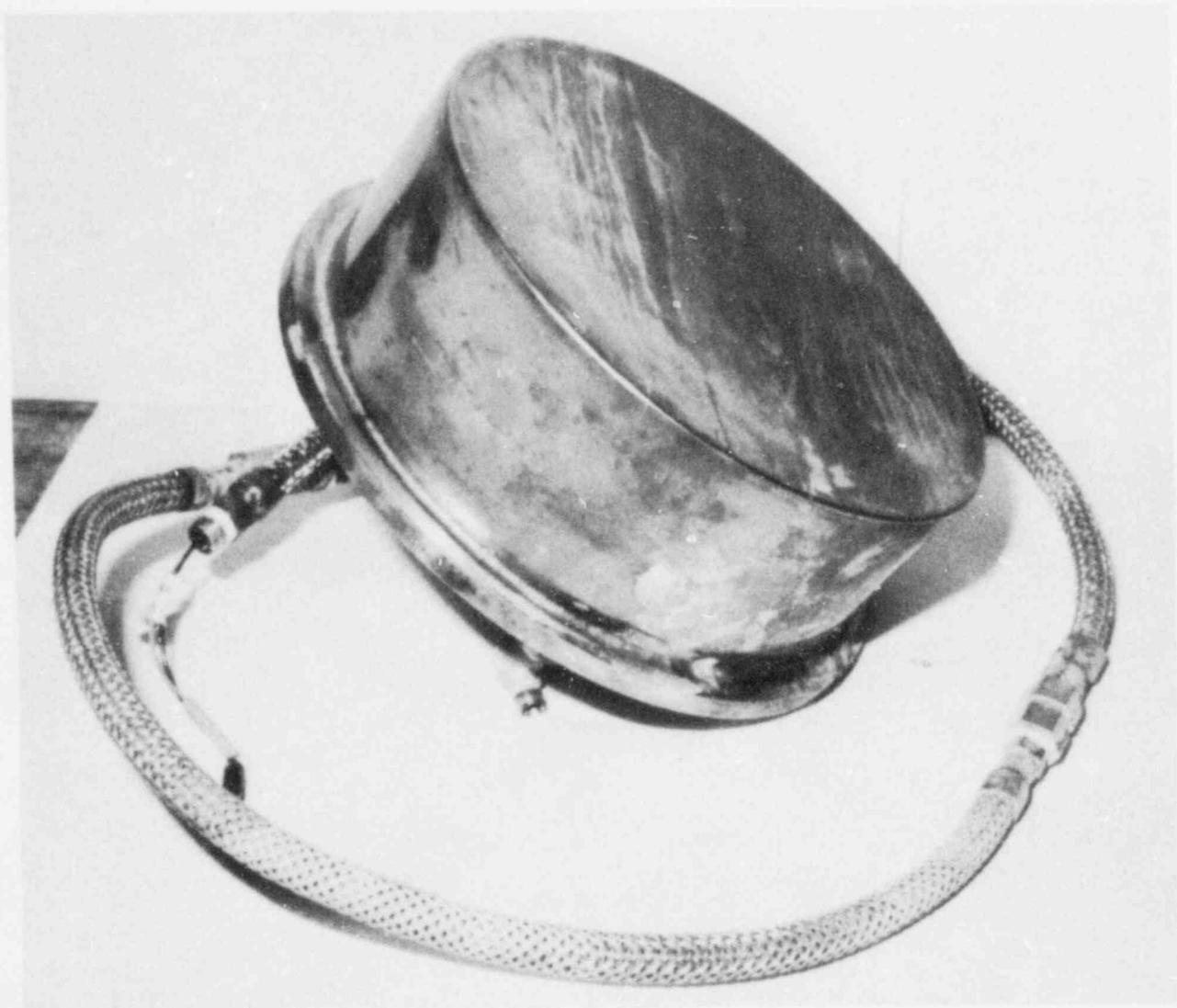
Figure 3-1 Transmitter T4 in Stainless Steel Enclosure
