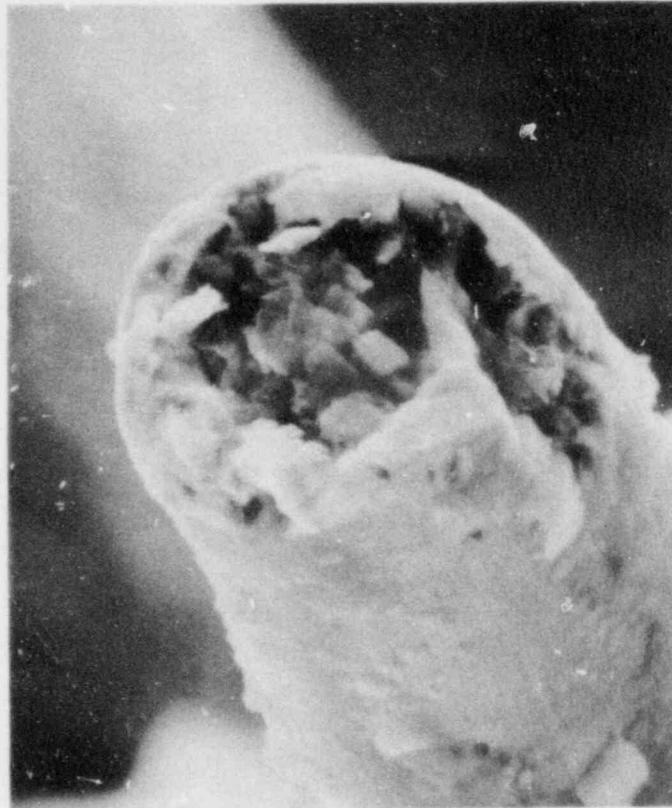
Figure 9-6 SEM of the Wire Cross Section From the Test-Induced Break Occurring in the Active Portion of the Potentiometer Resistive Element (2000x)
