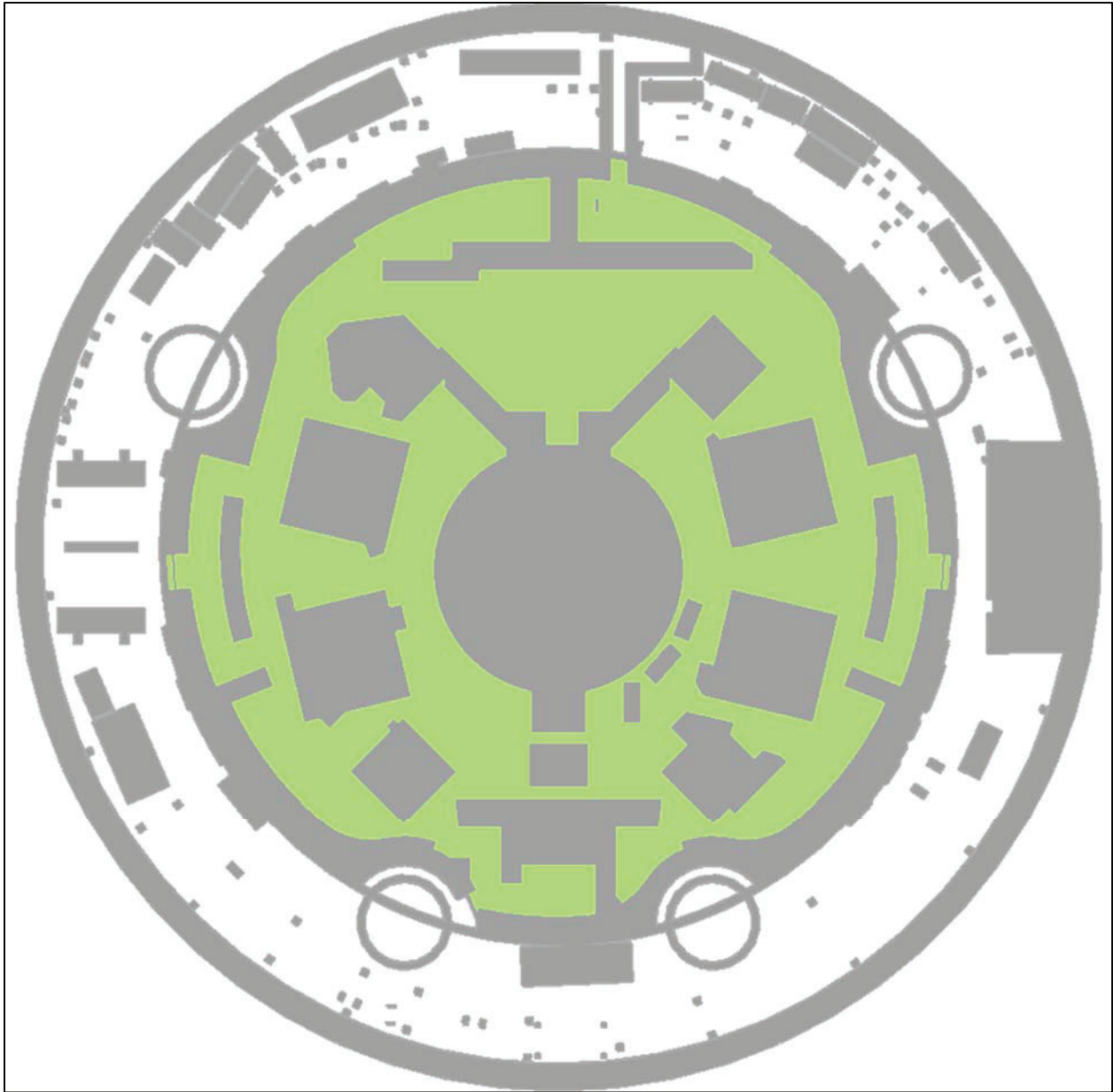
Figure 3.e.1-3: Distribution of Small Debris Blown into Lower Containment at Start of Recirculation
