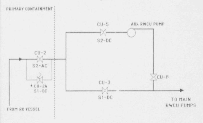
\*CU-2A power supply changed from S1-DC to S2-DC during 1991 refueling outage
