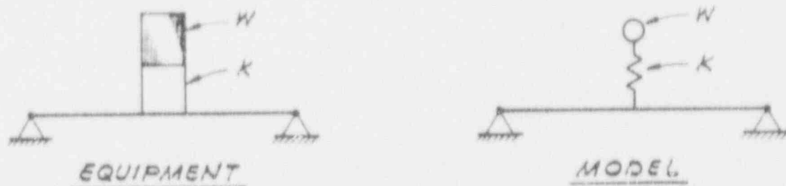
FIG. C-3 EQUIPMENT SUPPORTED ON FLEXIBLE BEAM OR SLAB
