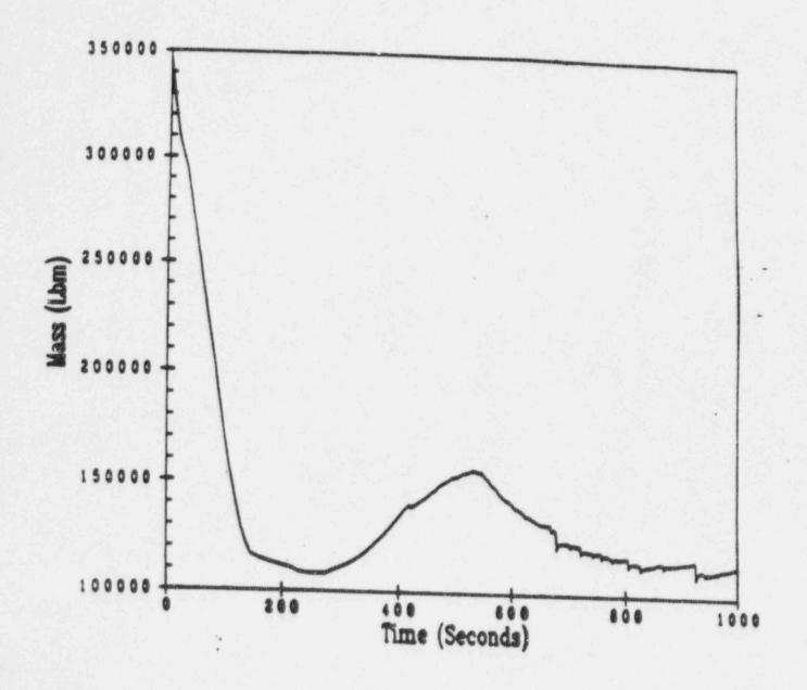
Figure 440.328-2 Double Ended DVI Line Break, Reactor System Coolant Inventory
