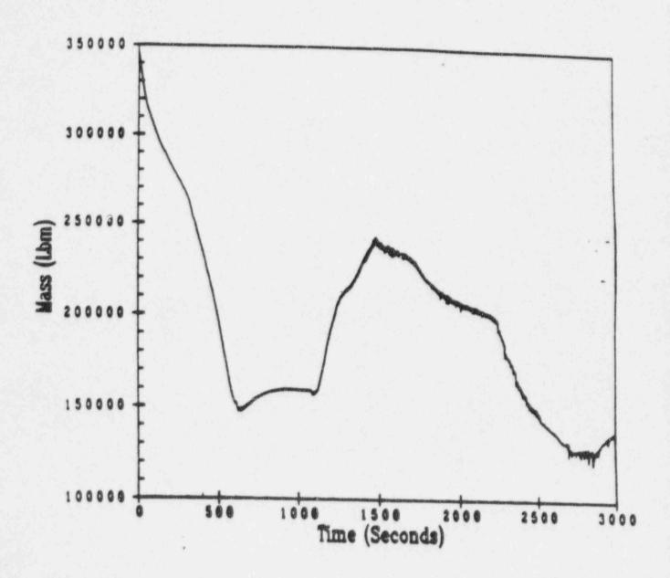
Figure 440.328-3 Two Inch Cold Leg Break Is Salance Line Loop, Reactor System Coolant Inventory
