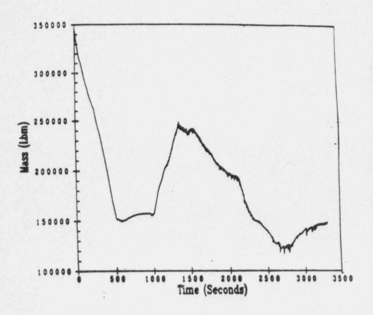
Figure 440.328-4 Two Inch Cold Leg Break in PRHR Loop, Reactor System Coolant inventory
