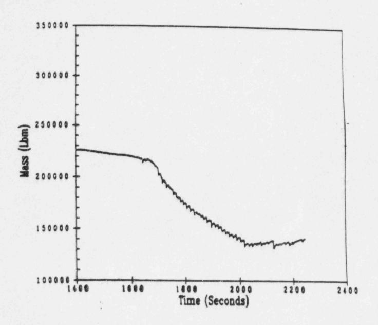
Figure 440.328-5 Inadvertent ADS Actuation, Reactor System Coolant Inventory
