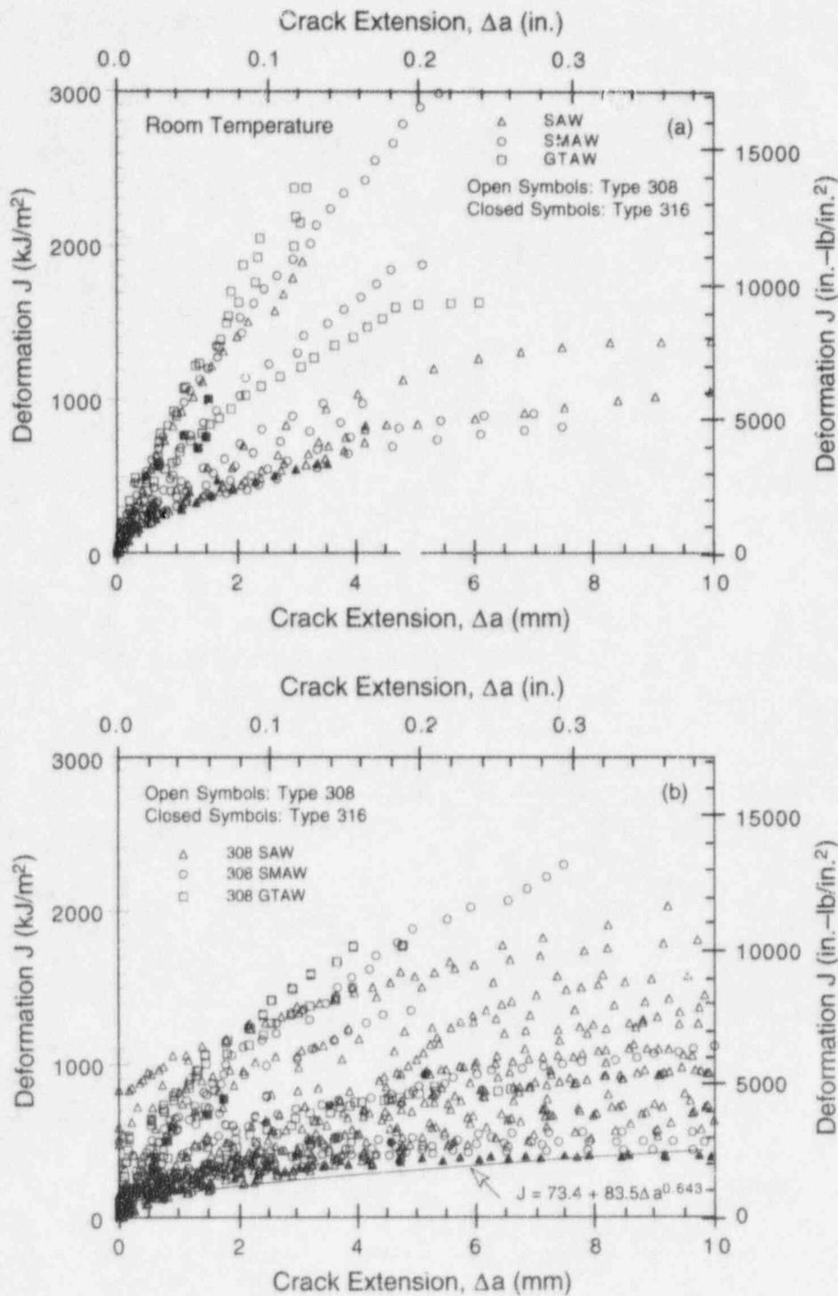
Figure 15. Fracture toughness  $J$ - $R$  curves for stainless steel welds at (a) room temperature and (b) 288-427°C. Solid line represents lower-bound curve.
