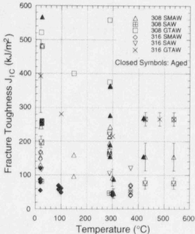
Figure 17. Fracture toughness  $J_{IC}$  for unaged and aged stainless steel welds
