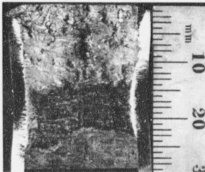
Figure A-4. Fracture surface of aged weld metal PWCE tested at 25°C
