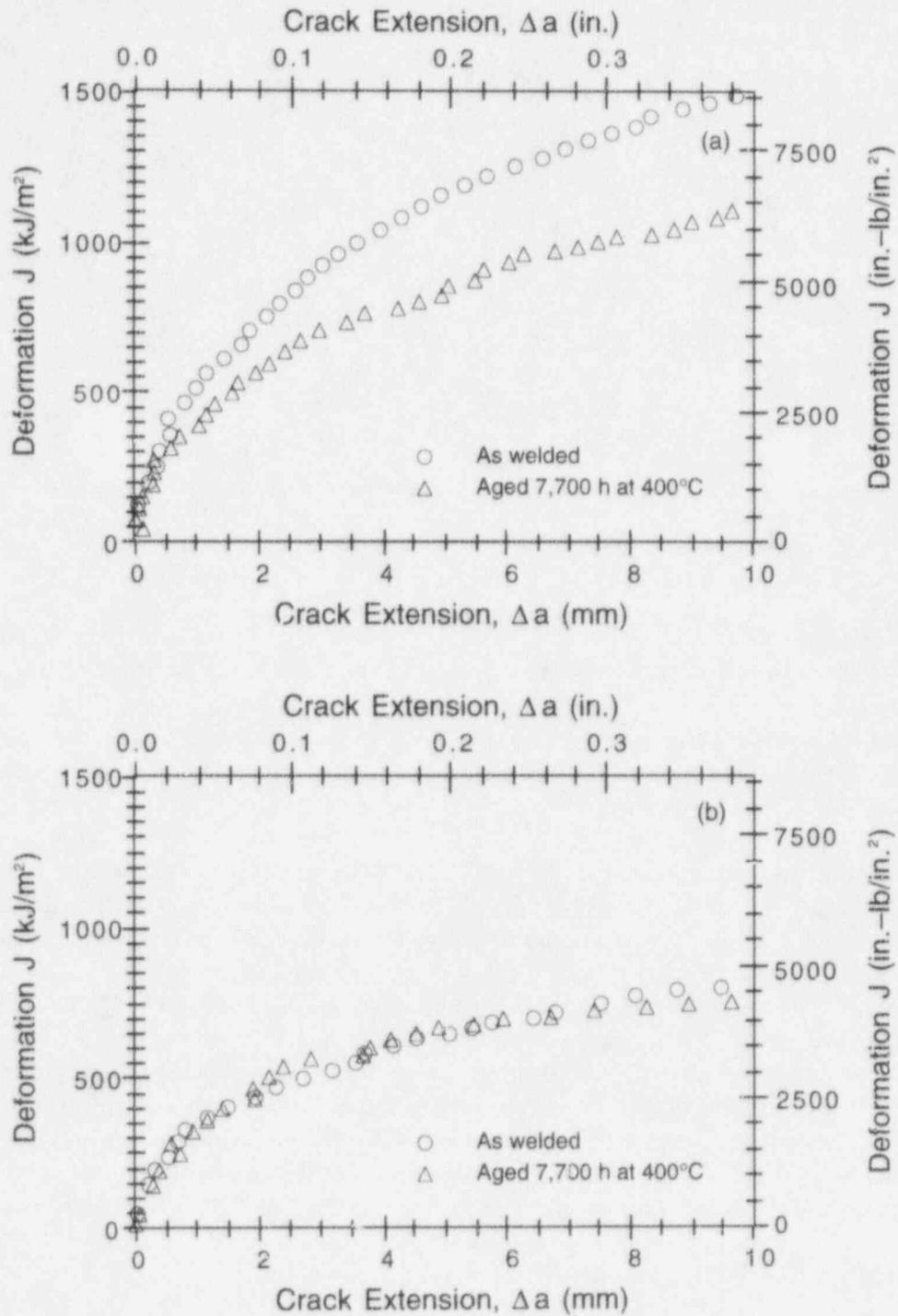
Figure 13. Fracture toughness J-R curve for PWWO weld at (a) room temperature and (b) 290°C
