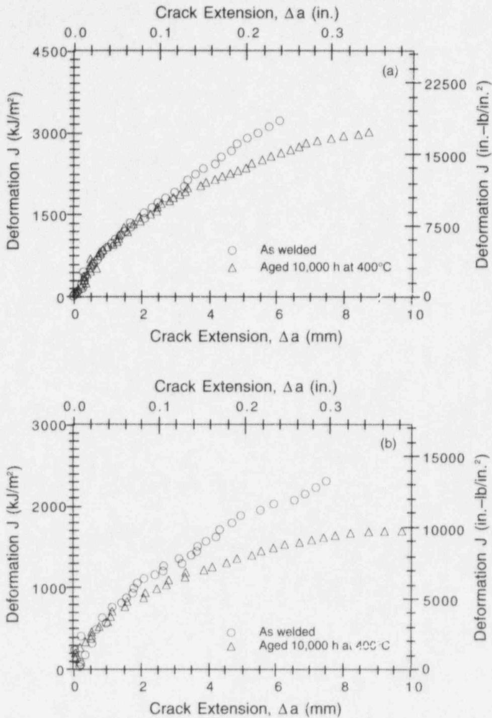
Figure 12. Fracture toughness J-R curve for PWCE weld at (a) room temperature and (b) 290°C
