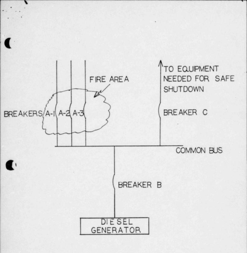
GURE IS MULTIPLE HIGH IMPEDENCE FAULTS
