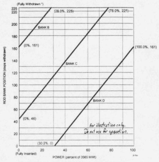
\* Fully withdrawn shall be the condition where control rods are at a position within the interval ≥225 and ≤231 steps withdrawn
