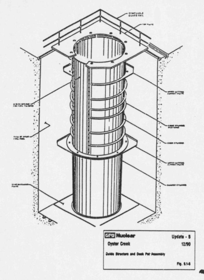
Figure 2 - Cask Drop Protection System (showing steel guide cylinder and dashpot)
