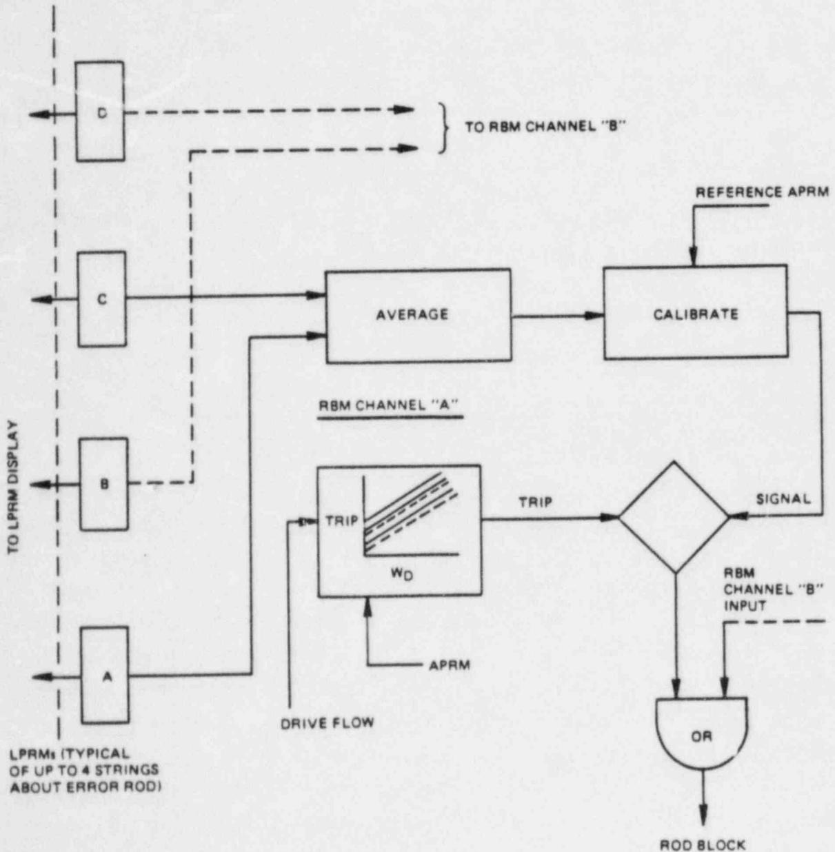
Figure 4-1. Conceptual Illustration of Current DAEC Flow Dependent RBM System with AC/BD LPRM Assignment
