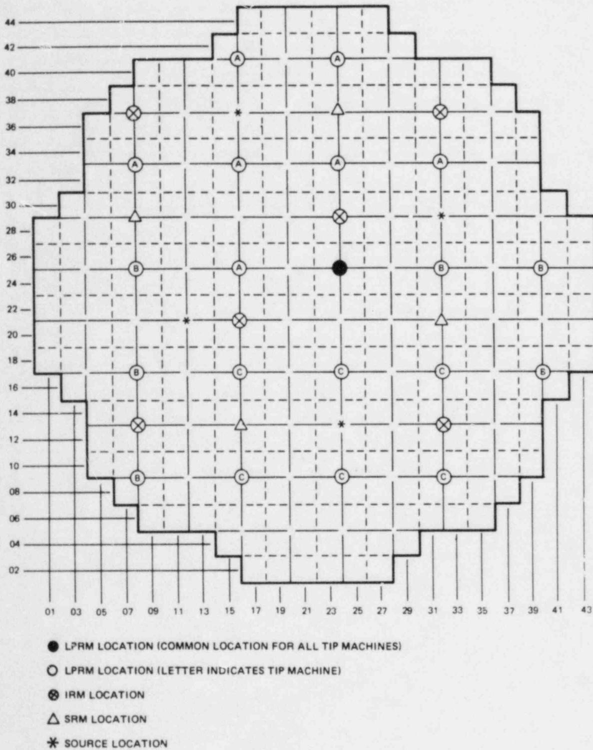
Figure 4-11. DAEC Neutron Monitoring System
