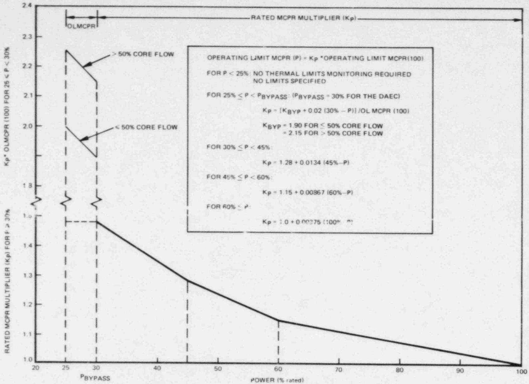
Figure 3-2. Power Dependent MCPR for the DAEC ( $K_p$ )
