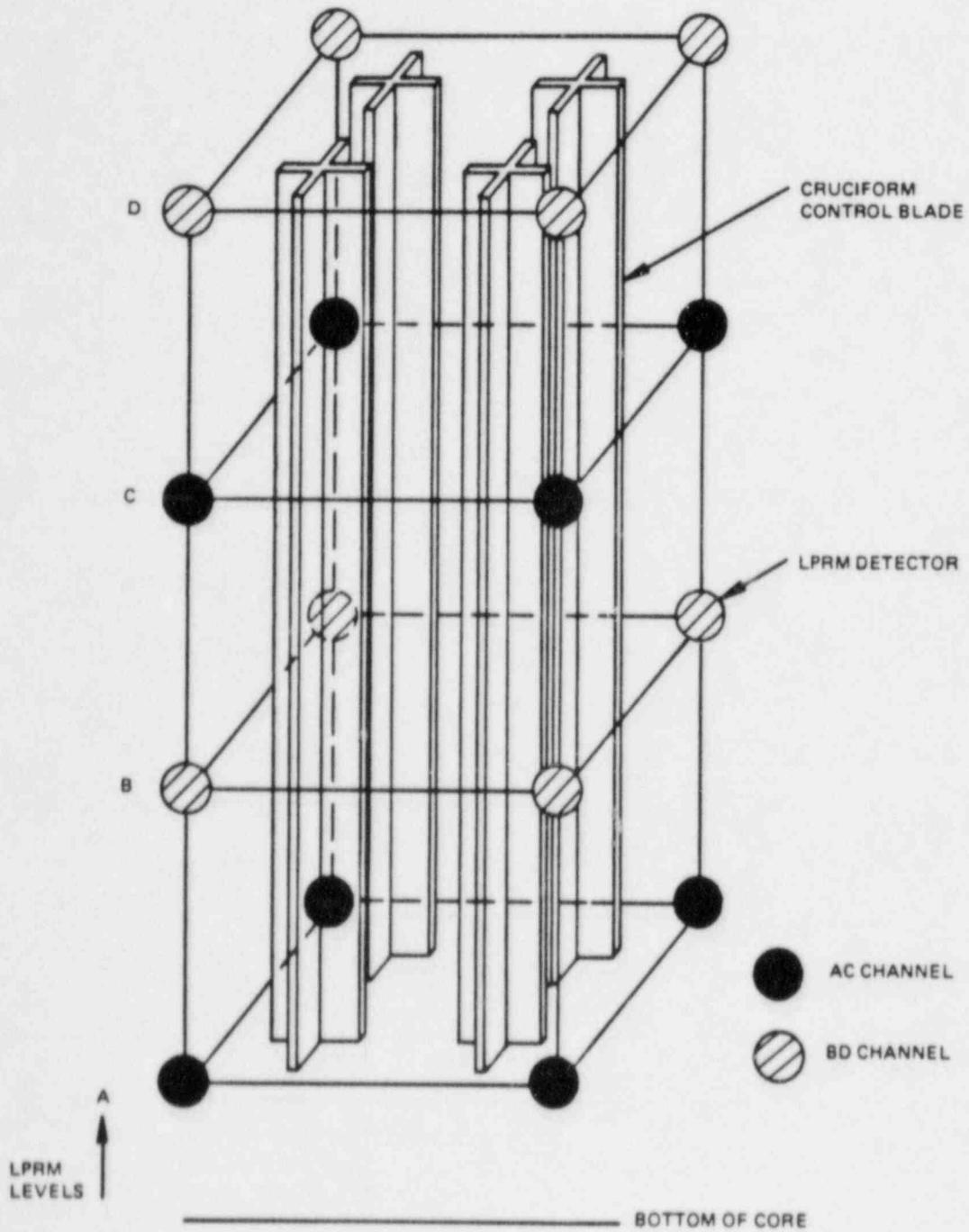
Figure 4-4. DAEC RBM Current AC/BD LPRM Assignment
