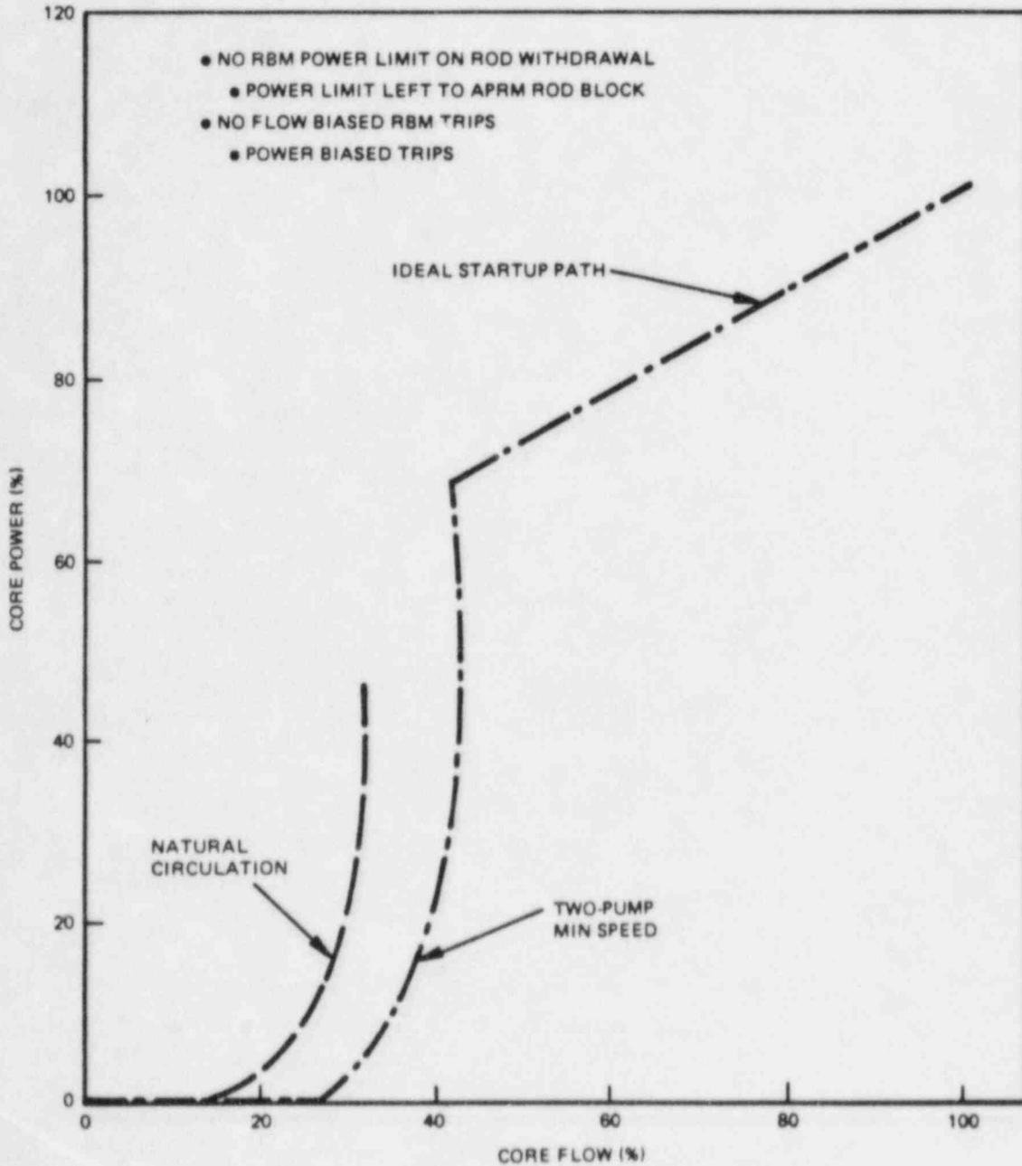
Figure 4-7. New DAEC RBM System Core Power Limit
