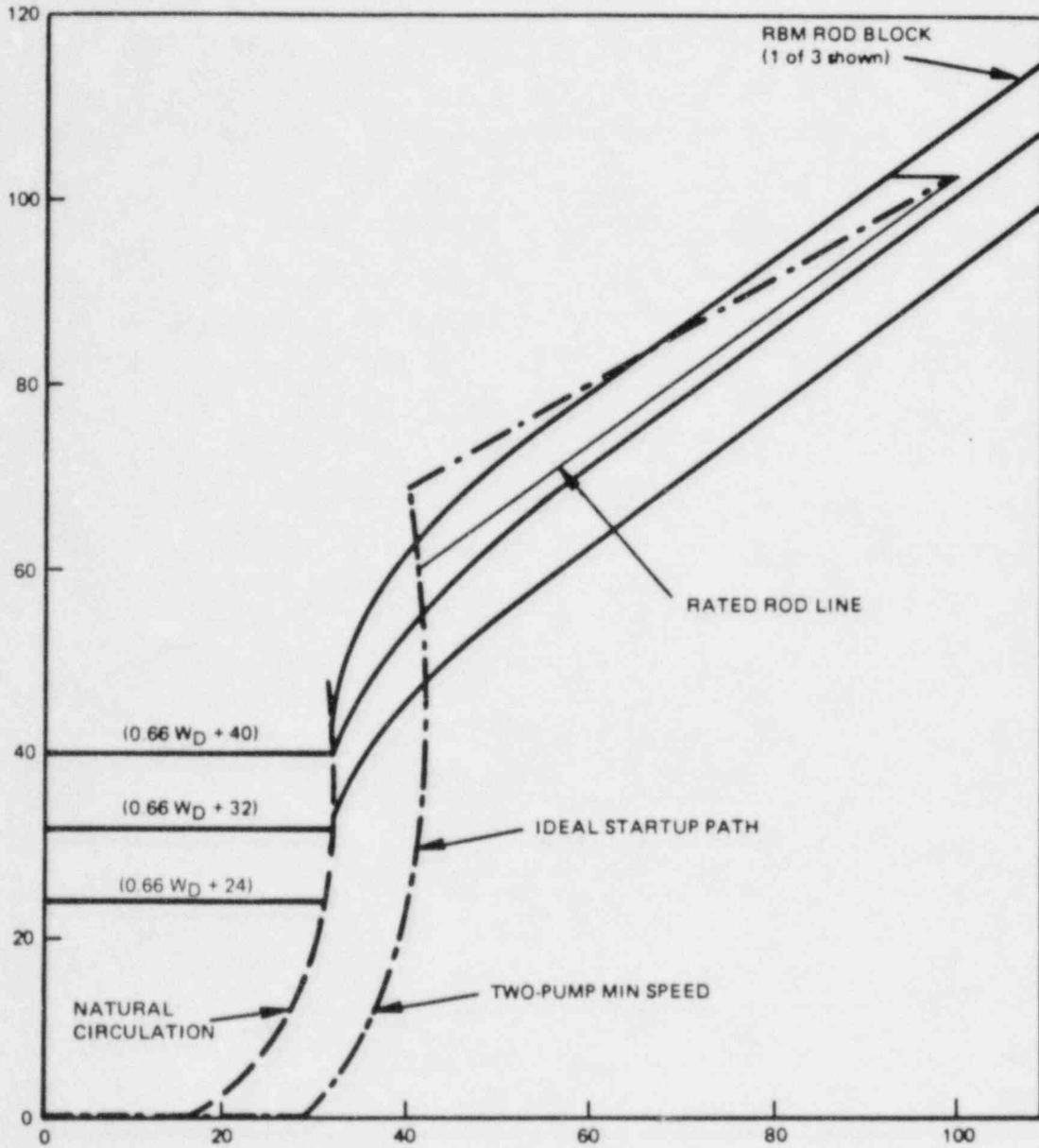
Figure 4-2. Current RBM Limits (Typical for 106 Setpoint)
