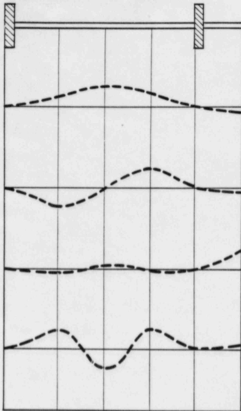
UGS GUIDE TUBE NATURAL FREQUENCIES & MODESHAPES FIGURE 2.2-12
