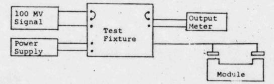
a. Set signal generator to output a 10 Hz square wave,
