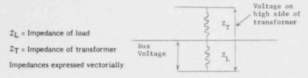
Bus Voltage =  $\frac{Z_L}{Z_L+Z_T}$  Voltage on high side of transformer.
