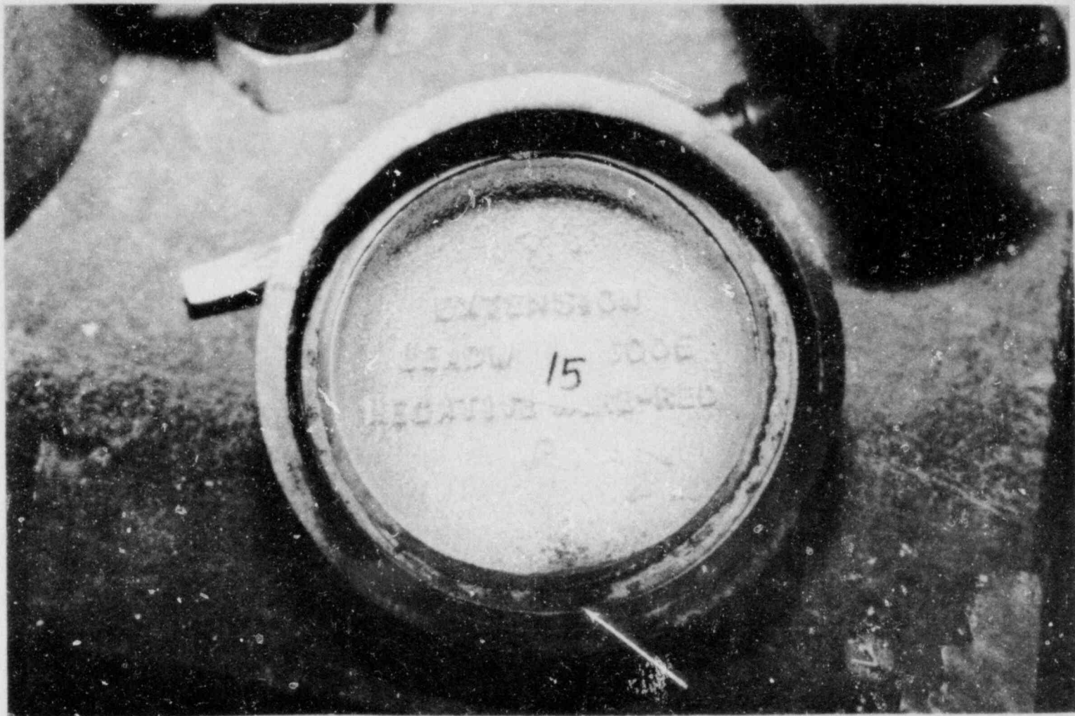
Figure 32. RTD No. 4, showing discoloration of cap seal.
