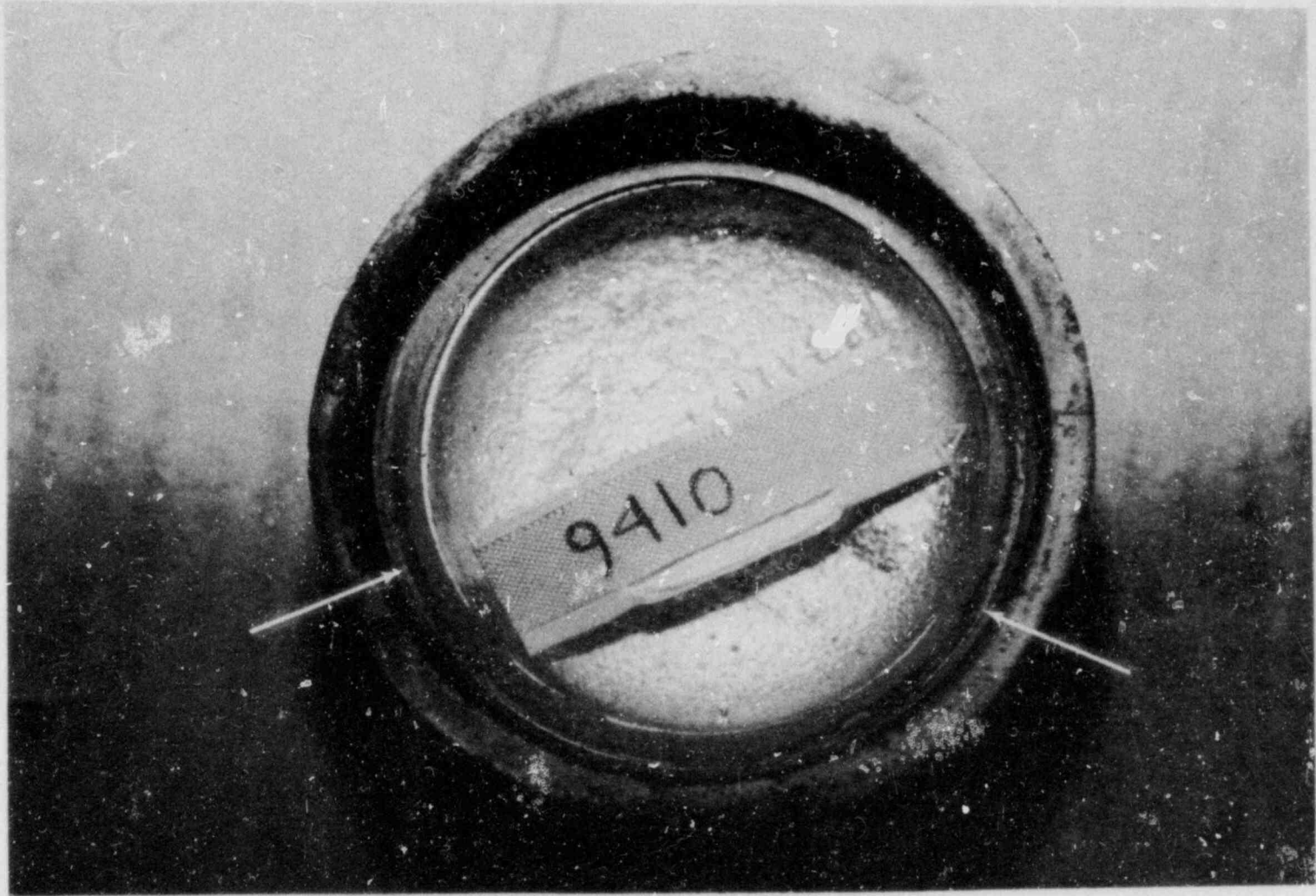
Figure 31. RTD No. 2, showing discoloration of cap seal.
