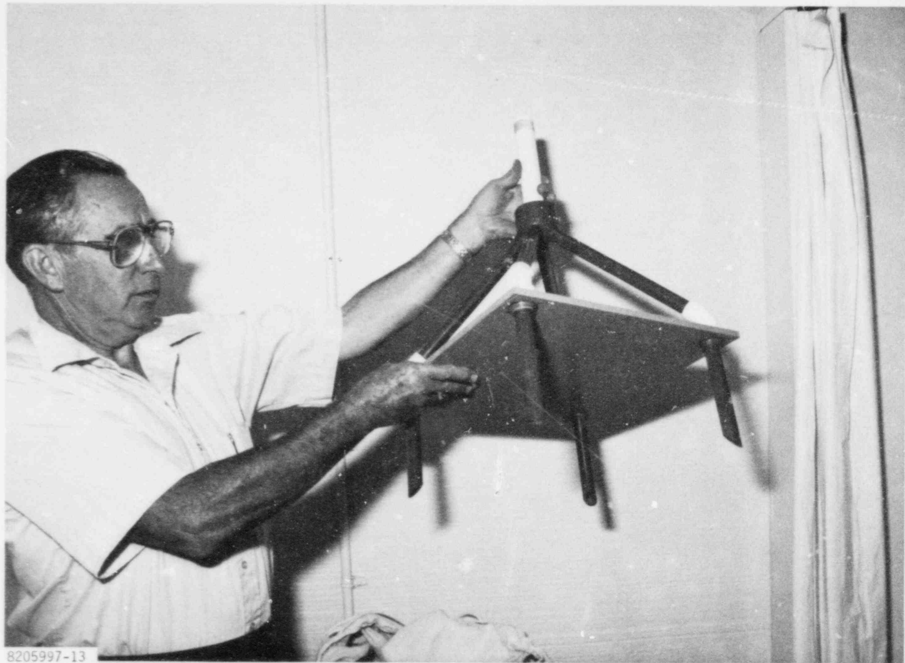
FIGURE 3-19. Header Used to Divide the Slurry Stream
