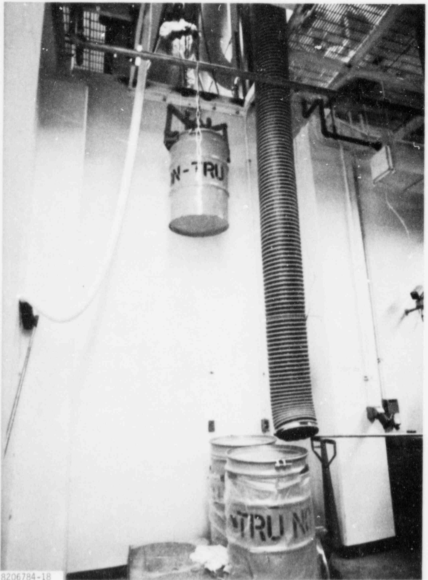
FIGURE 3-24. Remote Clamping and Hoisting System
