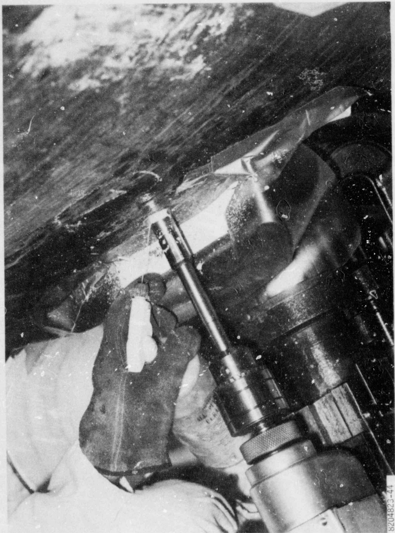
FIGURE 2-1. Core Drilling to Obtain Samples of the Interior Channel Head Surfaces
