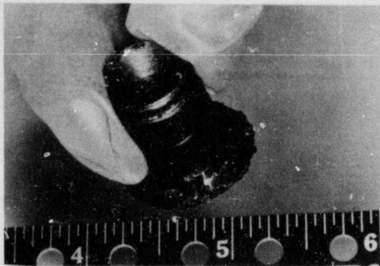
FIGURE 7-6. Core Specimen Removed From the Hot Leg Channel Head Wall Before Decontamination
