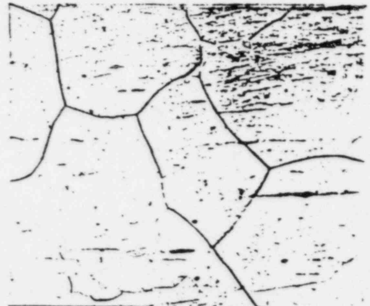
FIGURE 10A PHOTOMICROGRAPH OF CROSS SECTION OF WELD #8 AFTER ETCHING.
