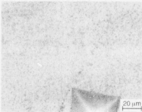
(a) Electroetched in 10% phosphoric acid solution
