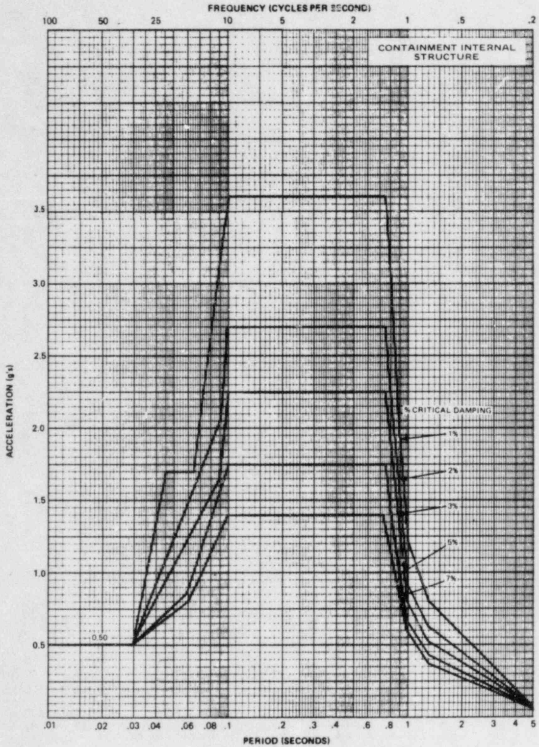
Figure B-9 SAFE SHUTDOWN EARTHQUAKE HORIZ. ACCEL. RESPONSE SPECTRA EL. 261 FT. 0 IN.
