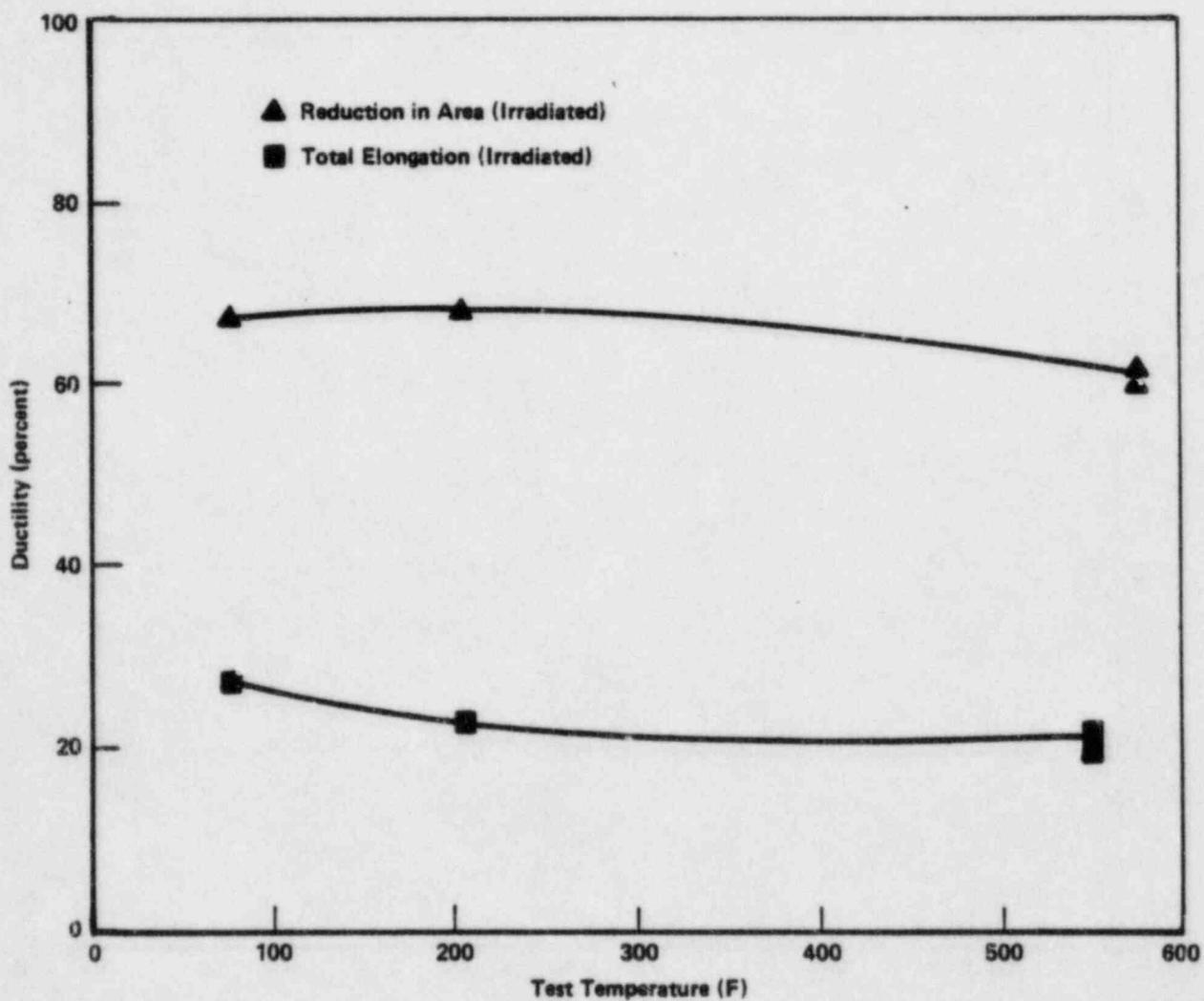
FIGURE 25. BASE METAL TOTAL ELONGATION AND REDUCTION IN AREA VERSUS TEST TEMPERATURE FOR THE IRRADIATED TENSILE SPECIMENS FROM THE MONTICELLO 30 DEGREE SURVEILLANCE CAPSULE
