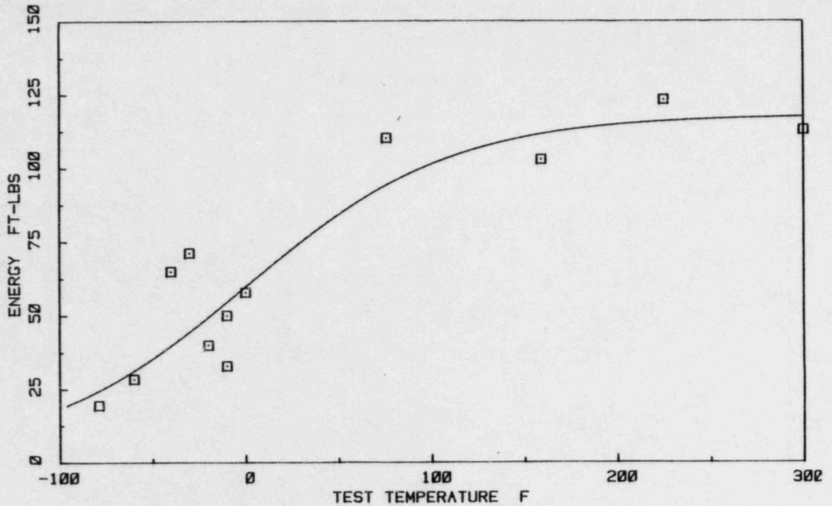
FIGURE 18. CHARPY V-NOTCH IMPACT ENERGY VERSUS TEST TEMPERATURE FOR THE IRRADIATED HAZ METAL SPECIMENS FROM THE MONTICELLO 30 DEGREE SURVEILLANCE CAPSULE
