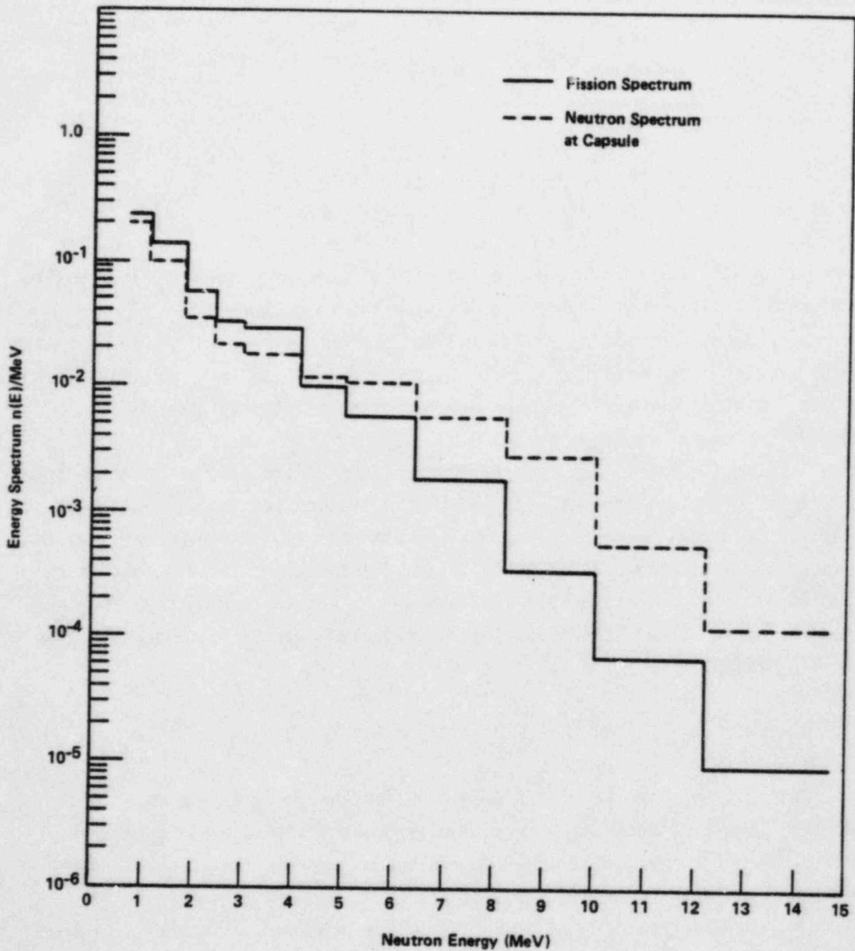
FIGURE 9. COMPARISON OF DOT SPECTRUM WITH FISSION SPECTRUM AT THE MONTICELLO 30 DEGREE SURVEILLANCE CAPSULE
