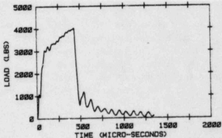
FIGURE A-4. INSTRUMENTED CHARPY IMPACT DATA FOR IRRADIATED BASE METAL SPECIMENS FROM THE MONTICELLO 30 DEGREE SURVEILLANCE CAPSULE
