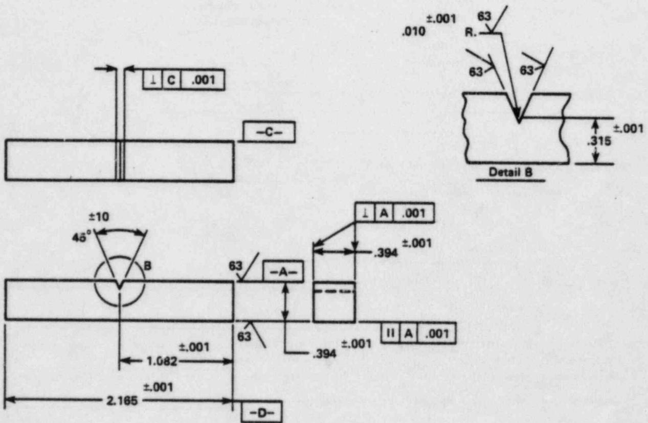
FIGURE 2. TYPICAL CHARPY V-NOTCH IMPACT SPECIMEN
