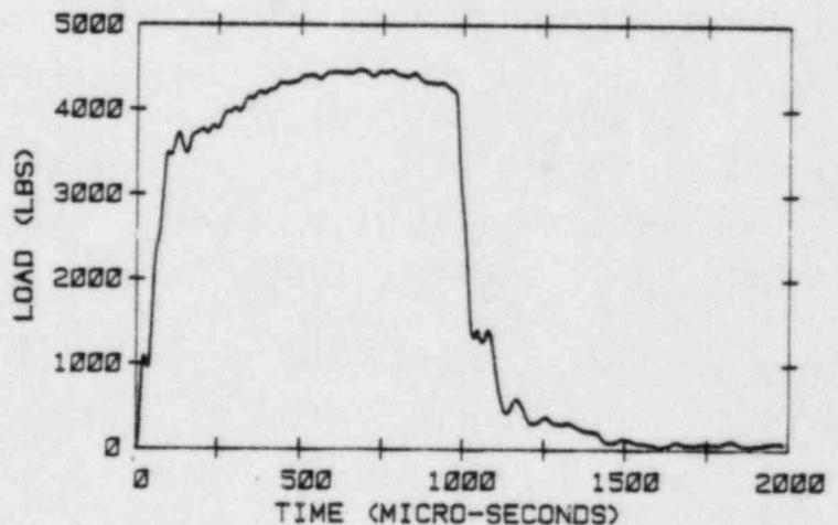
FIGURE A-5. INSTRUMENTED CHARPY IMPACT DATA FOR IRRADIATED WELD METAL SPECIMENS FROM THE MONTICELLO 30 DEGREE SURVEILLANCE CAPSULE
