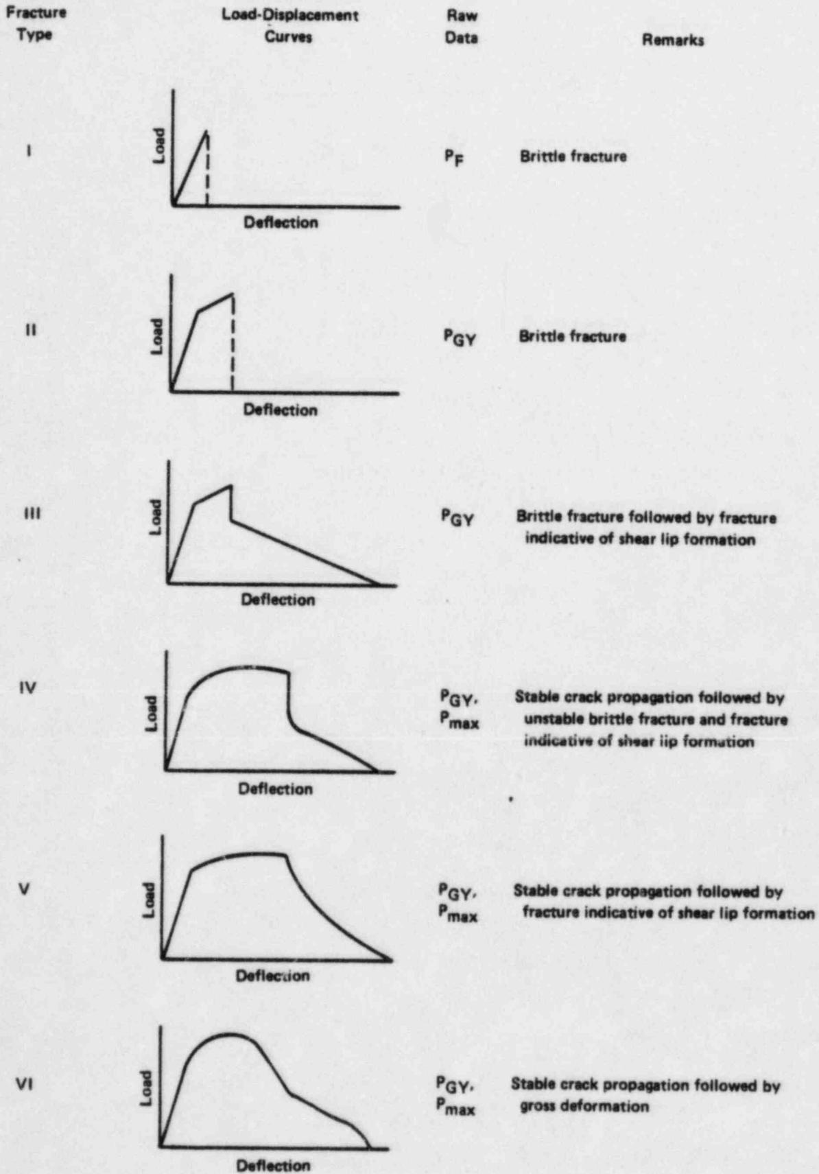
FIGURE A-7. THE SIX TYPES OF FRACTURES FOR NOTCHED BAR BENDING
