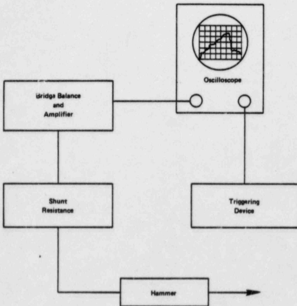
FIGURE A-3. DIAGRAM OF INSTRUMENTATION ASSOCIATED WITH INSTRUMENTED CHARPY EXAMINATION
