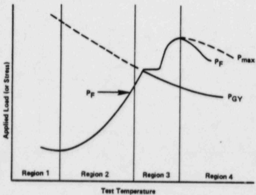
FIGURE A-2. GRAPHICAL ANALYSIS OF CHARPY IMPACT DATA
