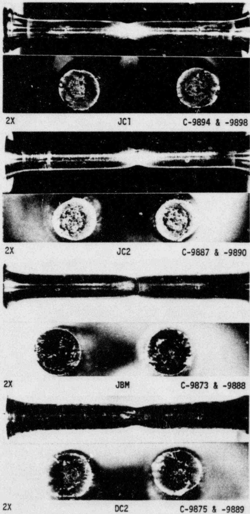
FIGURE 26. POSTTEST PHOTOGRAPHS OF THE IRRADIATED BASE METAL TENSILE SPECIMENS SHOWING BOTH THE REDUCED AREAS AND FRACTURE SURFACES (MONTICELLO 30 DEGREE SURVEILLANCE CAPSULE)
