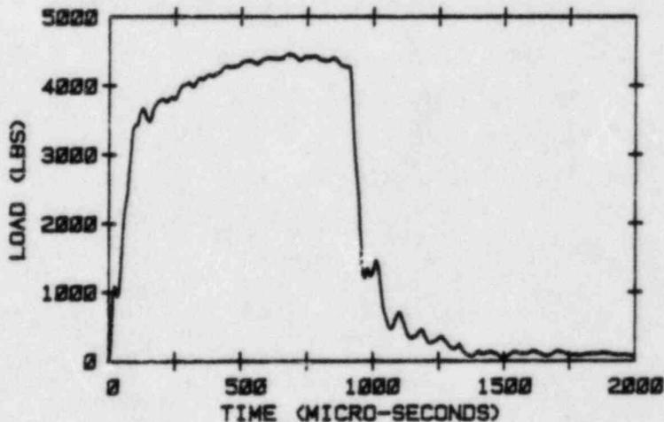
FIGURE A-6. INSTRUMENTED CHARPY IMPACT DATA FOR IRRADIATED HAZ METAL SPECIMENS FROM MONTICELLO 30 DEGREE SURVEILLANCE CAPSULE
