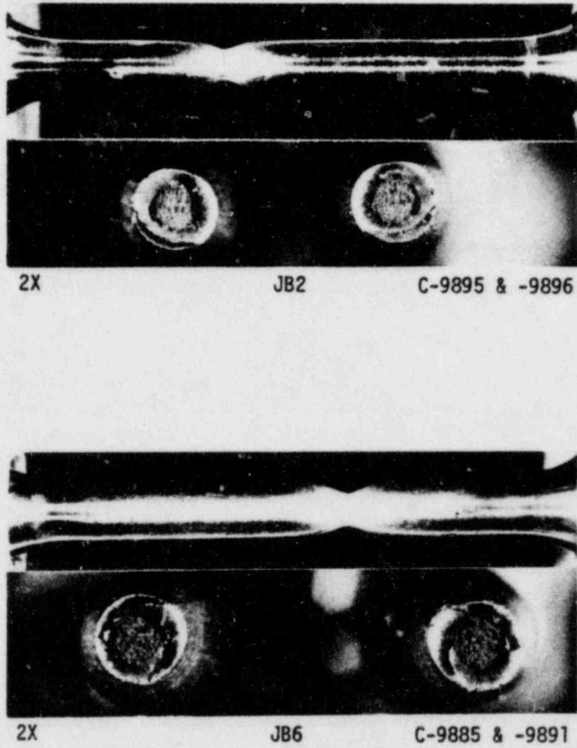
FIGURE 27. POSTTEST PHOTOGRAPHS OF THE IRRADIATED WELD METAL TENSILE SPECIMENS SHOWING BOTH THE REDUCED AREAS AND FRACTURE SURFACES (MONTICELLO 30 DEGREE SURVEILLANCE CAPSULE)
