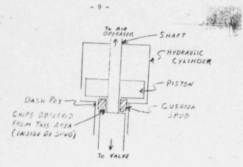
The cushion spud is "captured" between the piston and a larger shoulder of the shaft. In the above sketch the piston is shown with the valve in the closed position and the cushion spud in the dash pot. This cushion spud and dash pot decelerates the valve plug assembly just prior to seating.
